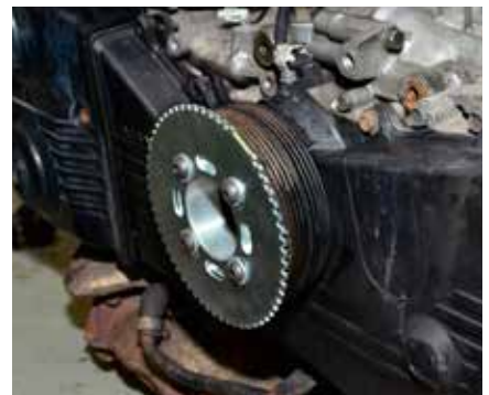
The top of the engine is cluttered by the a/c compressor and the power steering pump. The kit calls for these to be removed. Factory Five supplies a shorter belt. We also installed a trigger wheel that our aftermarket Electromotive ECU will use to measure crank position.
