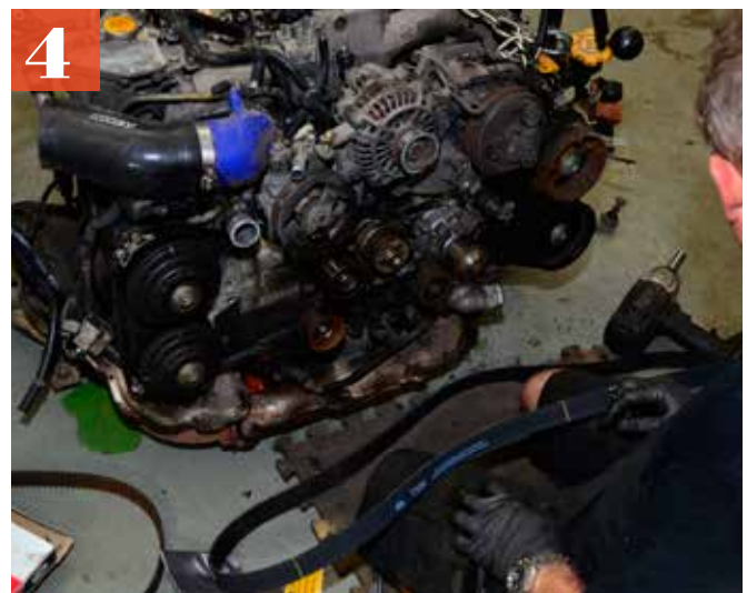
Subaru timing belts have yellow marks that line up with the timing marks on the cams.
