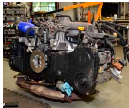
The top of the engine is cluttered by the a/c compressor and the power steering pump. The kit calls for these to be removed. Factory Five supplies a shorter belt. We also installed a trigger wheel that our aftermarket Electromotive ECU will use to measure crank position.
