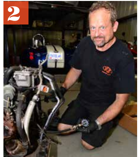
A simple compression test showed that our engine was healthy. Every cylinder had more than 150 psi of compression. Now we could prep it for the swap.
