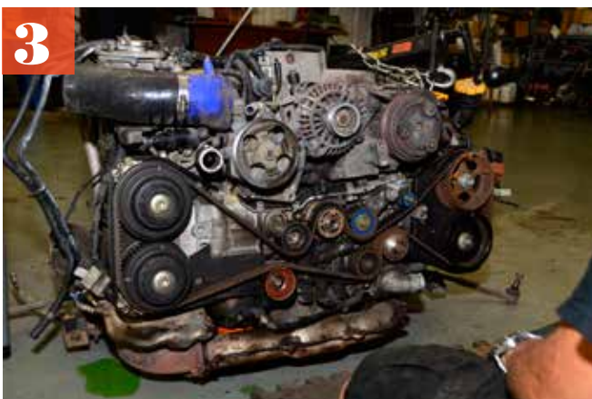
Subaru flat-fours have a convoluted timing belt arrangement, but not changing it can be an expensive mistake. Since access would be rather tough once the engine was installed in the 818, we decided to change it now.
