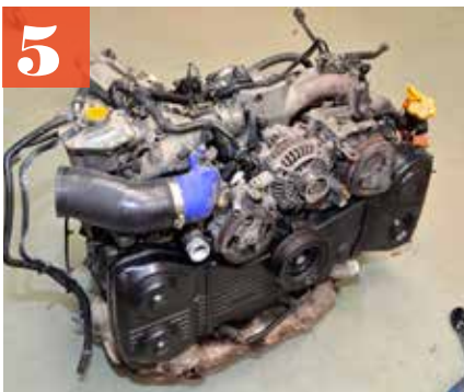
The top of the engine is cluttered by the a/c compressor and the power steering pump. The kit calls for these to be removed. Factory Five supplies a shorter belt. We also installed a trigger wheel that our aftermarket Electromotive ECU will use to measure crank position.
