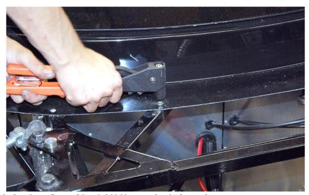
Rivet the front lower flange of the windshield surround to the frame tubes.
