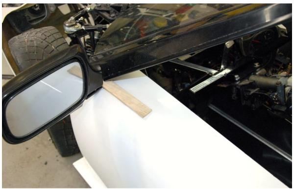
Keep about  $^{1}/_{8}$  inch (paint stick) between the windshield frame and door to prevent rubbing. Note, the side mirrors are not mounted yet.
