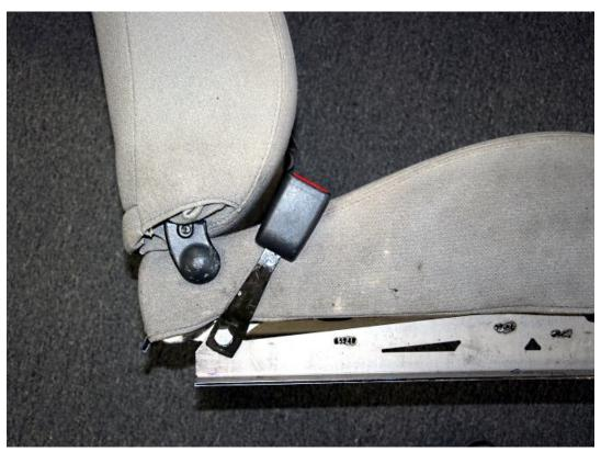
The bracket bolts to the seat using OEM hardware in the rear hole and slot of the bracket. Make sure to bolt the seat belt receiver to the seat using the rear bolt.
