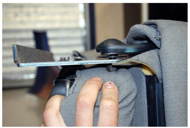
The rear also acts as a hinge so a bolt must be put through the hinge of the seat back into the bracket.
