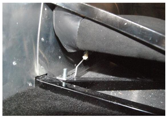
Place the bolt up through the bottom of the tube and seat bracket.
