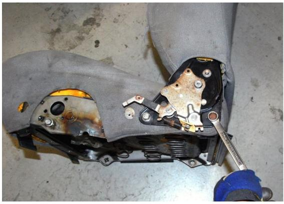
On the left seat left side, the rear bolt holding the seat hinge must be temporarily removed, because it also holds the seat bracket on.
