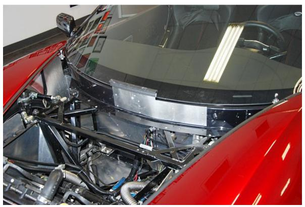
Rivet the rear hood support aluminum in-place.
