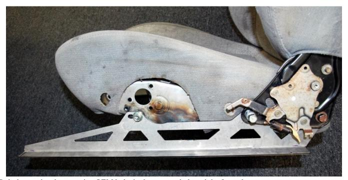
Bolt the seat bracket on using OEM bolts in the top rear hole and the front slot.
