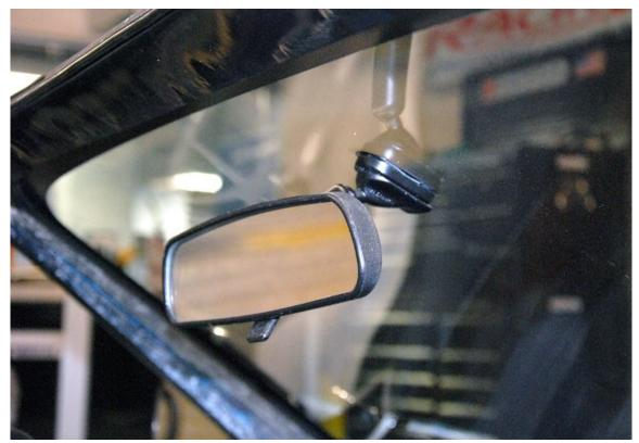
Some windshields have the rear view mirror mount already glued in place, if yours does not, have the glass guy attach it while he is there fitting the windshield. Once the glass adhesive is dry, install the OEM Subaru mirror onto the mount.
