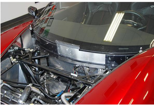
Cut the area out using the rear hood support aluminum as a maximum guide. The taller part of the aluminum should be centered on the windshield.
