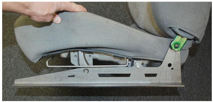
The right seat left side bracket bolts to the seat with two bolts in the front. Make sure to bolt the seat belt receiver to the seat using the rear bolt.
