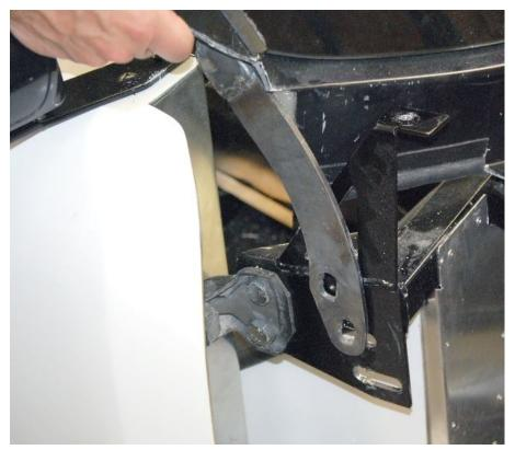
Fit the windshield surround on the car between the two fender/hood mount brackets that stick up from the frame.
