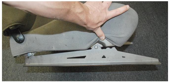
On the right side of the early model left seat, the forward hole must be cut in addition to the two long tabs. This cut can be seen above.
