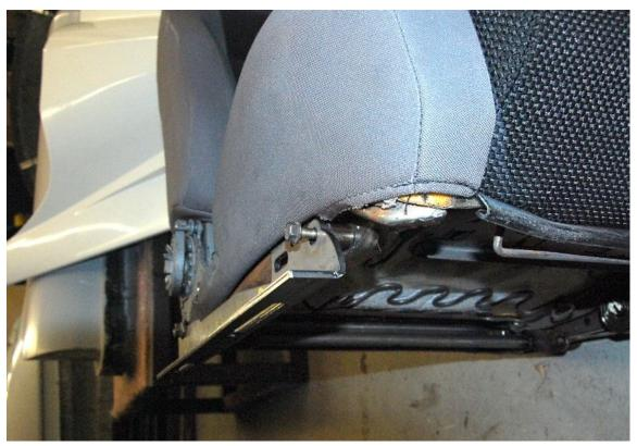
Use the provided spacer between the front hole of the bracket and seat in order for the bracket to sit flat.
