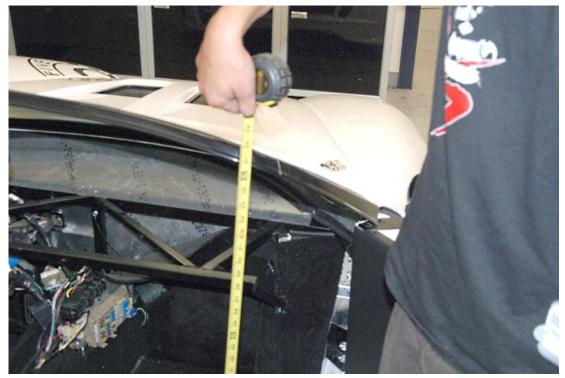
Measure both corners from the floor to make sure the fame is even then tighten the mounting hardware.
