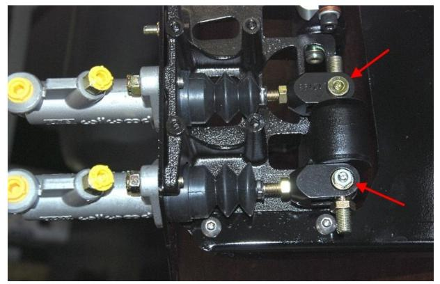
The brake pedal master cylinder pushrod mounts are different from each other. Only one has a screw and nut. This is normal.
