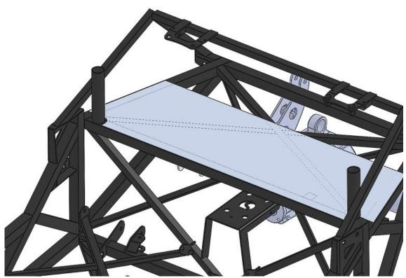
Install the front aluminum floor that goes under the front of the fuel tank.
