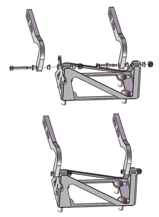
Attach the hinge arms to the hinge arm standoffs as shown. The hinge arms go on top of the mounts with the bronze bushings pushed into both sides of the arm and both sides of the hinge arm standoffs.
