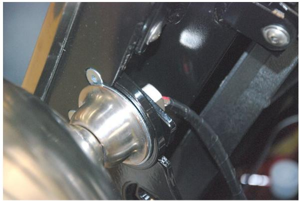
Headlights are bolted through the side covers. If you plan to take your side covers on and off and not have to thread each wire through the nut and have to realign the headlight each time a good idea is to make a spacer to go on the radiator mount and cut the side covers to go around the spacer so headlight removal is not necessary.
