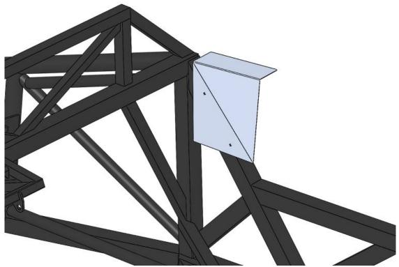
With the door hinge and latch adjusted, position the striker cover.
