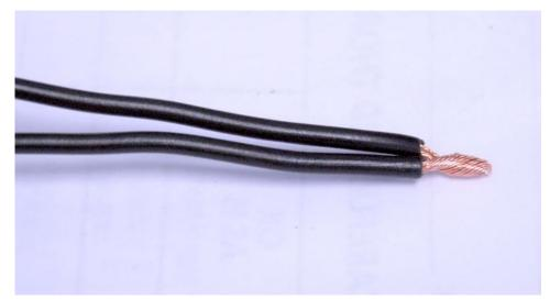
Use an extra piece of wire and twist it together with the fan ground wire on the front harness.
