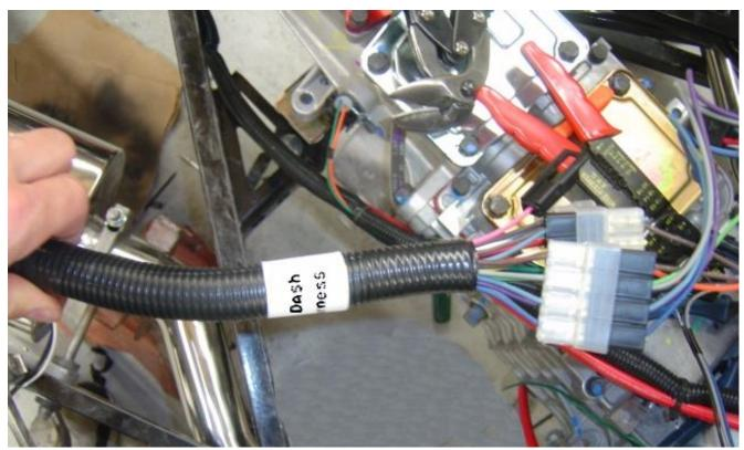
Locate the dash harness section of the chassis harness.
