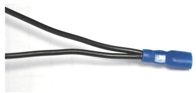
Attach the female terminal connector to the ground wires and connect it to the fan ground.
