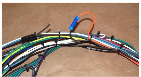
In the dash harness the fan switch lead can now be spliced into the gauge positive feed circuit (12 volts switched positive) so the fan will run only with the ignition on.
