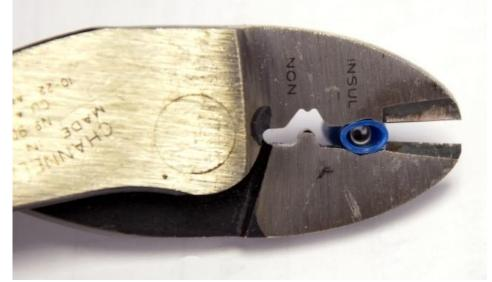
Squeeze the wire end of a <sup>1</sup>/<sub>4</sub>" female spade terminal so that it is slightly oval.
