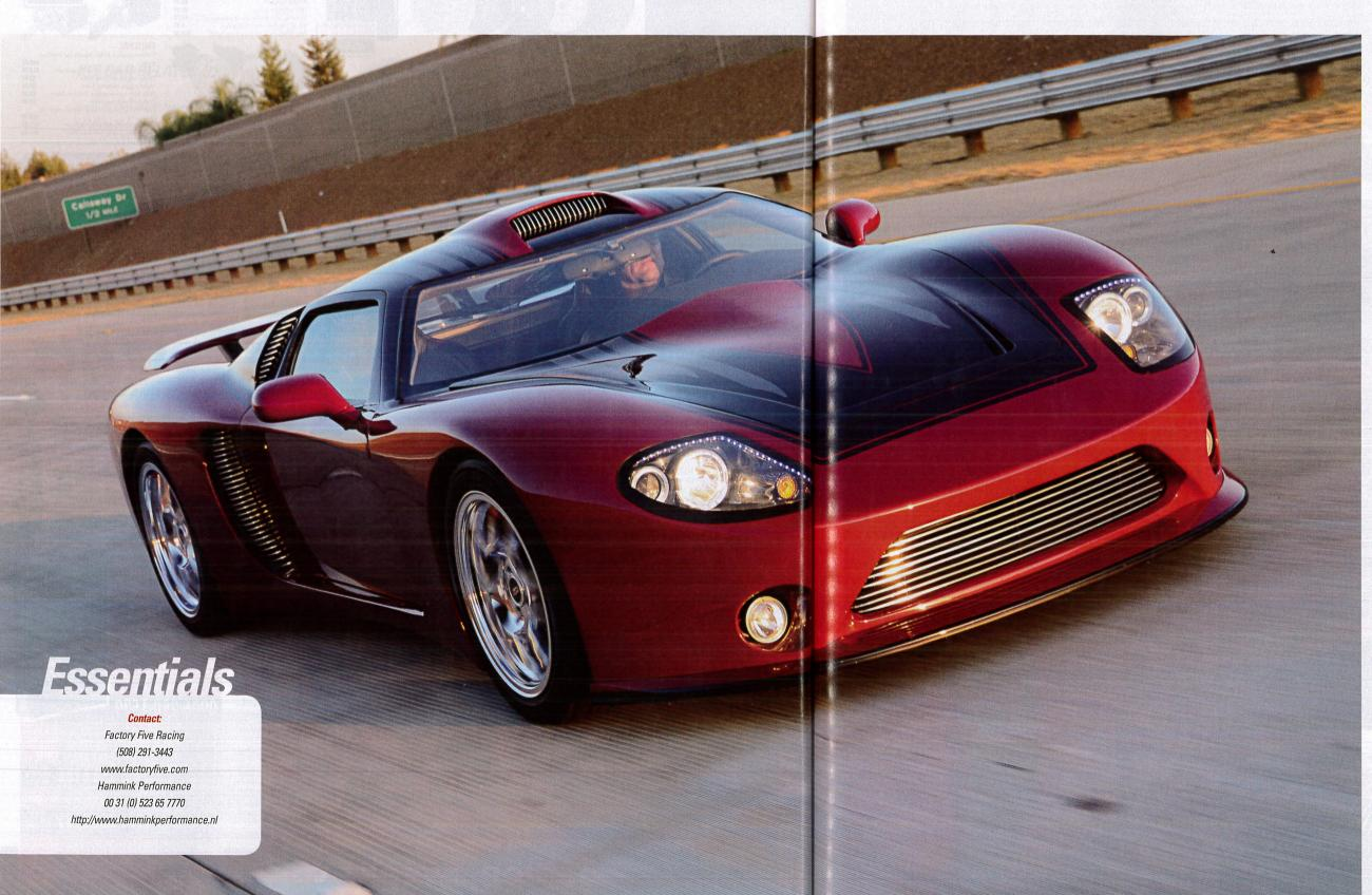
actory Five's GTM supercar is based on the running gear from a 1997-2004 Chevrolet C5 Corvette along with a Porsche G50 transaxle. It's a stunning looking car that can thankfully be constructed in kit form and is available in the UK via European distributor Hammink Performance of the Netherlands.
