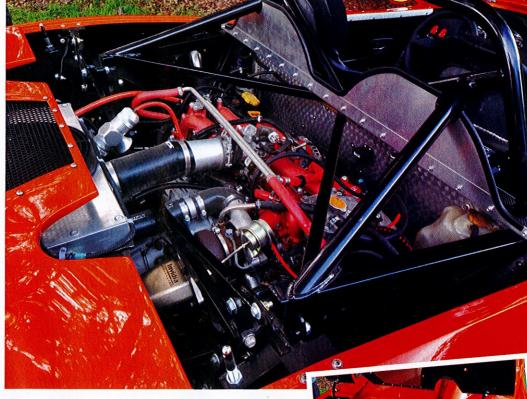
Tom's car was tuned on the dyno to ensure that everything was working properly. Since the transmission works best with horsepower numbers below 300, they actually detuned the motor slightly to ensure it could handle the new power, ending up with 250 rear-wheel horsepower and 240lb ft torque, produced at a conservative 14lb of boost. The finished car weighs slightly more than the published specs because of the extras involved, registering 934kg, but Tom doesn't plan on a name change!
