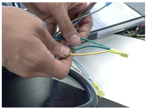
In the dash harness, cut the yellow and white rear turn signal light wires off the turn signal connectors that are for the dash turn signal switch so that the turn signal lights do not back feed and light the front turn signals when the brakes are pressed.
