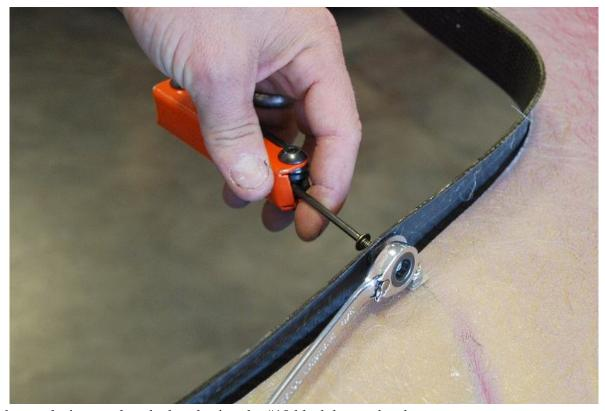
Attach the cowl trim panel to the hood using the #10 black button head screws.
