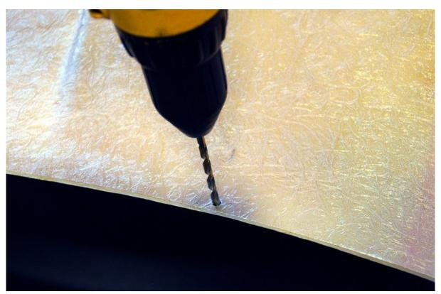
Use a  $\sqrt[3]{_{16}}$  drill bit to drill the locations marked.
