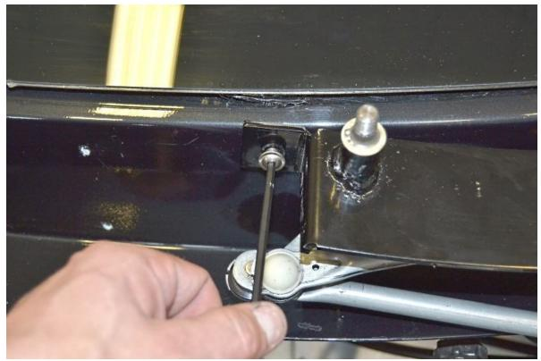
Attach the motor assembly using the  $\frac{1}{4}$ "x  $\frac{3}{4}$ " button head screws using a  $\frac{5}{32}$ " Hex key.
