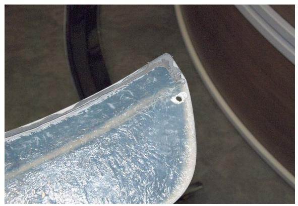
Drill the cowl at the marked locations using a ¼" drill bit.
