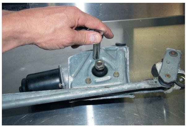
Remove the three bolts holding the wiper motor onto the mount bracket using a 10mm socket.
