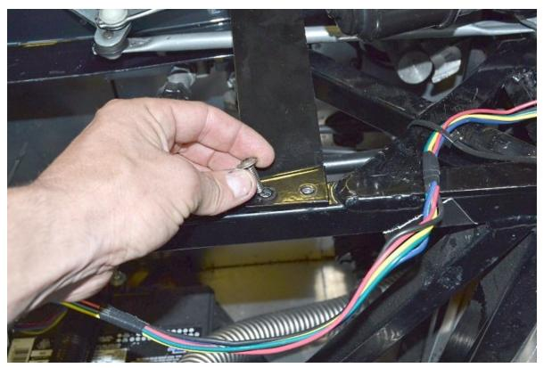
Reattach the front mount to the frame then double check clearance of the motor arm to control arm bolt and check all three linkage arms and wiper shaft arms for clearance by rotating the motor arm a full revolution by hand or with a wrench.
