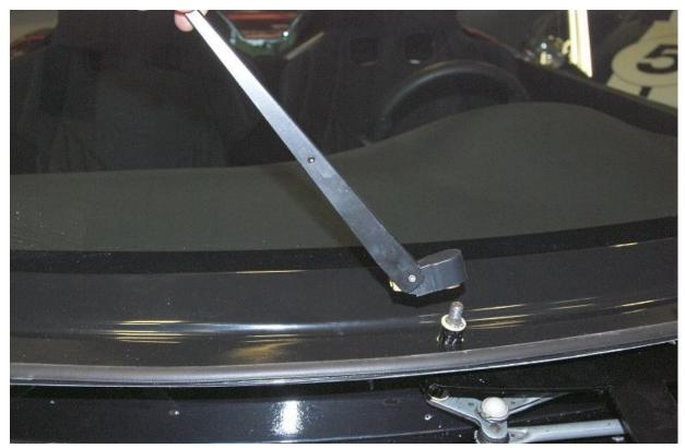
Put the wiper arms on the wiper shafts.
