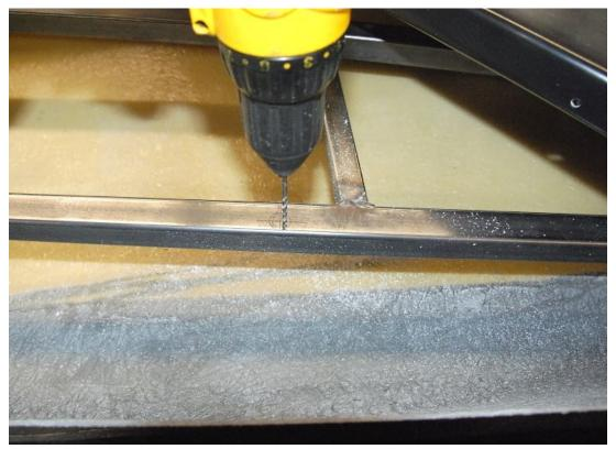
Drill a <sup>25</sup>/<sub>64</sub> inch hole and install a rivnut at the point marked.
