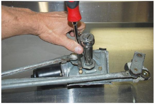
Remove the wiper motor arm using a 17mm socket and large flat head screwdriver between the arm and the head of a motor mount screw to stop it from turning.
