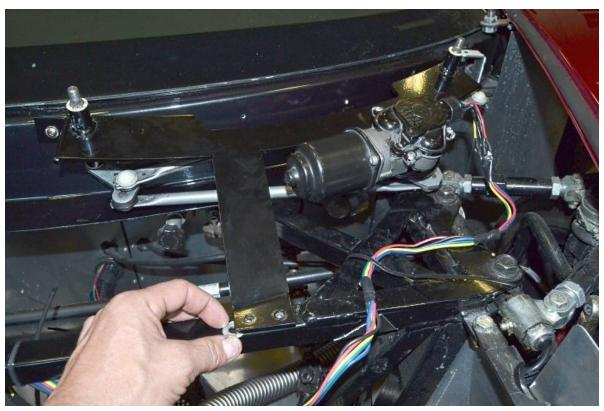
If necessary for clearance space the front mount up using the 1/4" washers under the front bracket mount.
