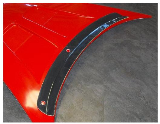
Remove the hood and place the cowl panel on top of the hood lining it up with the marks made and so that the back edge of the cowl is flush with the back edge of the hood.
