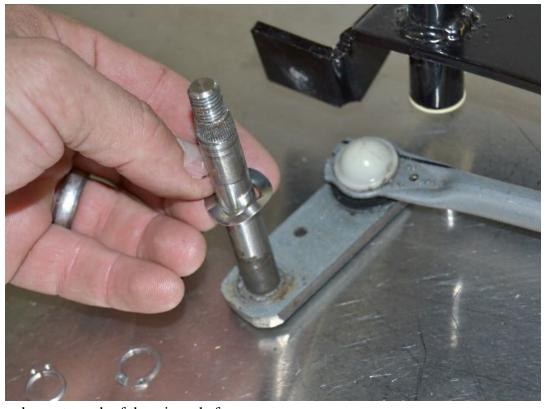
Put a wave washer onto each of the wiper shafts.
