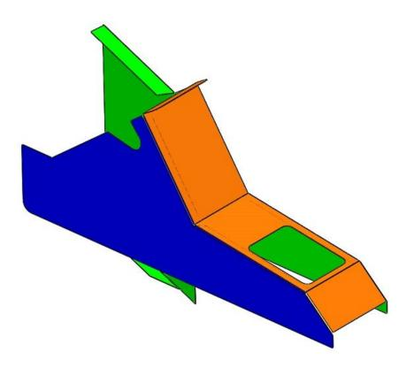
Mark the top of the center console along the edges for rivets.
