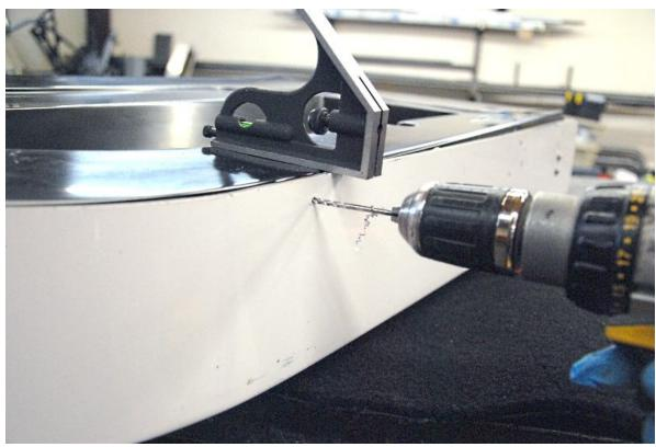
Set the door liner height so that it is flush with outer shell then drill  $^{1}/_{8}$  inch holes through the outer shell and the liner for #8 black oval head screws and countersunk washers around the bottom and back of the door. Pull the liner out then drill oversized  $^{3}/_{16}$  inch holes in outer shell so the screws pass through outer shell easily.
