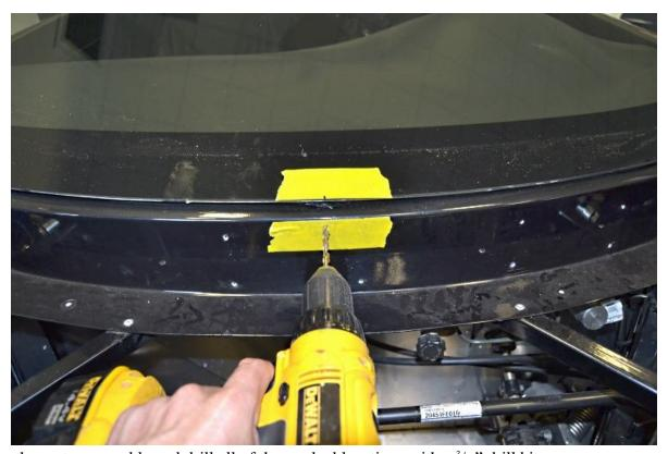
Remove the motor assembly and drill all of the marked locations with a  $\frac{3}{16}$ " drill bit.
