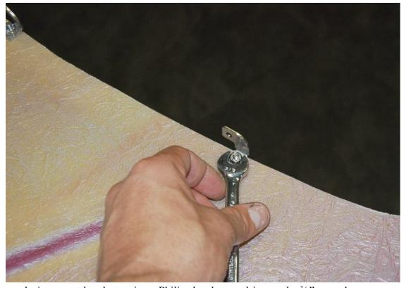
Attach the cowl trim mount brackets using a Philips head screwdriver and a 3/8" wrench.
