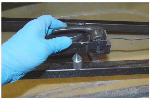
Install the door handle and bend/cut the linkage to the correct length so the latch will actuate.
