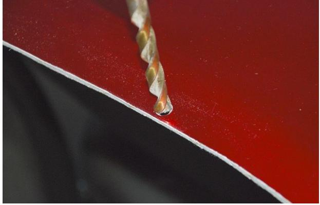
On the top side of the hood, use a  $\frac{3}{8}$ " drill bit or a counter sink bit to countersink the hole for the flat head screws.
