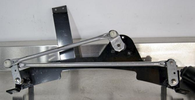
Insert the wiper shafts through the bushings in the bracket so that the linkage arms are as shown.
