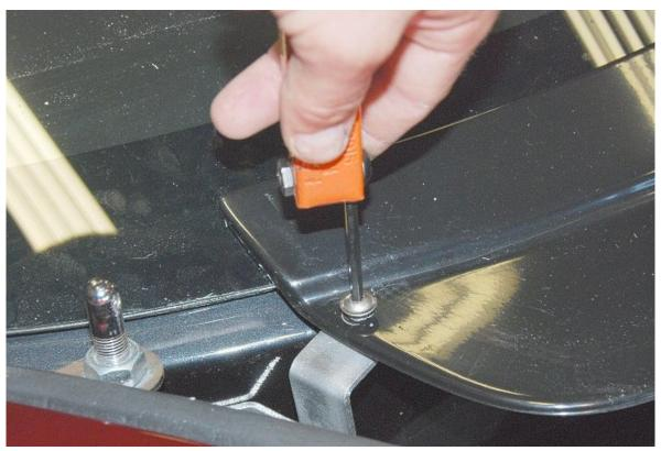
Attach the cowl panel to the side brackets using the  $\frac{1}{4}$ "x  $\frac{3}{4}$ " button head screws and a  $\frac{5}{32}$ " Hex key.
