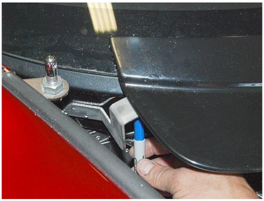
Locate the cowl panel so it sits down on the windshield then hold the side cowl mount brackets up to the windshield surround and the underside of the cowl panel and mark the holes on the cowl and the windshield surround.
