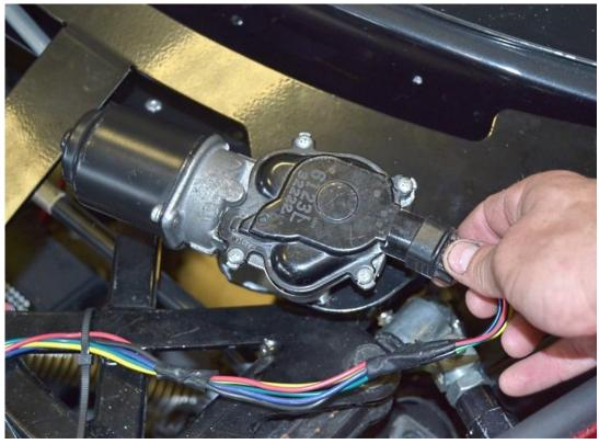
Attach the wiper motor connector to the wiper motor. If necessary extend the wires using the included wire and red butt connectors or solder the wires.
