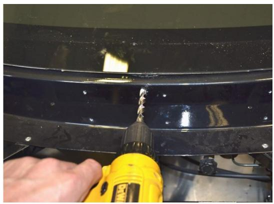
Open the hole up for a rivnut using a <sup>25</sup>/<sub>64</sub>" drill bit.
