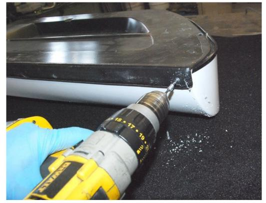
Drill 1/8" mounting screw holes along the top flange.
