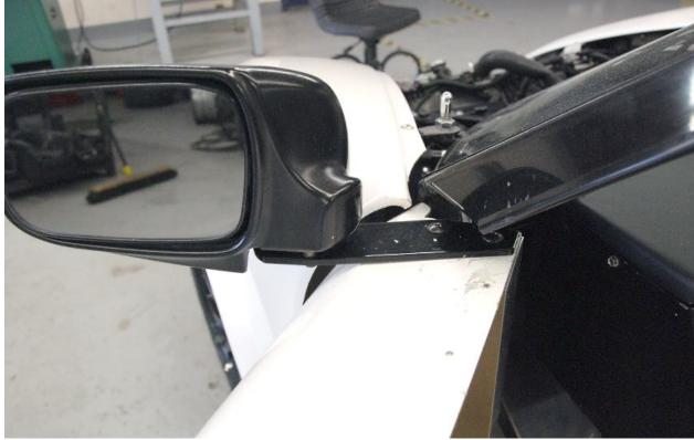
Mount the side view mirror bracket to the door using the two top existing black ¼" x 1" mounting screws that hold the door frame to the door.
