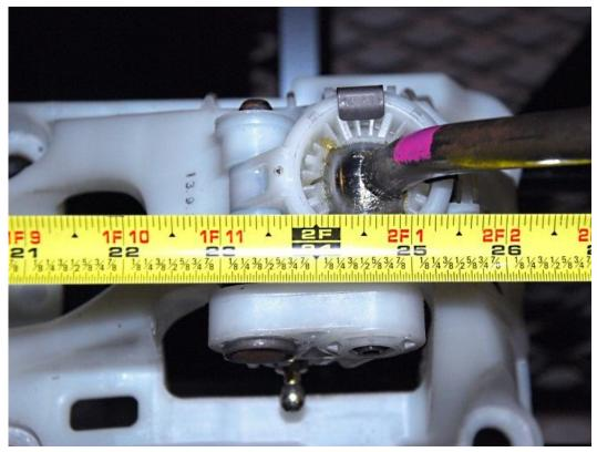
Put the shifter handle on the center tunnel and measure from the front cockpit wall center 1" tube to the center of the shifter pivot ball 24.50 inches.
