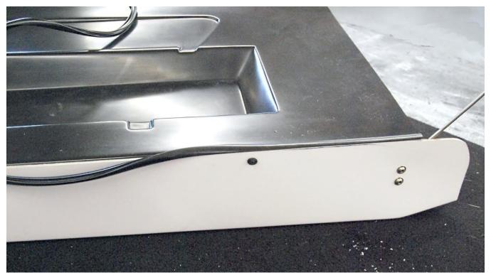
Back off the screws along the bottom of the liner and install "T" weather stripping along the bottom and back edge of door skin to door liner seam. We suggest applying silicone to the seam beforehand.
