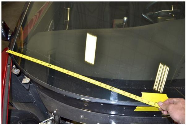
Use a tape measure and marker to find the bottom center of the windshield ( $\sim 31^{5}/_{16}$ ") and mark the masking tape.
