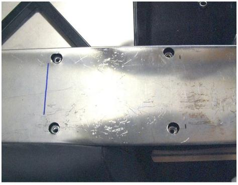
Install rivnuts in the top of the tunnel tubes for mounting the shifter.
