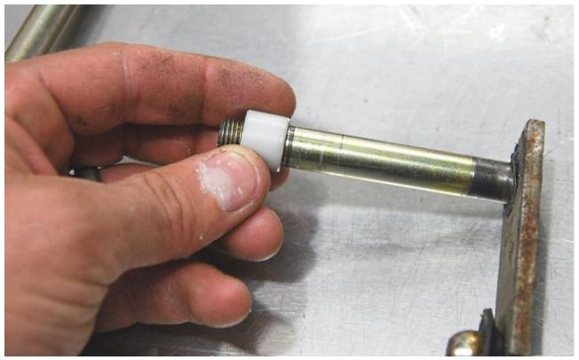
Remove the white bushing from the wiper arm shaft.
