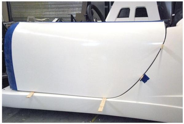
Close the door, lining up all body lines. Space the door <sup>3</sup>/<sub>16</sub> inch (paint stick thickness) from the body.
