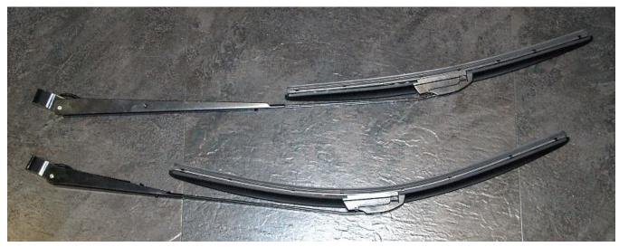
Attach the wiper arms to the wiper blades. The left side gets the short arm and long blade and the right side gets the long arm and short blade.
