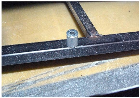
Use spacers to set the door handle to the desired height, flush with door liner.
