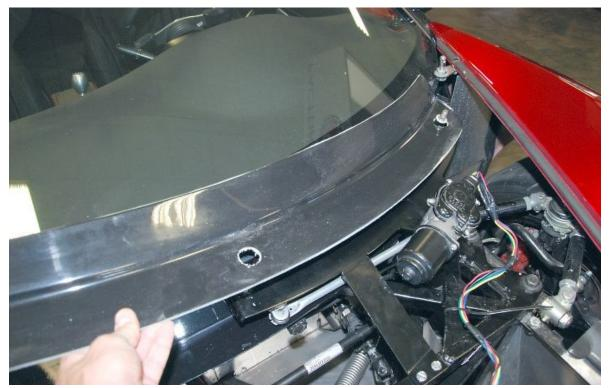
Put the cowl panel on over the wiper shafts.
