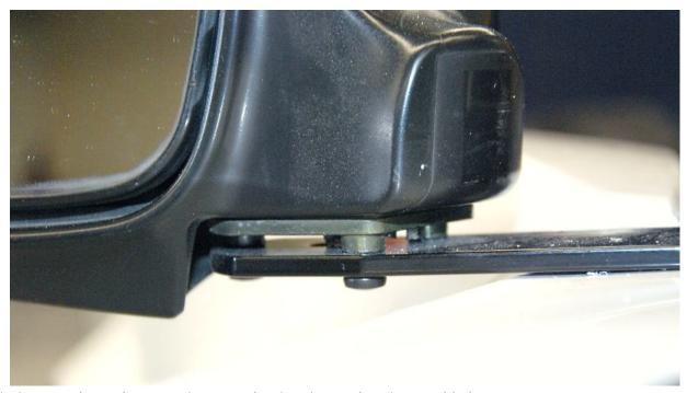
Attach the rear view mirrors to the mounting brackets using the provided screws.
