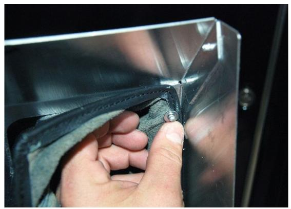
From the top side, use a  $\frac{3}{16}$ " rivet in the aluminum hole drilled with a #10 washer under the boot. Push the washer against the boot while tightening the rivet so that the boot is squeezed against the aluminum.
