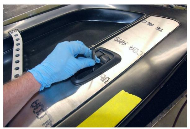
Place the door handle bezel in the aluminum and snap the opener to it, sandwiching the aluminum. Place the assembly on liner and mark mounting hole on door frame.
