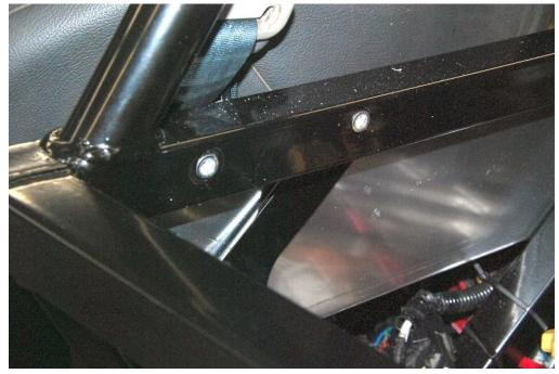
Install rivnuts at the mounting points marked.
