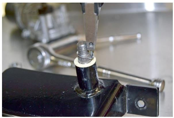
Attach the snap ring to the wiper shaft groove while pushing down on the bracket compressing the wave washer.
