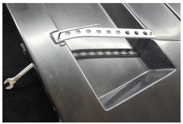
Install one M6 x 20mm button head nut and bolt.
