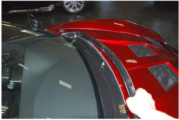
Check the fitment of the cowl trim panel with the hood on the car as well checking to see that the panel will touch the cowl panel.
