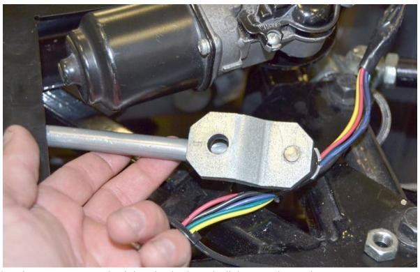
Rotate the wiper motor arm so that it is going back on the linkage as shown above.
