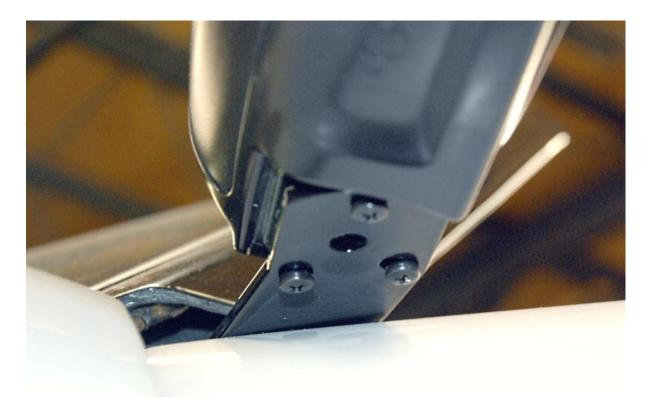
Fit the mirrors to the doors making sure to check the clearance on the windshield surround.
