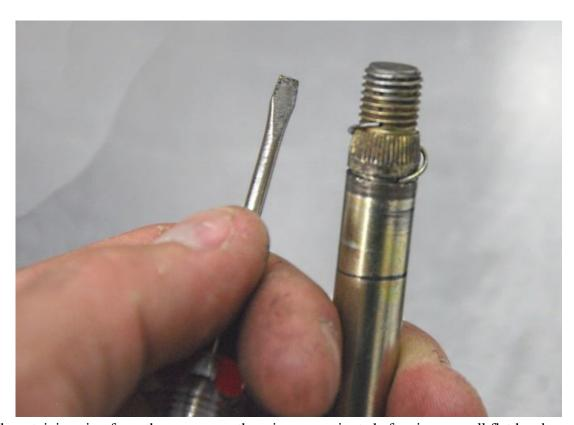
Remove the retaining ring from the groove on the wiper arm pivot shaft using a small flat head screwdriver.
