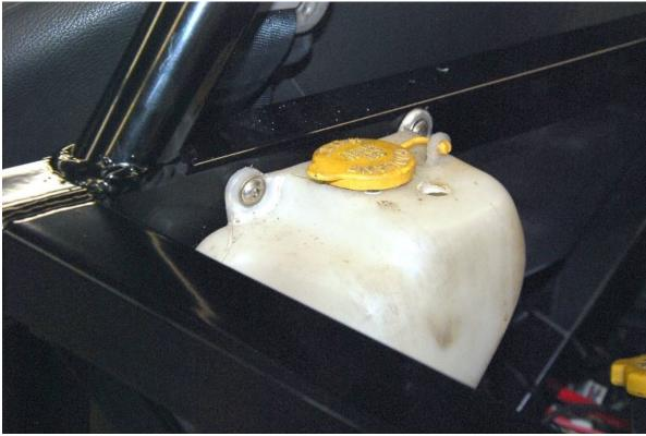
Attach the overflow to the frame.
