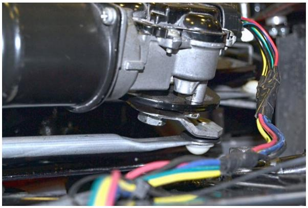
Attach the motor arm to the motor using the stock nut and 17mm wrench.
