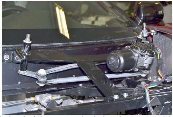
Move the wiper shafts and linkage arms so they are located as shown and the motor arm can reach the motor.
