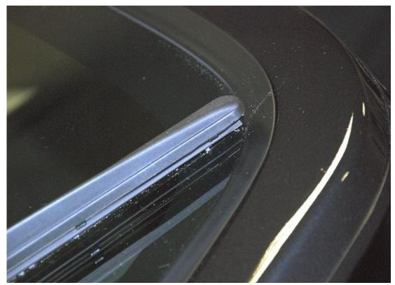
Check clearance between the left arm and the corner of the windshield. If necessary, rotate the arm down slightly.
