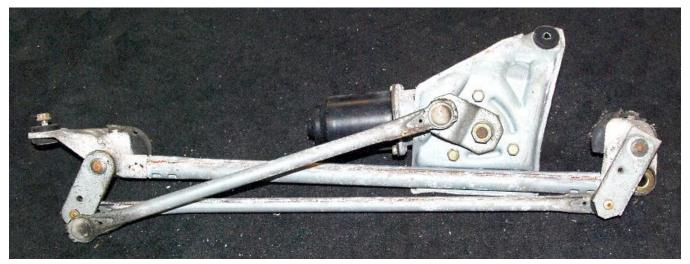
Wiper motor, shaft and wheelbox assembly.
