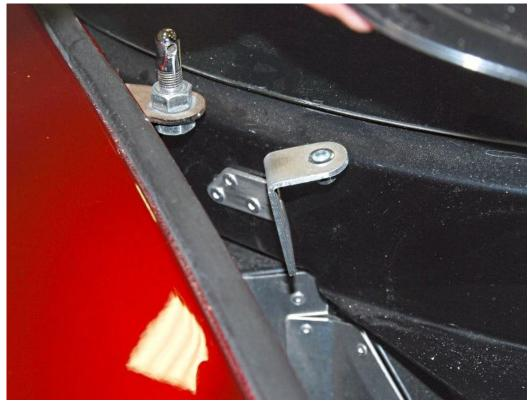
Install rivnuts on the side cowl mounts and rivet the side cowl mounts to the windshield surround using the  $^{3}/_{16}$ " rivets.
