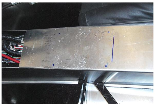
Remove the shifter and drill the four marked holes for rivnuts. Drill slightly larger holes through the alum so the tunnel can be removed.
