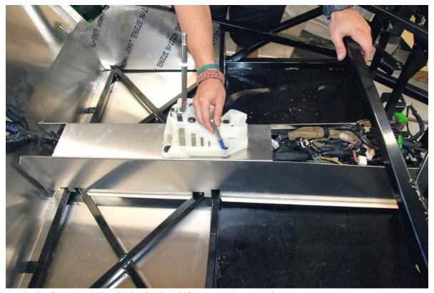
Mark through the four mounting holes in the shifter onto the tunnel.
