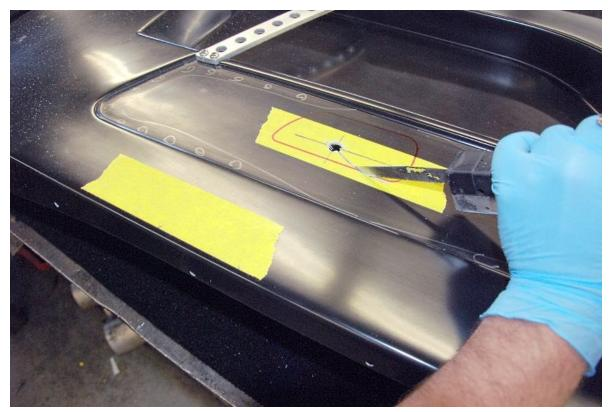
Use a saw to cut to the outside of the marker on the door liner.
