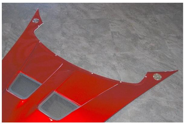
Using a conservative line, cut the hood so that the cowl trim panel will sit correctly on the hood.
