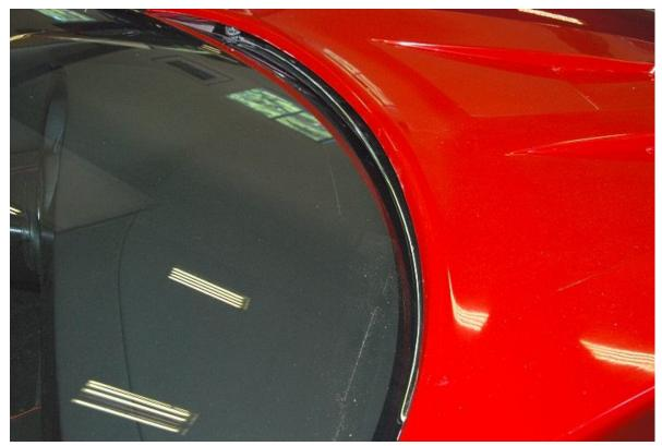
Note that the cowl panel is flush with the rear edge of the hood.
