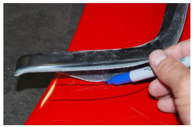
Center the trim panel between the cowl lines made and move the trim panel forward and so the top curved area is above the curve on the hood so they will sit on top of each other once the hood it cut.
