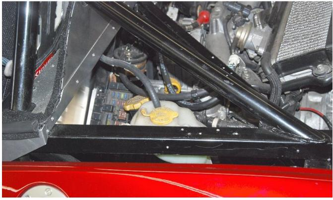
Hold the coolant overflow up to the 1.50 inch tube to the left side of the engine and mark the center of the mounting holes. Make sure you have enough room to fit a drill in to drill the holes.
