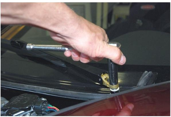
Use a 17mm wrench or socket to snug the wiper arms up so they will just move with the motor. Do not fully tighten the nuts.
