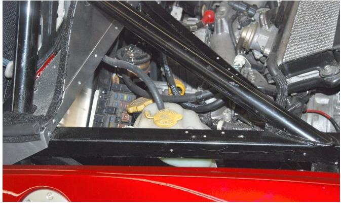
Insert the overflow tubing into the tank and run it over to the engine attachment location.
