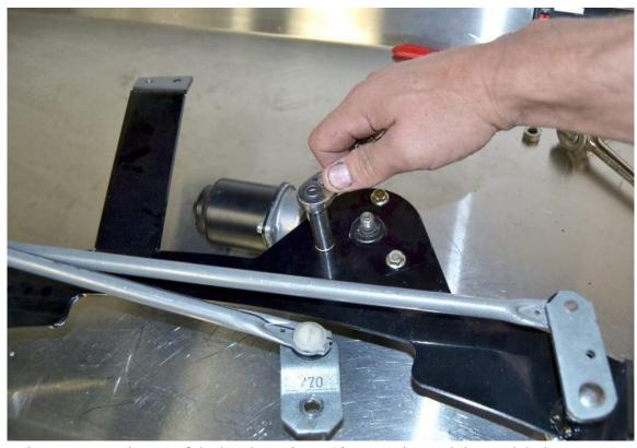
Attach the wiper motor to the top of the bracket using a 10mm socket and the stock bolts.
