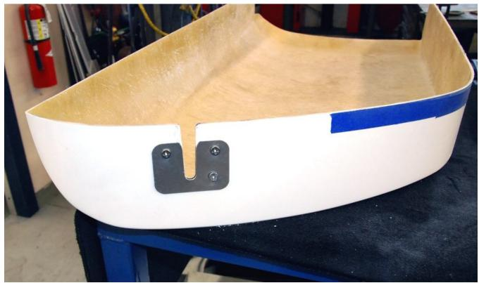
Place the latch trim piece around the cutout, and then drill the three mounting holes out of the door skin.
