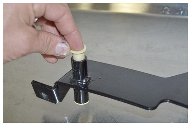
Push the nylon bushings into the shaft sleeves.
