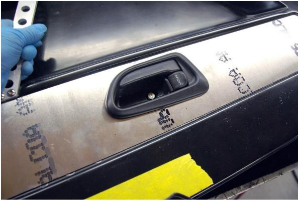
Re-install the door liner with the door handle bezel to check for fitment attaching them with the  $\frac{1}{4}$  inch x 2.00 inch round Philips head screws.
