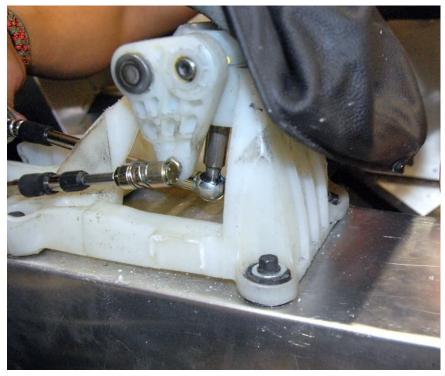
Tighten the shifter down to the transmission tunnel using ½" x 1.50" hex head bolts.
