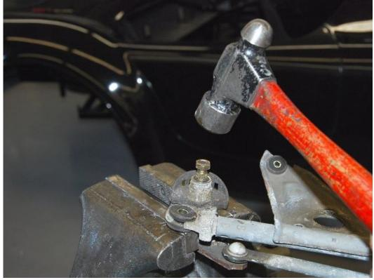
Remove the wiper arm shafts from the mount bracket. With the nut still on the splined shaft end, hit the nut with a hammer to remove the washer then remove the nut.
