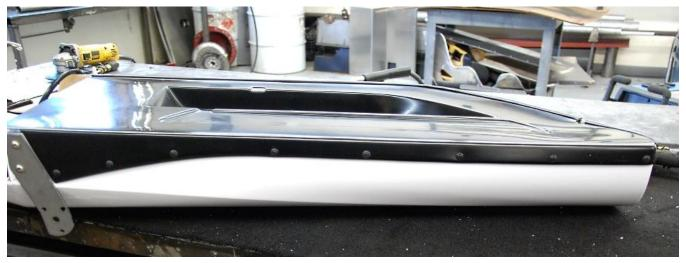
If desired install oval head screws and countersunk washers all along the top flange. If not, Put one at each end of the top flange.
