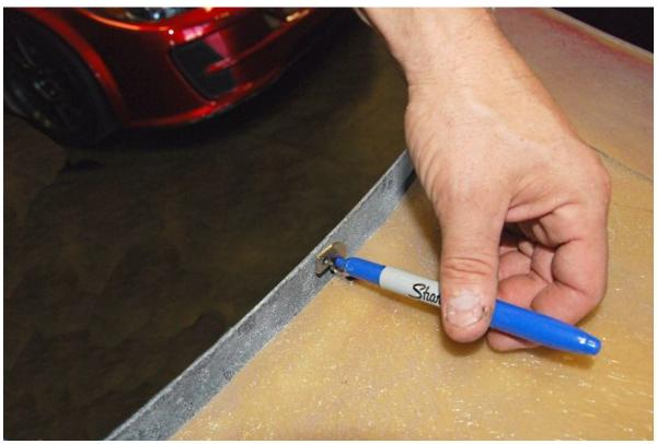
Hold the cowl trim panel up to the hood and mark the location of the mounting holes on the back side of the cowl trim bracket.
