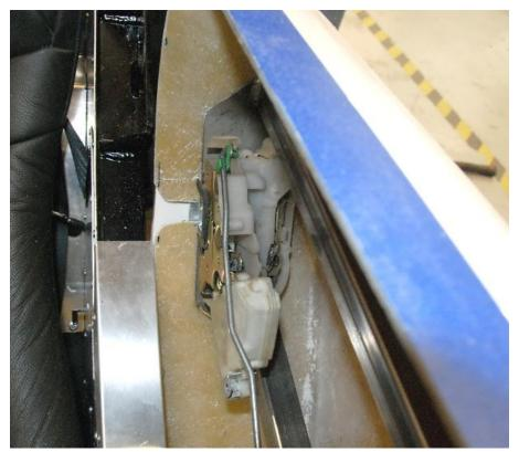
Test fit the door, latch and striker together. Make sure the cutout is deep enough for the door to fit correctly.
