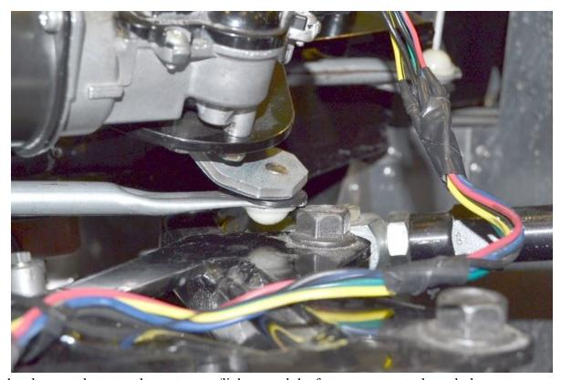
Check the clearance between the motor arm/linkage and the front upper control arm bolt.
