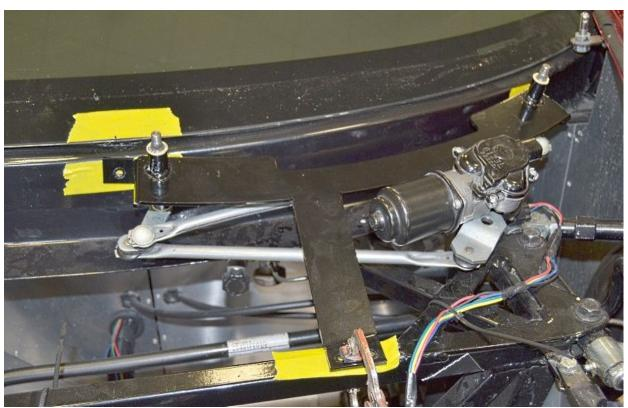
Clamp the motor bracket assembly to the 1" tube that goes across the car. The front of the bracket should be even with the front side of the tube and the rear mounting hole near the center of the car should be aligned with the center mark made. The top of the rear mounting hole tabs should be aligned with the angled edge of the windshield.
