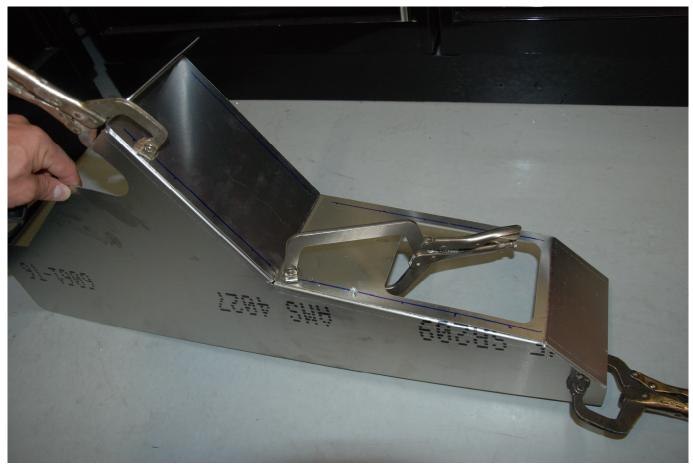
Clamp and screw the aluminum panels together using the self-taping screws.
