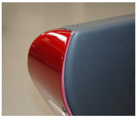
Either the liner or the door skin will need to get sliced so that the door liner can make the transition from the outside of the panel to the inside.
