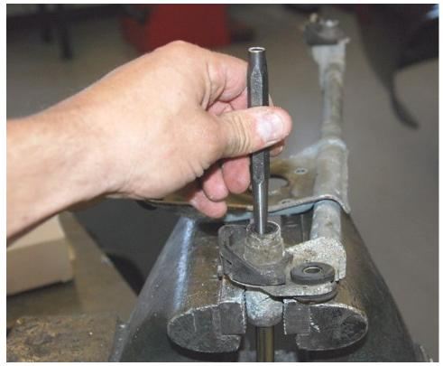
If necessary, use a punch or similar to get the wiper arm shaft completely out.
