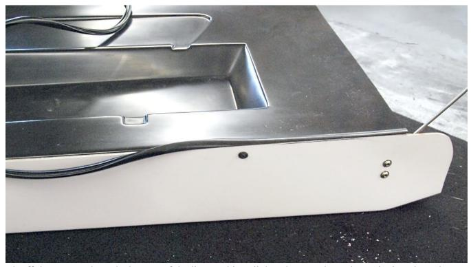
Back off the screws along the bottom of the liner and install the edge guard weather stripping along the bottom and back edge of door skin to door liner seam.
