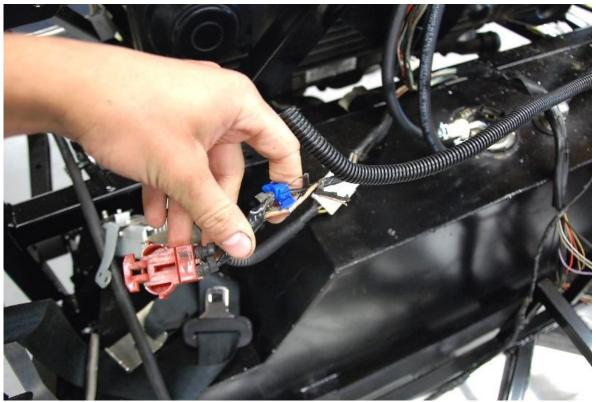
Splice the provided fuel pump plug into the harness in place of the Subaru plug. If you did not mark it on disassembly you can use the top of the sending unit plate to locate the correct plug and wire locations.
