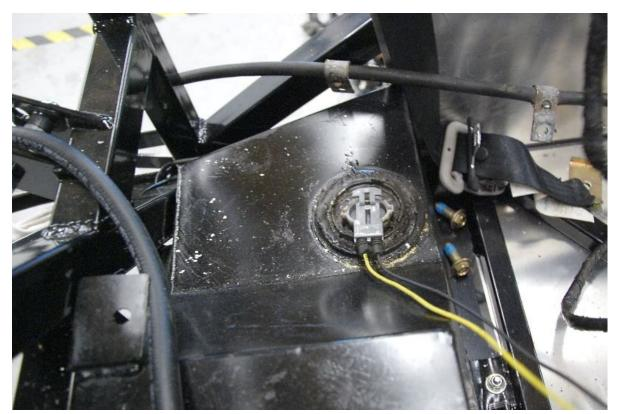
Splice the fuel level sender into the factory harness in place of the old Subaru unit.
