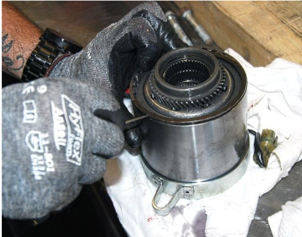
Remove the c-clip that holds the differential together.
