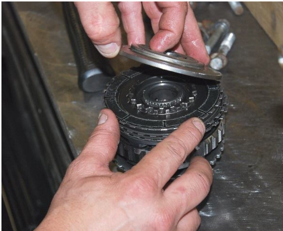
Separate the differential and all the clutches until just the center section is free.
