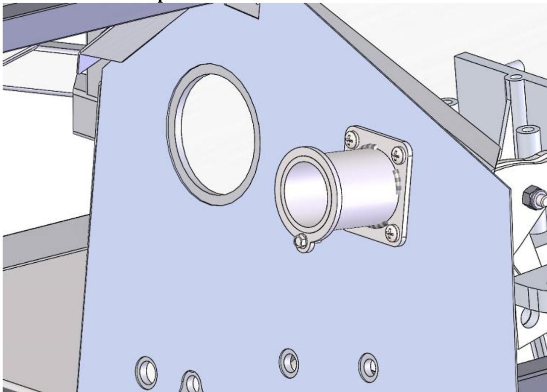
Push the firewall spacer into the front of the footbox and attach to the front of the pedal box using the screws provided and a Philips head screwdriver and  $\frac{3}{8}$ " wrench.
