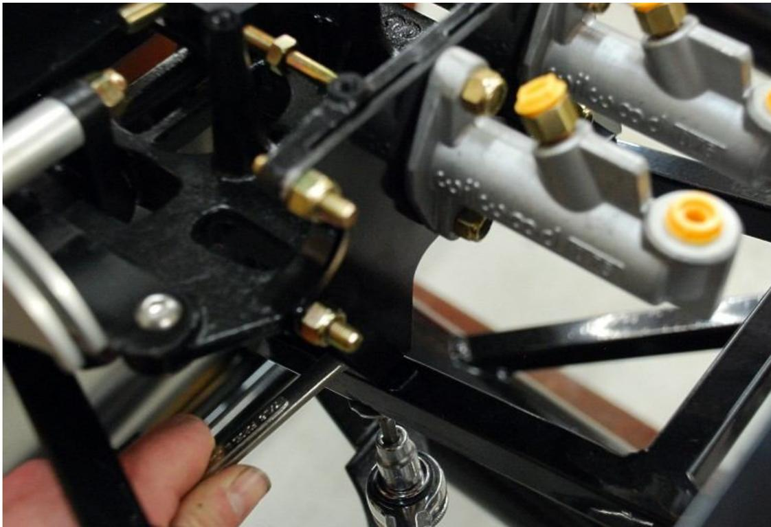
Tighten all the remaining hardware mounting the pedal box to the chassis.
