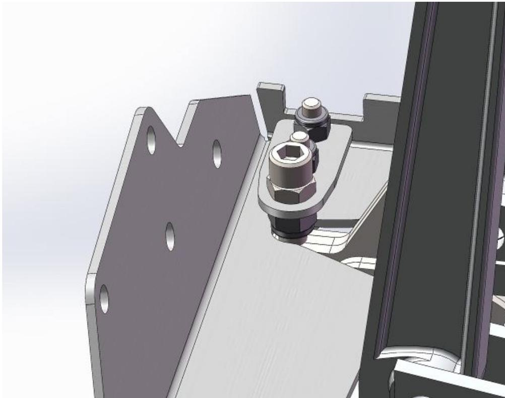
From the underside, push the screw through the quadrant pedal stop mount plate and hand tighten the locknut on the screw.
