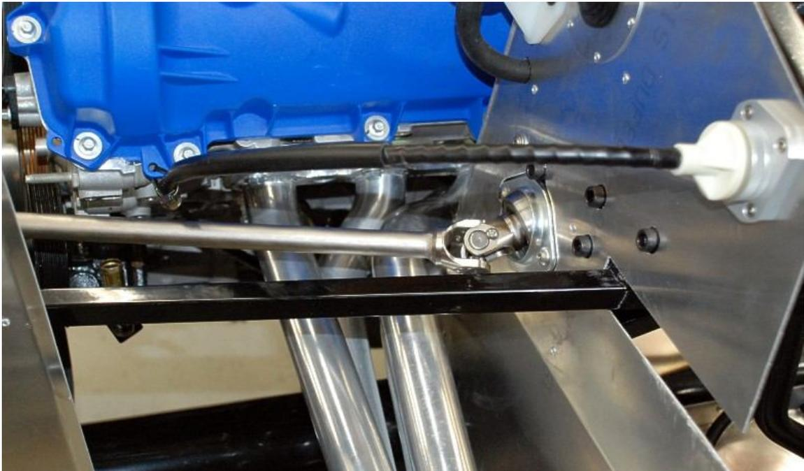
Route the clutch cable down to the bellhousing. Using zip ties or insulated clips tie the cable safely away from the headers and the moving steering components. It can be fastened to the engine using the bracket on the cable to the front lower bolt that holds the starter cable just before it leaves the block or, to the lower engine bay ¾" tubing.
