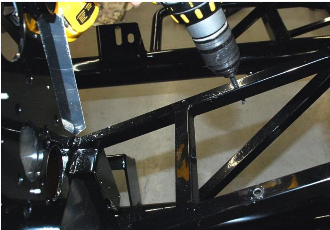
Loosen the bolts and remove the pedal box assembly from the footbox then use a 1/4" drill bit and drill to drill through the 3/4" tubes at the locations marked for the rear mount.
