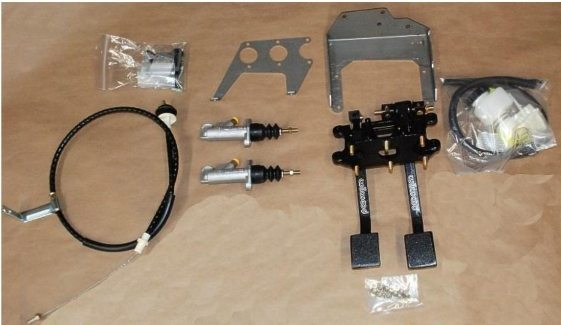
Unpack the pedal box assembly. Now is a good time to paint all of the bare steel brackets.
