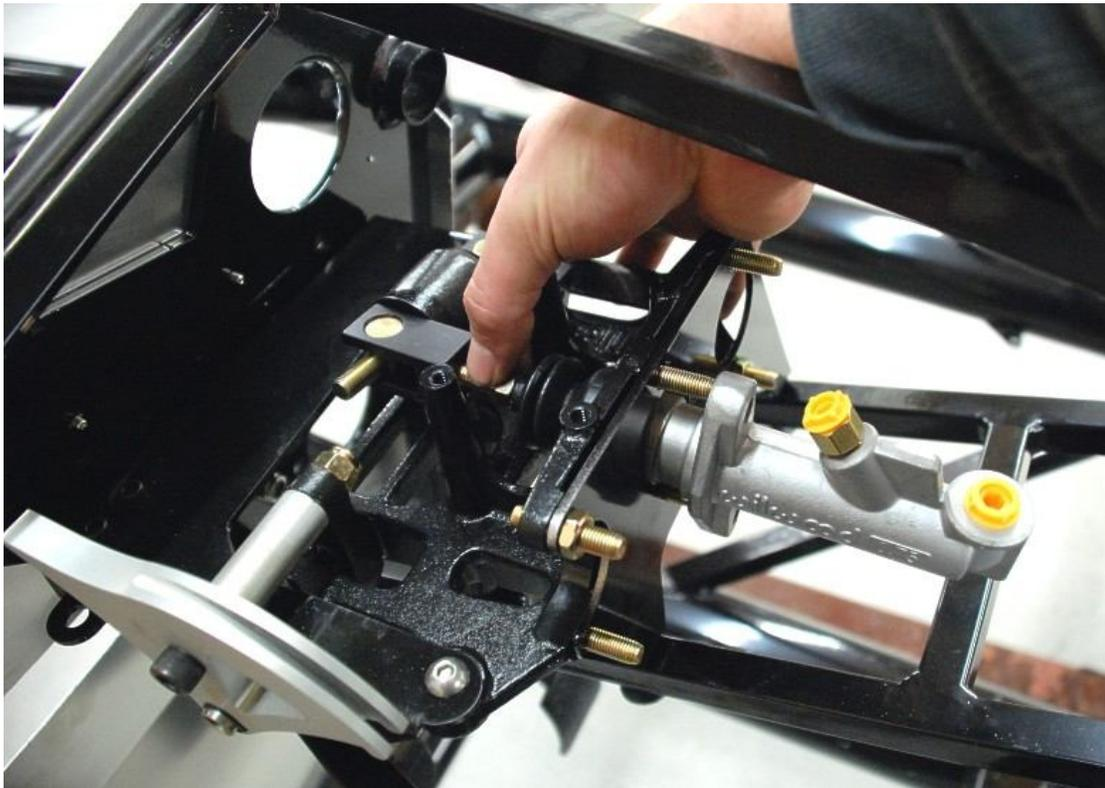
Put one of the master cylinders onto one of the brake master cylinder mounts and turn the threaded shaft into the threaded mount on the brake pedal. As a starting point, thread the shaft in until you can see it is flush on the other side of the mount.
