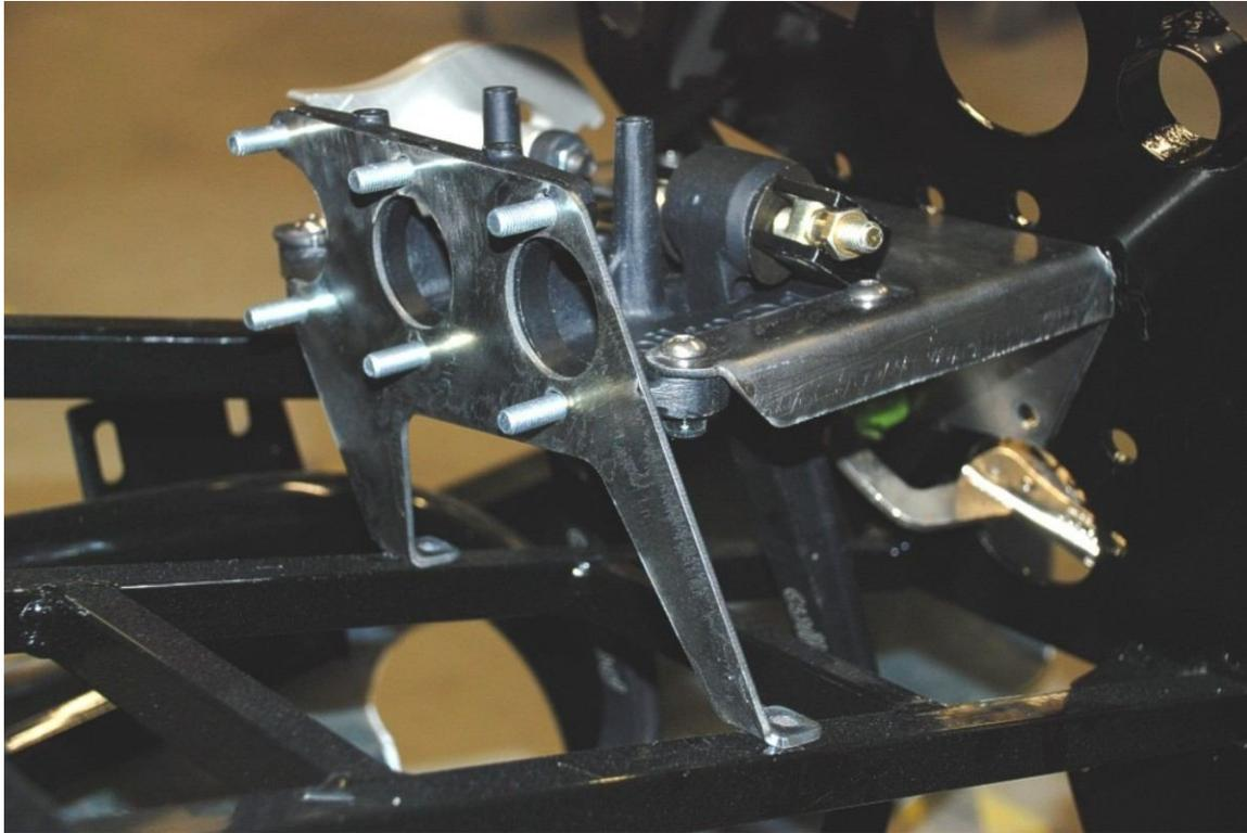
Push the rear pedal box mount onto the master cylinder mount studs and use a few of the jam nuts from the Wilwood pedal assembly to temporarily hold the rear mount in place.
