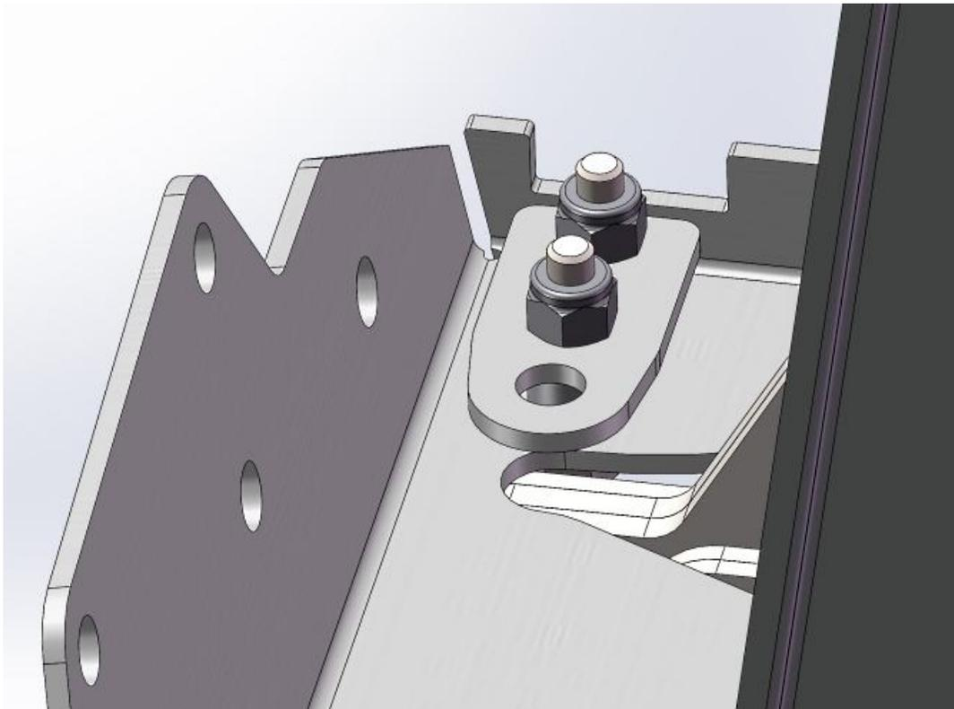
Attach the Clutch pedal stop mount to the bottom of the pedal box using two 1/4" socket head screws, spacers and locknuts.
