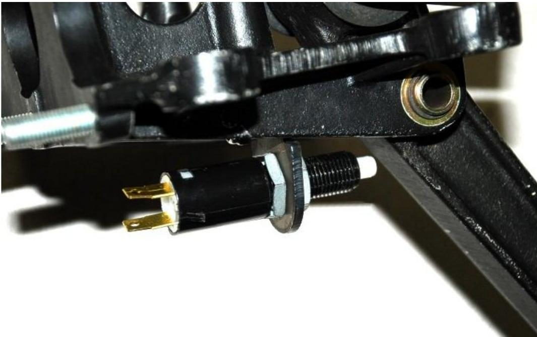
Attach the brake switch mount to the pedal box using the black #10 screw and locknut.
