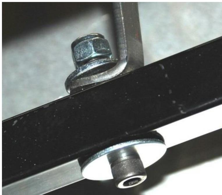
Reinstall the pedal box assembly in the driver's footbox; use the 1/4" x 1.50" screws from the pedal box fastener assembly with a fender washer next to the head. Leave all the hardware hand tight.
