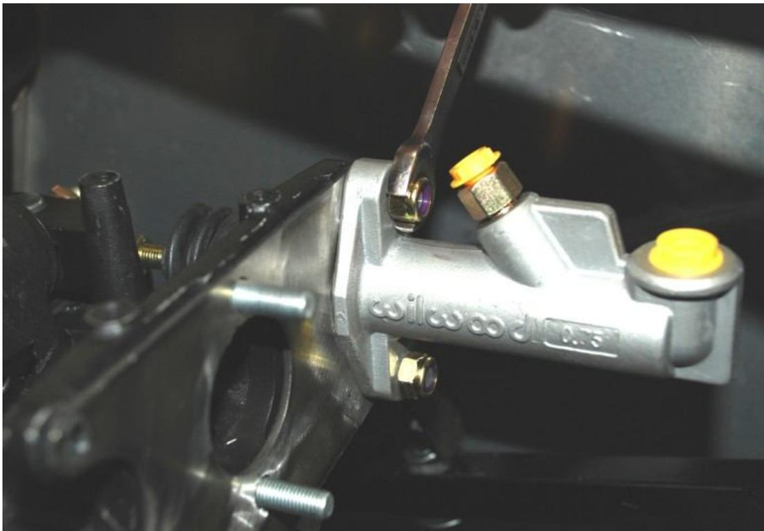
Attach and tighten the locknuts holding the master cylinder to the pedal box then repeat for the other master cylinder.
