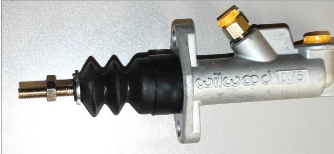
Place a jam nut from the Wilwood pedals onto each of the master cylinder threaded shafts.
