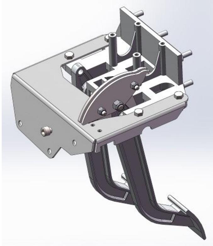
Attach the Wilwood pedals to the underside of the mounting bracket using four hex head screws and locknuts.
