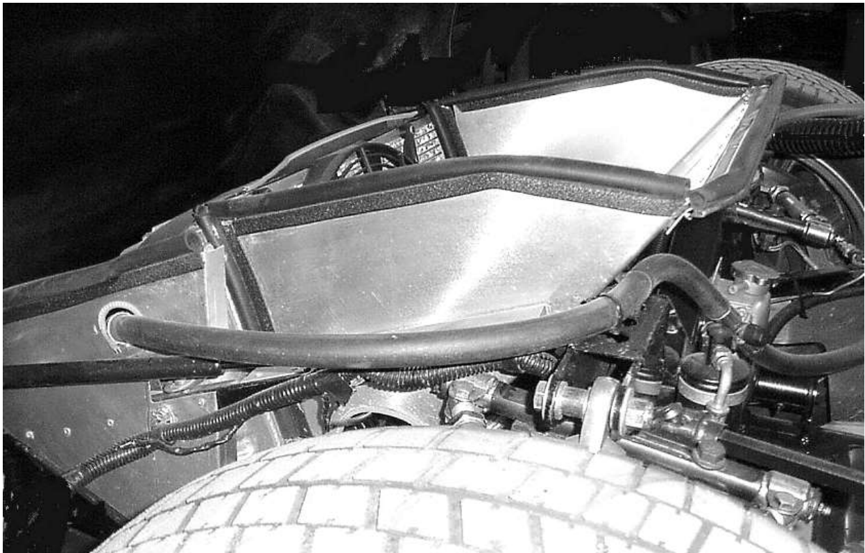
High pressure line going to the condensor through the aluminum.
