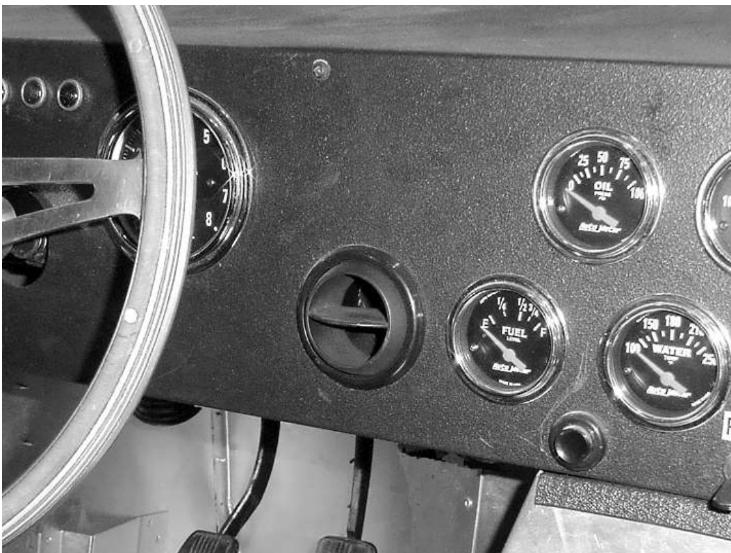
Mount the ball vents in the dash where desired, above is a picture showing the driver side dash vent.
