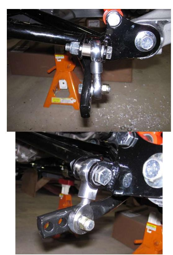
Attach the female rod end to the control arm using the  $\frac{1}{2}$ " bolts and spacers provided and the male rod end to the swaybar using the  $\frac{7}{16}$ " bolts provided.
