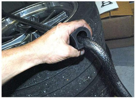
Push the bushings onto the swaybar.
