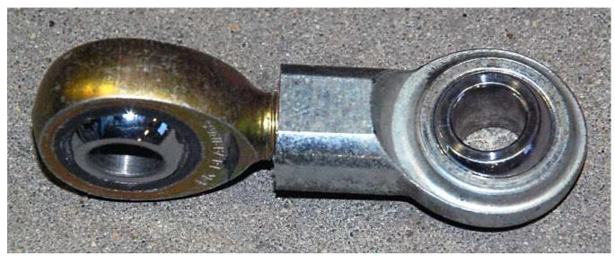
Screw the male and female rod ends all the way onto each other.
