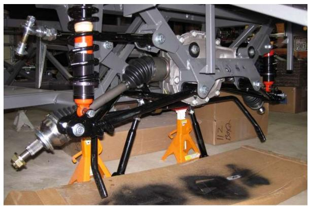
Attach the swaybar bracket to the mount plate holes using a 5/16" hex key and 9/16" wrench.
