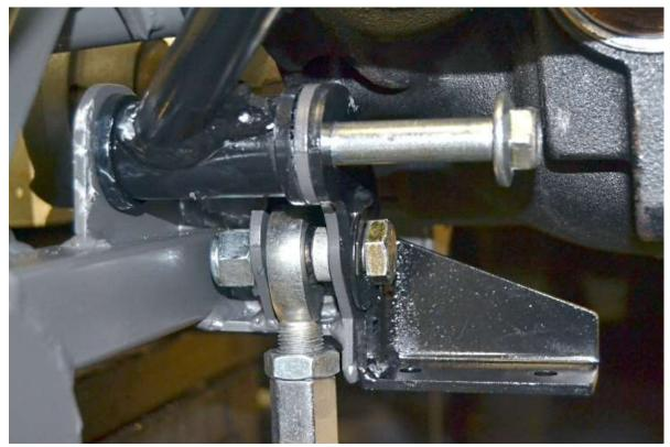
Insert the control arm bolt through the swaybar mount and control arm. Use the new included  $\frac{5}{8}$  x 2.50" bolt for the Toe link.
