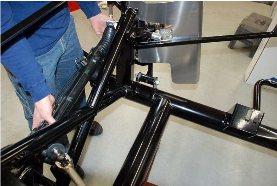
Line up the steering shaft and adapter and push the rack onto the steering shaft.
