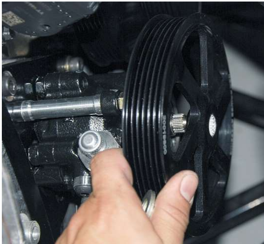
Put the pulley on the pump so the words are visible.
