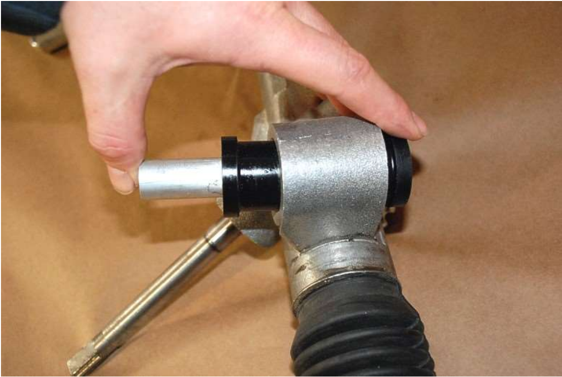
Push the bushings and sleeves into the mounting bosses on the rack.
