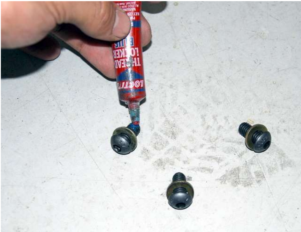
Put blue Loctite on the screws.
