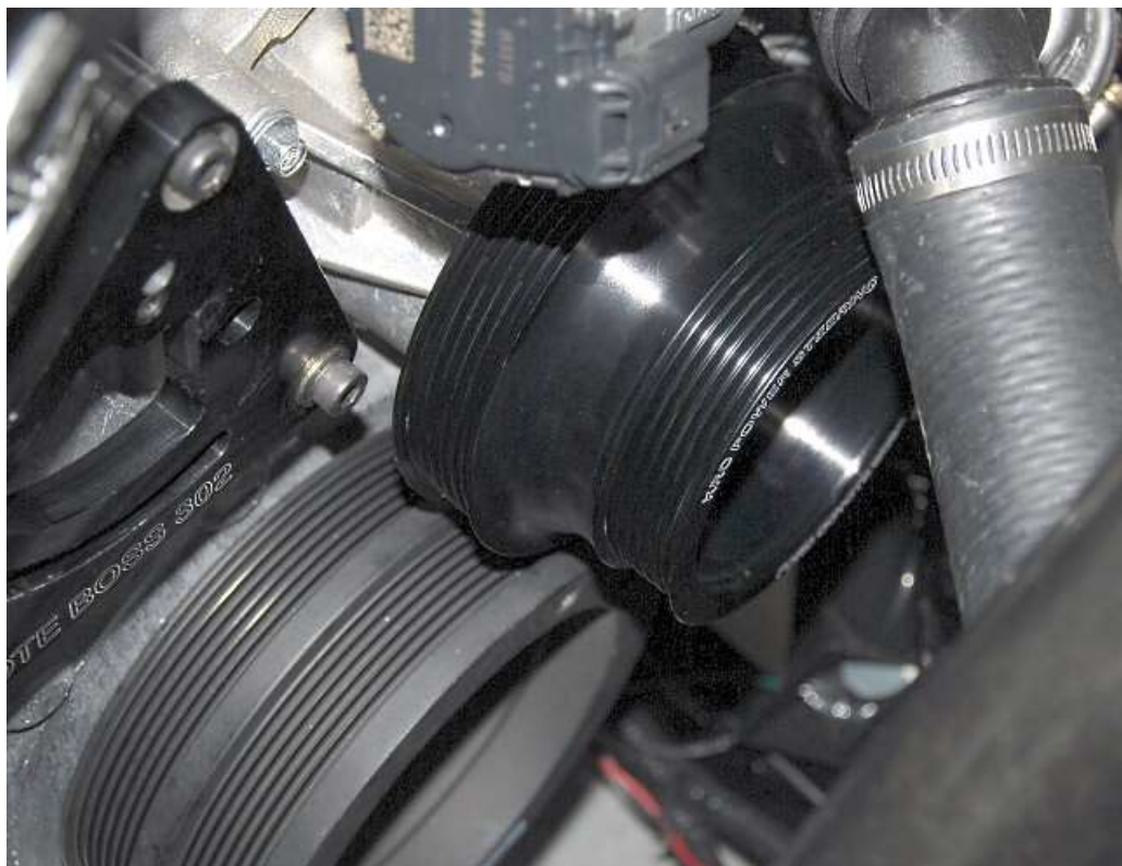
Put the pulley on the water pump and screw the screws in using a 5mm hex key and the belt as a strap wrench.
