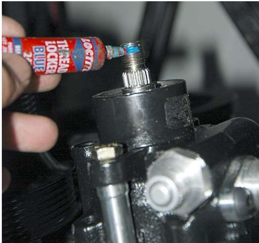
Put Loctite on the pump threads.
