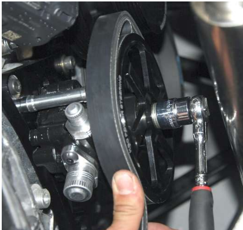
Use the belt as a strap wrench and tighten the pulley nut.
