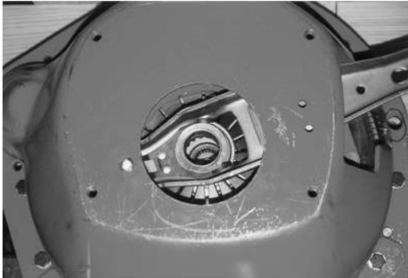
Clutch Fork installed awaiting transmission
