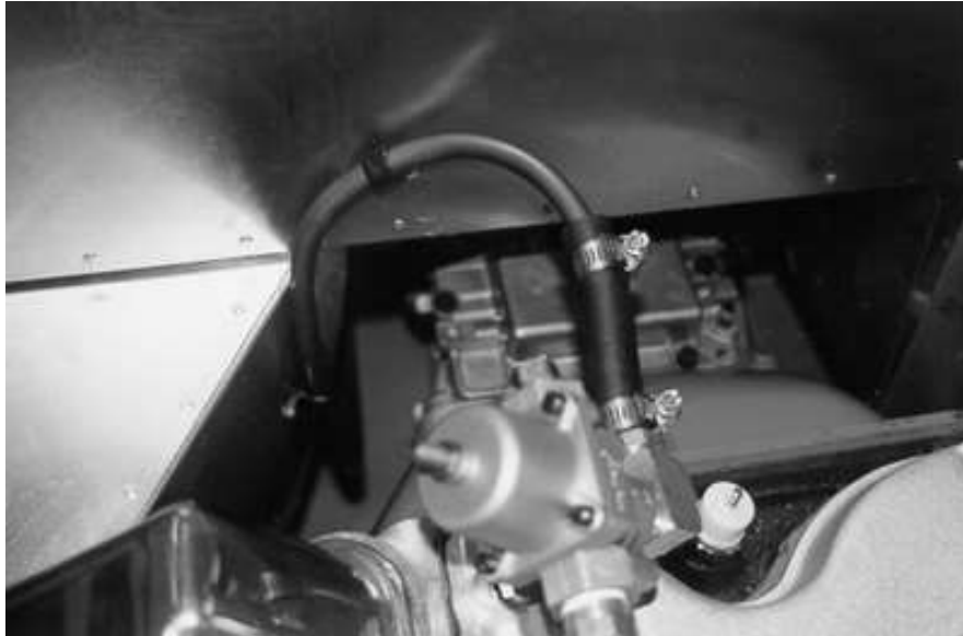
Fuel line and pressure regulator mounted at rear of engine(For carbureted applications)
