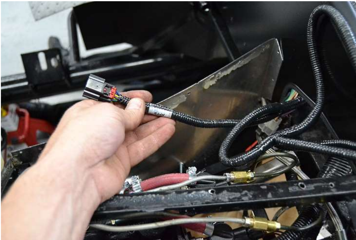
Connect the Accelerator pedal lead (APPS) to the pedal.
