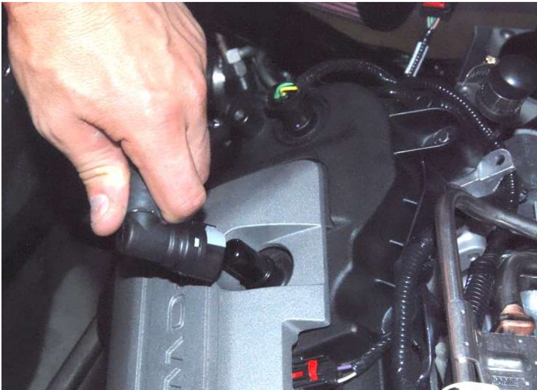
Attach the fitting to the left side valve cover.
