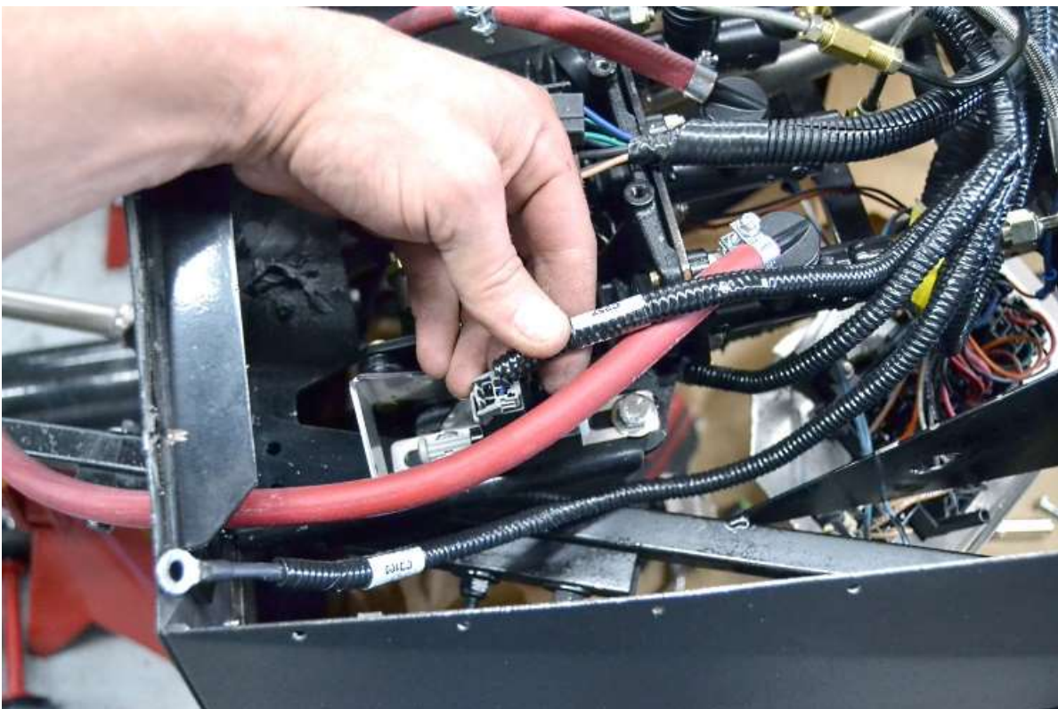
Connect the clutch pedal travel switch leads to the correct switches.
