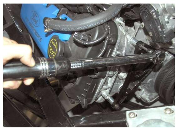
Torque the mounting bolts using a 6mm hex socket to 18lbft.
