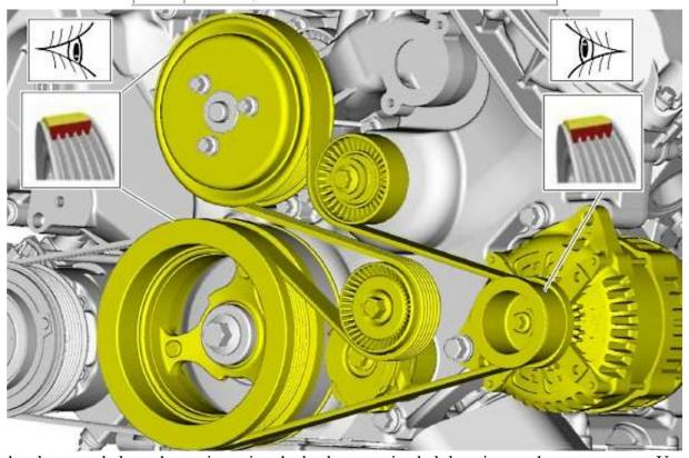
Install the alternator belt on the engine using the back serpentine belt location on the water pump. Use a 15mm socket and ratchet to pull the tensioner
