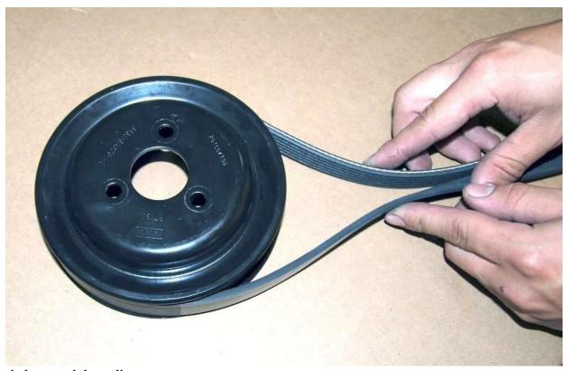
Loop a belt around the pulley.
