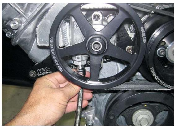
Attach the 90° AN fitting to the pump then the end of the braided line to the fitting using an <sup>11</sup>/<sub>16</sub>" wrench.
