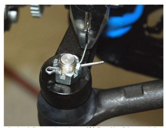
Attach the tie rod to the spindle, torque the castle nut to 25 ft-lbs and install the cotter pin from the kit.
