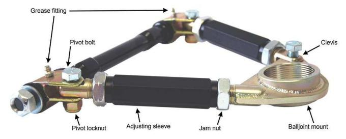
Slightly loosen the three pivot bolts using a 5/8" wrench and socket.
