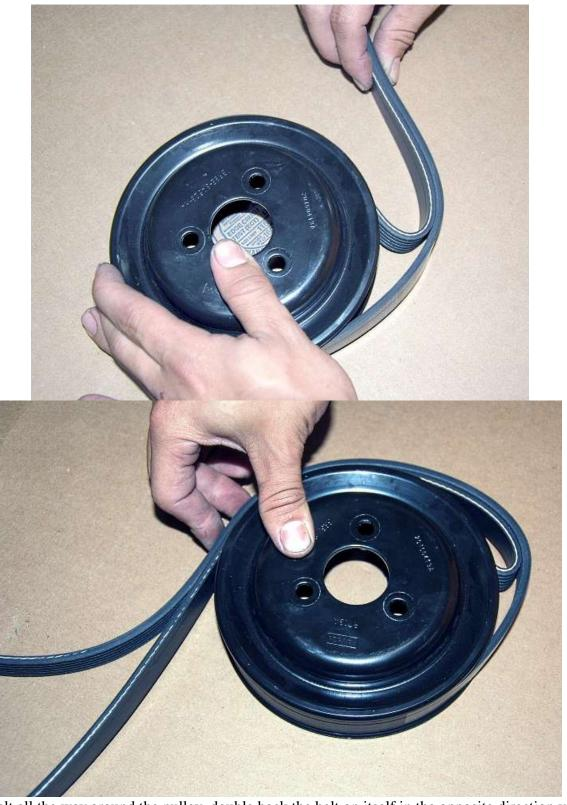
With the belt all the way around the pulley, double back the belt on itself in the opposite direction you are going to turn the wrench. The pictures above shows doubling back for tightening the bolts.
