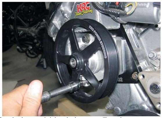
Use a ¼" Hex and ratchet to snug the bolts so that the pump can still rotate for now.
