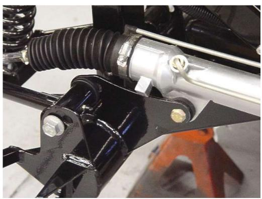
Bolt the rack into the frame. It is easier to do the driver side first then swing the passenger side down into the mount.
