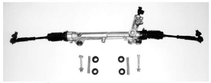
Power steering rack and fasteners.
