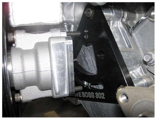
Attach the pump to the bracket. The lower bolt will go into the flange nut in the slot.
