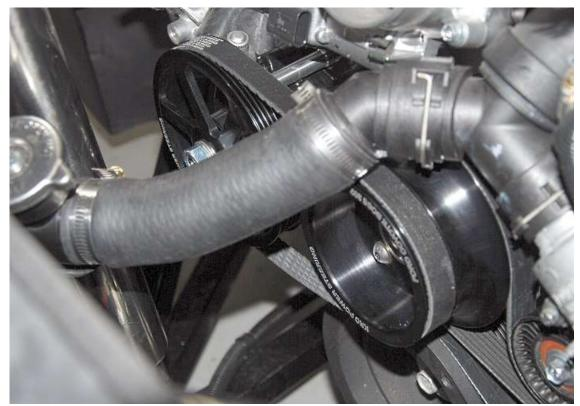
Put the power steering pump belt on the engine.
