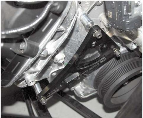
Repeat the bolt assembly and Loctite procedure at the other two bracket locations.
