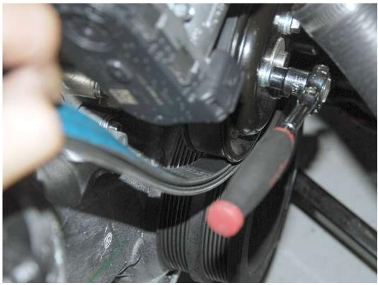
Use the included serpentine belt like a strap wrench to hold the water pump pulley while loosening the bolts with a 10mm socket.
