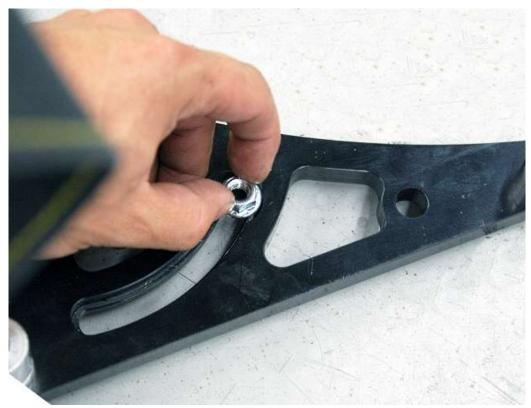
Turn the bracket over and place the flange nut in the slot with the flange first.
