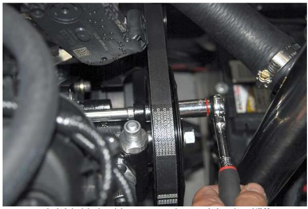
Pull the pump out so the belt is tight then tighten power steering pump bolts using a ¼" Hex.
