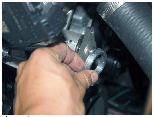
Place the centering ring on the water pump snout.
