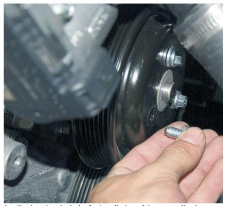
Remove the bolts and pulley keeping the bolts for installation of the new pulley later.
