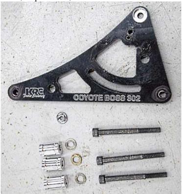
Locate the power steering pump bracket and fasteners.
