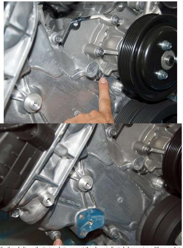
Remove the three bolts on the timing chain cover at the places indicated above using a 10mm socket.
