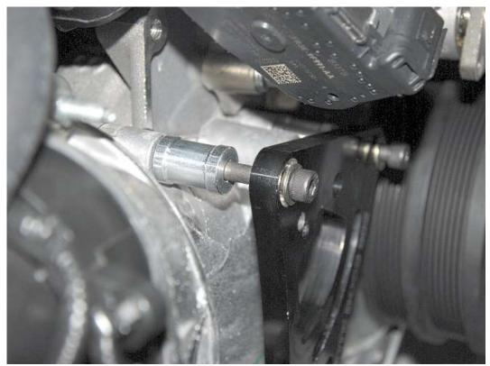
Start the threads for this bolt in the timing chain hole indicated above.
