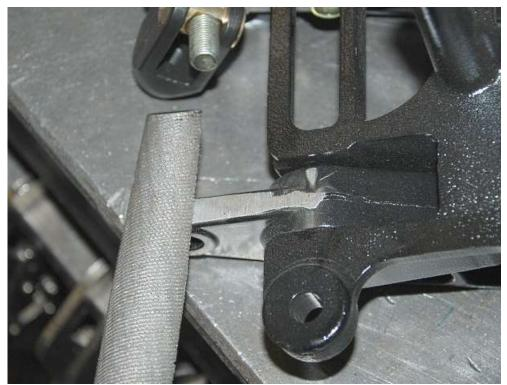
If necessary use a file to remove the forging centerline so the 3/8" bolt can go through the clutch pedal hole.
