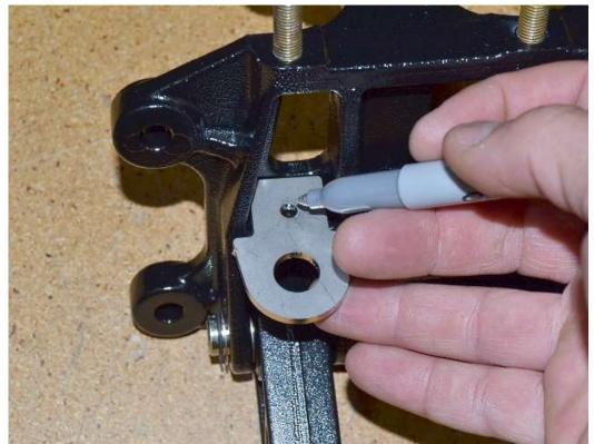
Place the switch mount between the clutch pedal mount tabs on the side closest to the clutch pedal pivot holes and drill a 3/16 hole through the switch mount hole and the pedal box.
