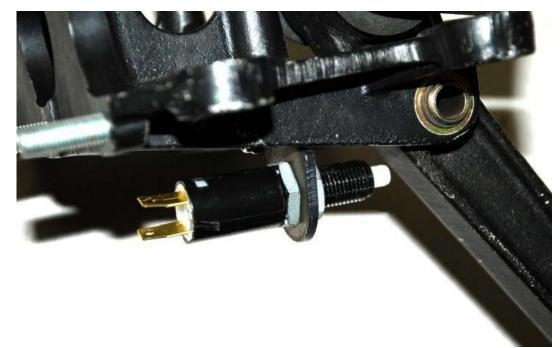
Connect the switch to the switch mount using a hex nut on each side of the mount bracket.
