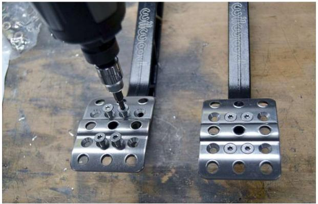
Attach the pedal pads to the pedals using a T-20 Torx bit. The pads mount holes allow the pads to be moved around if desired depending on foot room needed. Start with the pads in the middle holes. Once the seats are mounted in the car the pads can be moved or cut as needed.
