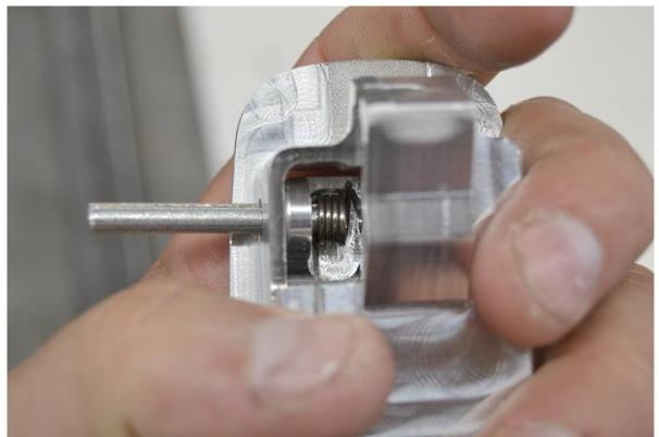
Position the spring as shown with the short end of the spring on the inside of the lever and pointing towards the shorter end of the base using needle nose pliers to push the spring down and onto the spring pin.
