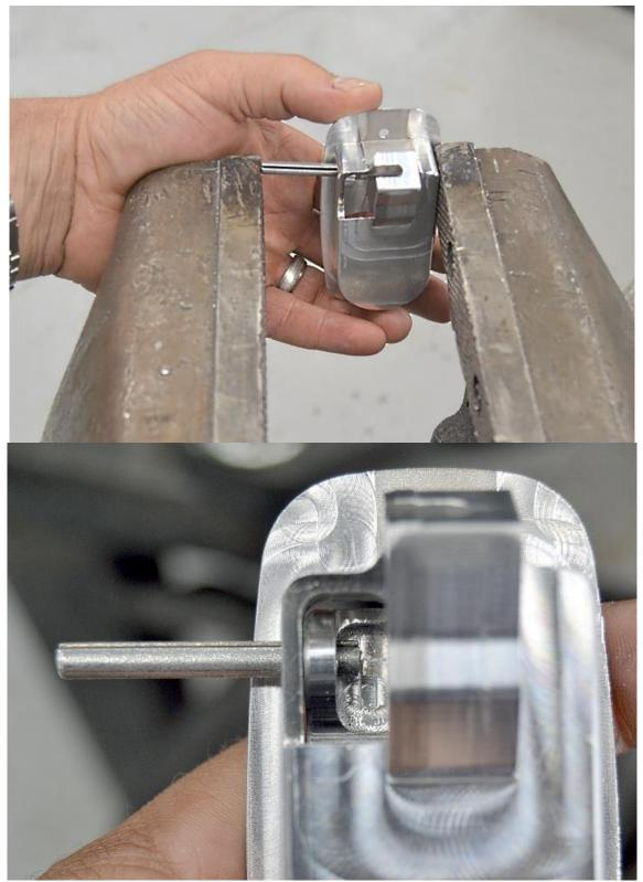
Holding the lever inside the base so that the pivot holes are lined up, push the spring pin from the open side of the base through the base and just into the opening of the lever so that the spring can still fit between the spring pin and inside of the lever.
