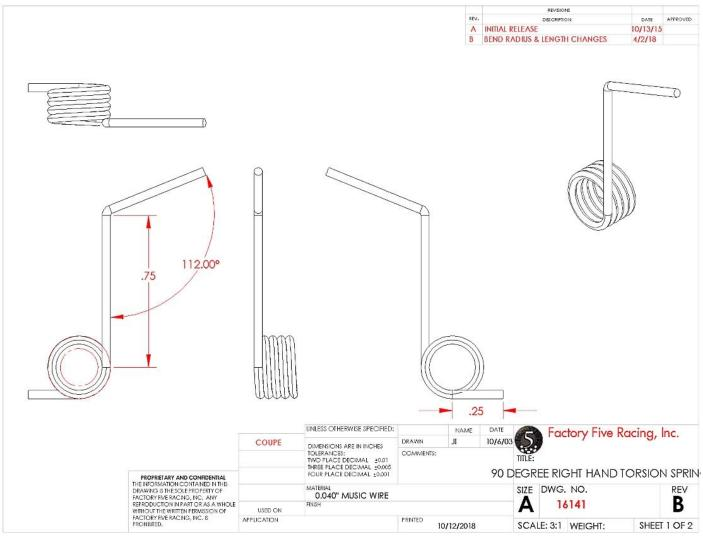
Use the diagram above to bend the spring with the pliers and needle nose pliers at the correct location and angle then cut the other side using the needle nose pliers.
