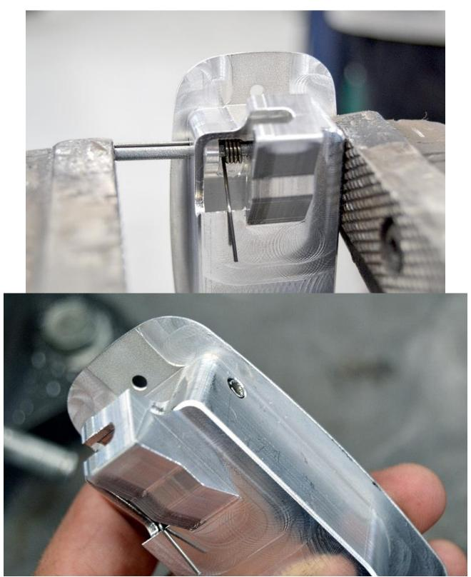
With the spring positioned, push the spring pin through the rest of the lever and other side of the base so that the pin is flush on both sides of the base.
