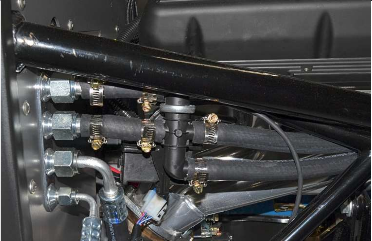
Position the control valve on the engine or the firewall between the bulkhead fitting and the engine heater fittings.
