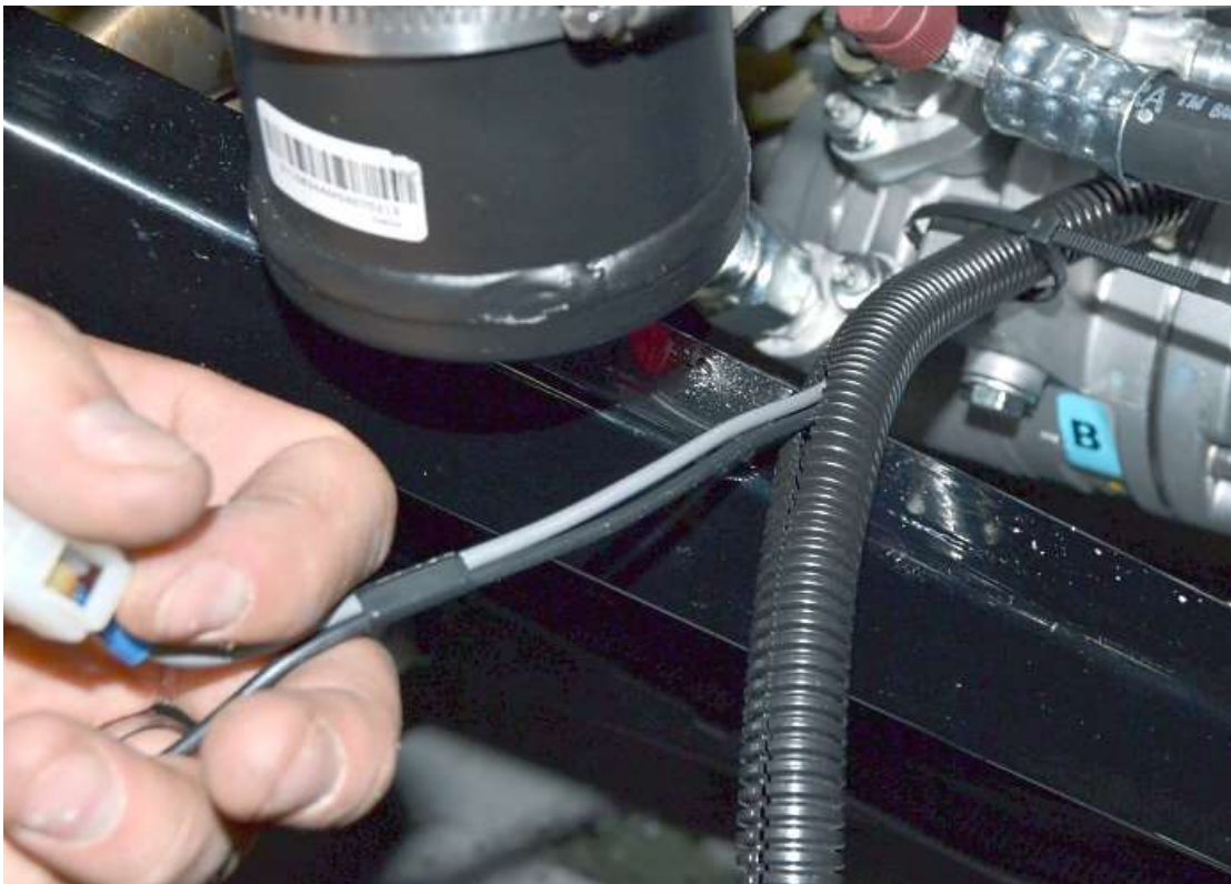
Starting at the compressor, put the gray and black wires in the conduit.
