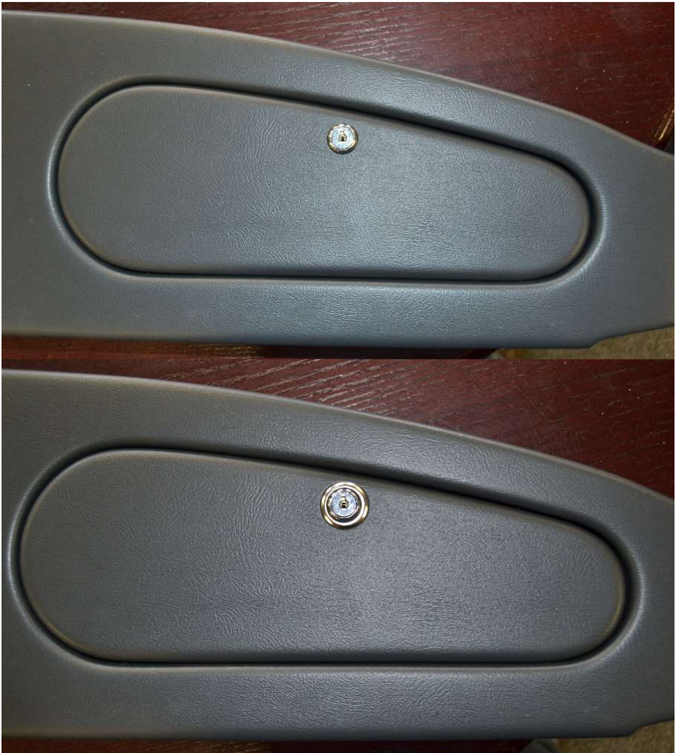
The glove box lock can be used with or without the trim ring as desired.
