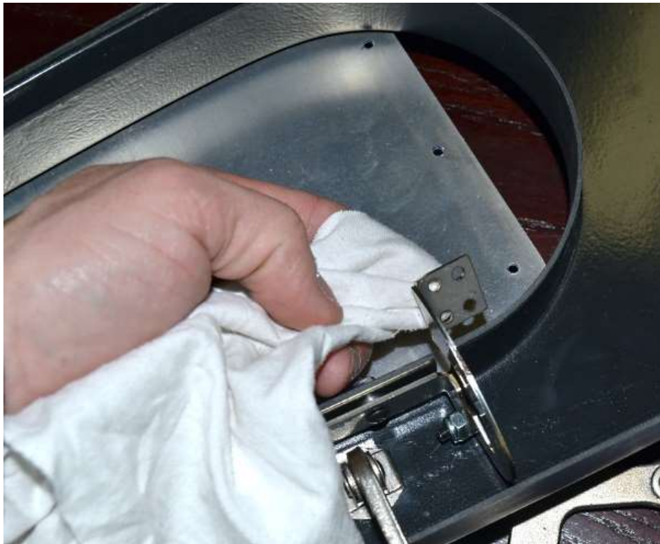
Wipe the hinge arm tabs with cleaner.
