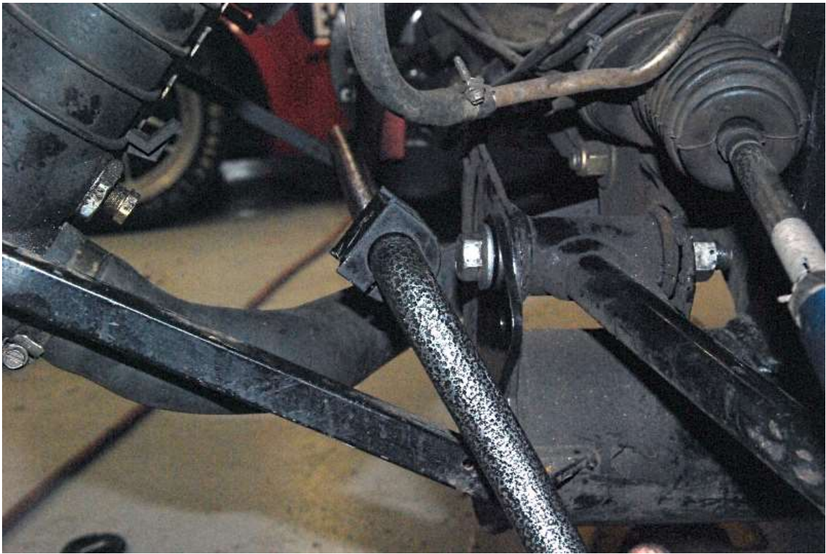
Position the swaybar on the car above the lower radiator mount tubes and lower radiator hose.
