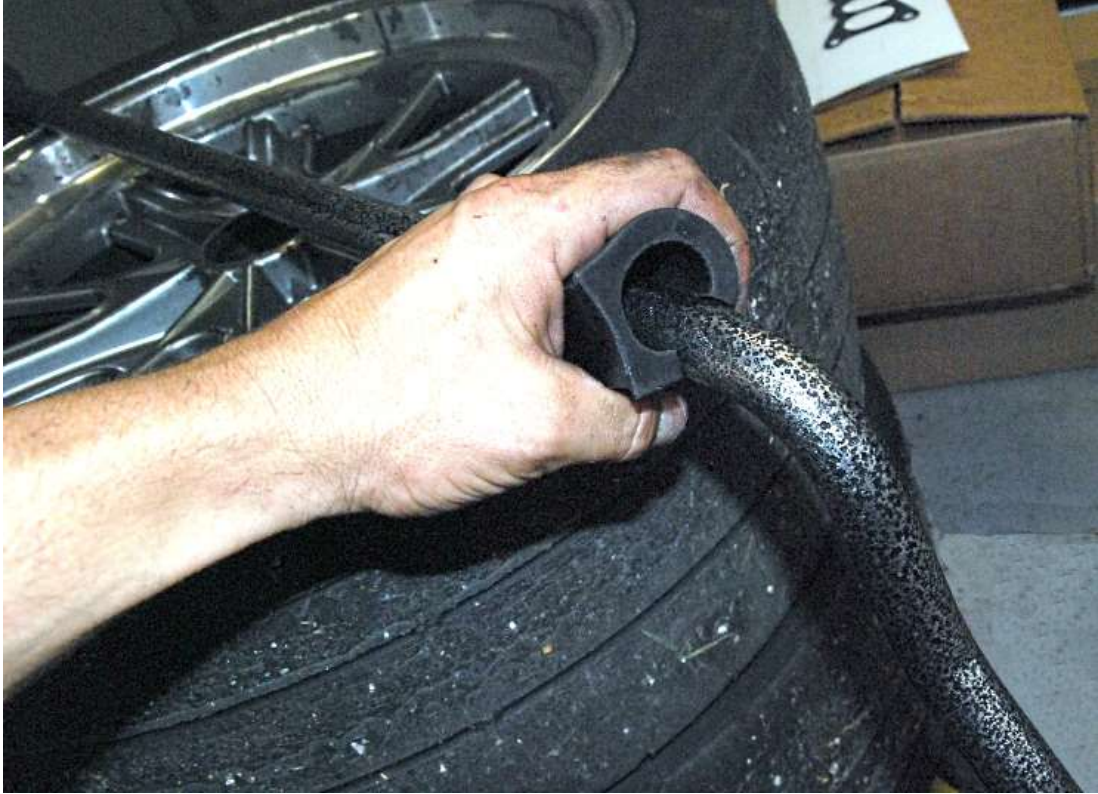
Push the bushings onto the swaybar.
