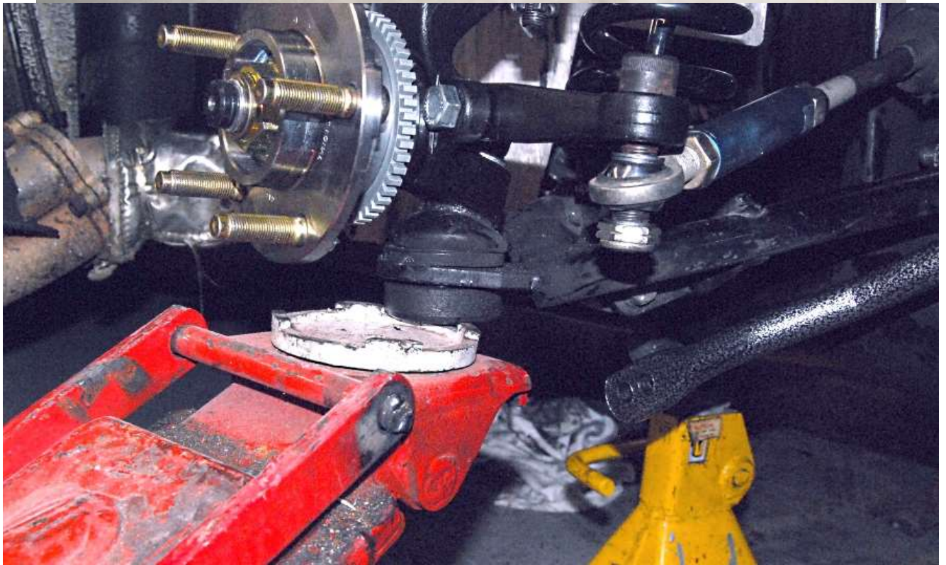
Place the jack under the lower control arm balljoint without hitting the grease fitting.
