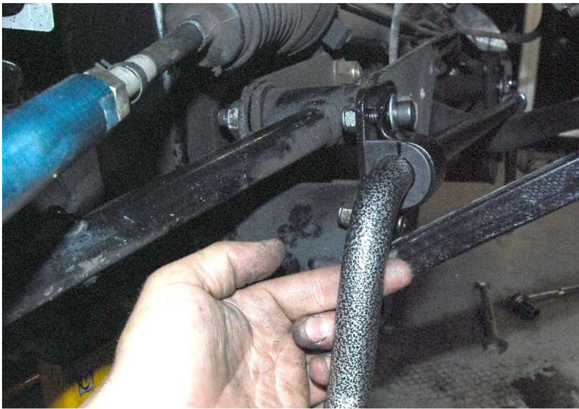
Attach the lower swaybar bracket mounting bolts using a \frac{5}{16} " hex key and \frac{9}{16} " wrench.
