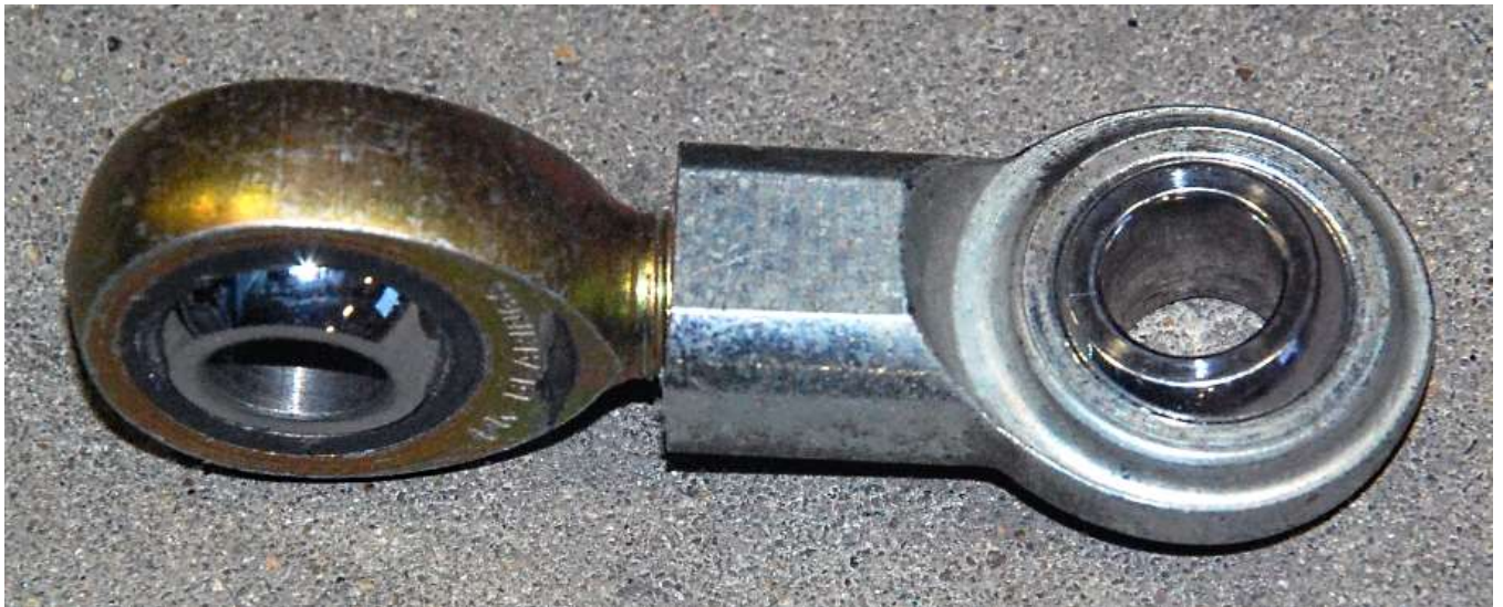
Screw the male and female rod ends all the way onto each other so they are 90° from each other.
