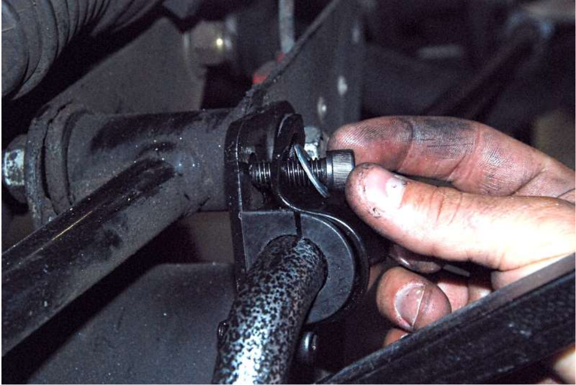
Attach the swaybar bracket to the top mount plate holes using a \frac{5}{16} " hex key and \frac{9}{16} " wrench.
