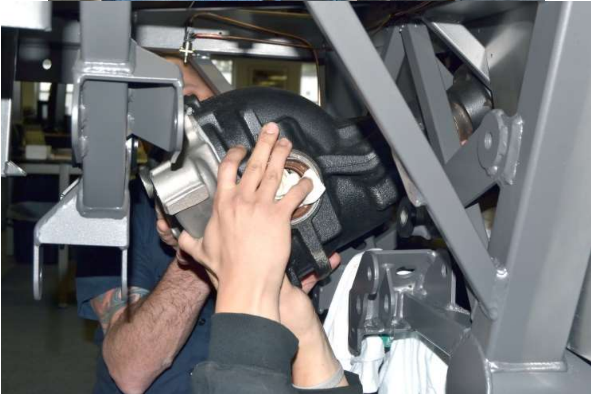
With the help of a friend, lift the center section nose up into the frame and over the front mount.
