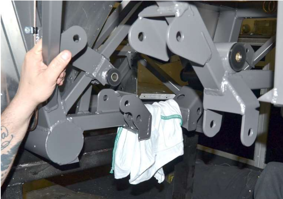
Use rags to protect between the front center section mount on the frame.
