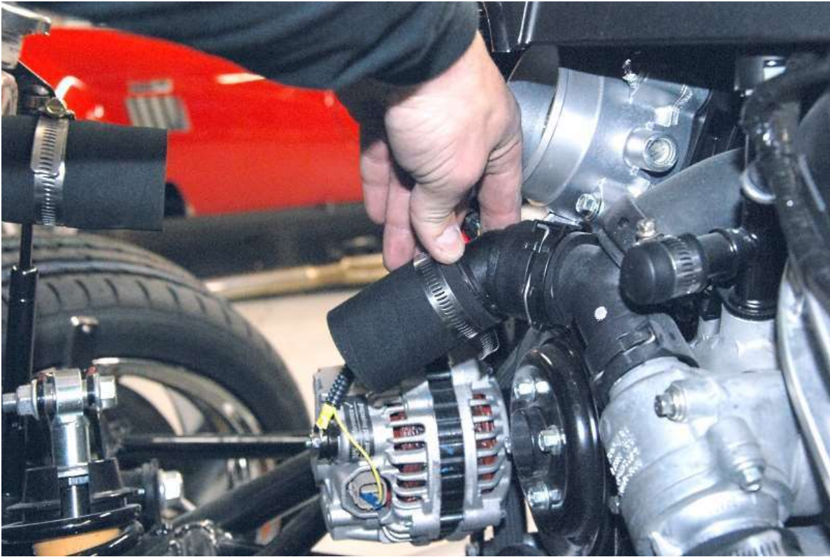
Push the adapter onto the engine.
