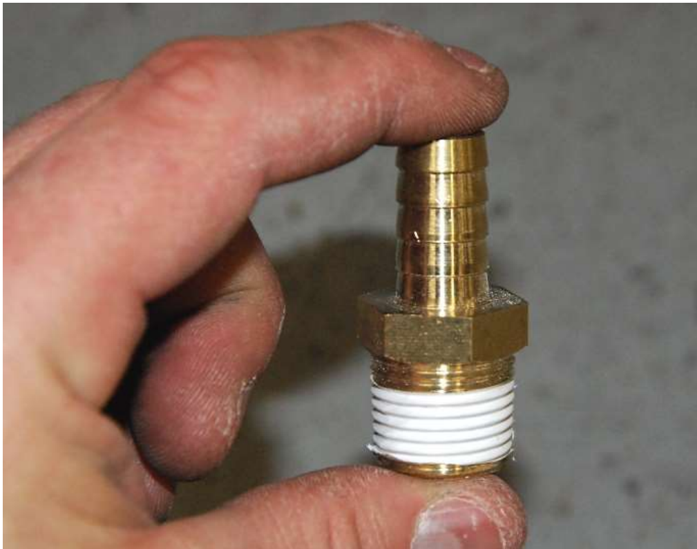
Use Teflon tape on the hose fittings.
