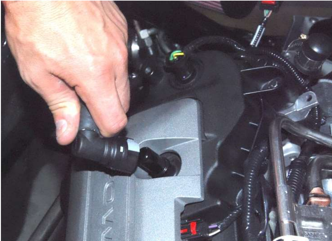
Attach the Right PCV fitting to the left side valve cover.
