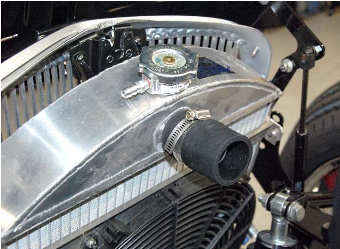
Attach another hose adapter to the radiator.
