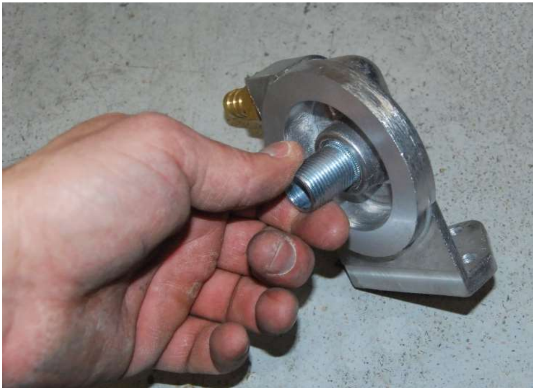
Screw the threaded nipple into the relocater.
