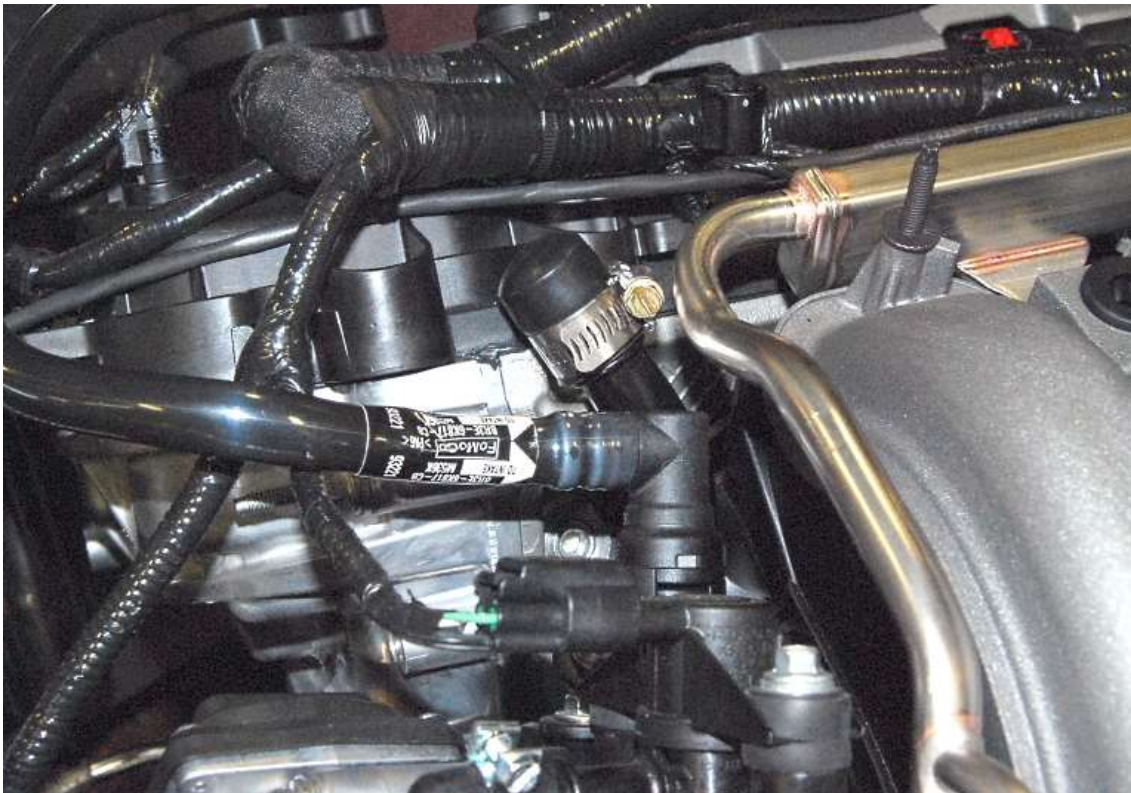
Cap and hose clamp the 3/4" coolant.
