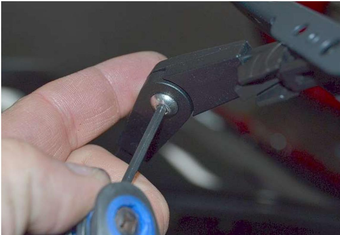
Tighten the screw at the end of the arm holding the angle using a 2.5mm hex key.
