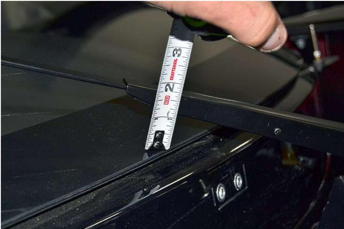
Check the clearance to the glass at the bottom of the glass. It needs to be less than  $\frac{5}{8}$ " from the glass to the bottom of the arm.
