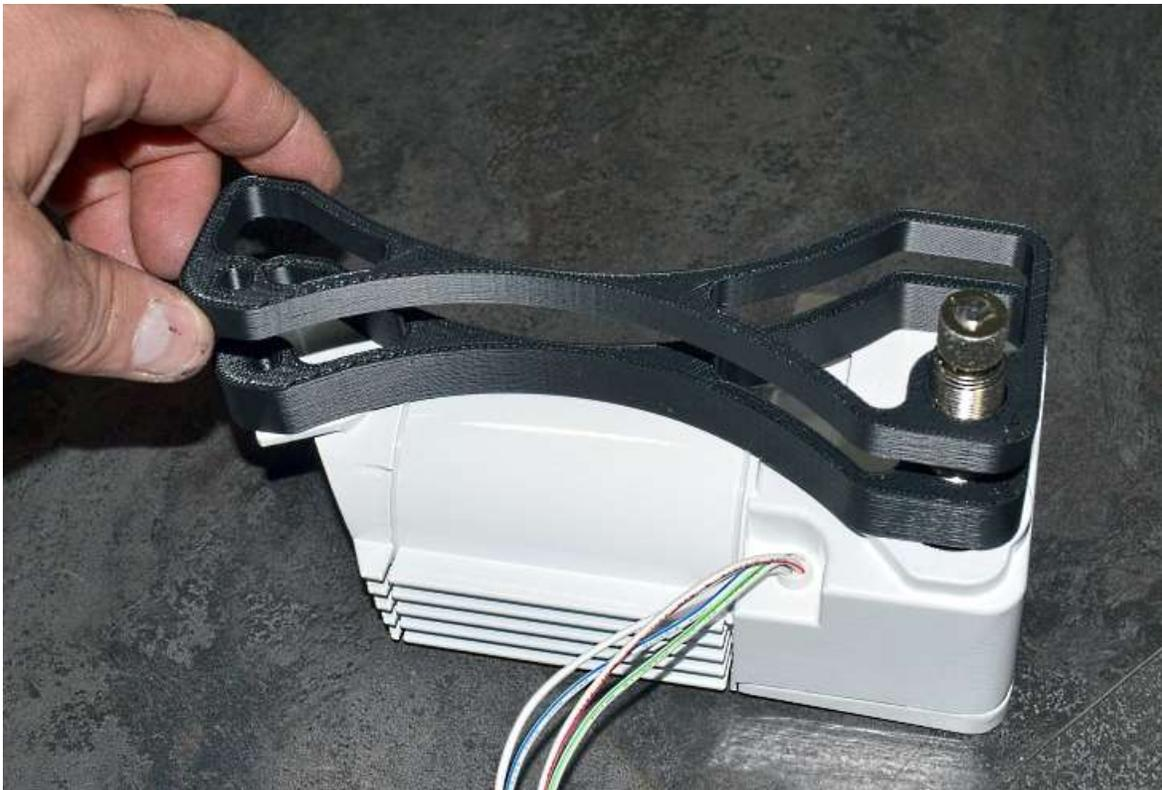
If the gap is too high, remove the wiper mount and wiper motor and add the other spacer.
