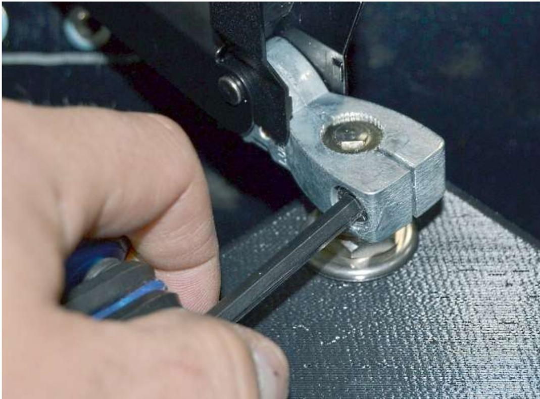
Tighten the arm on the motor using a 5mm hex key.
