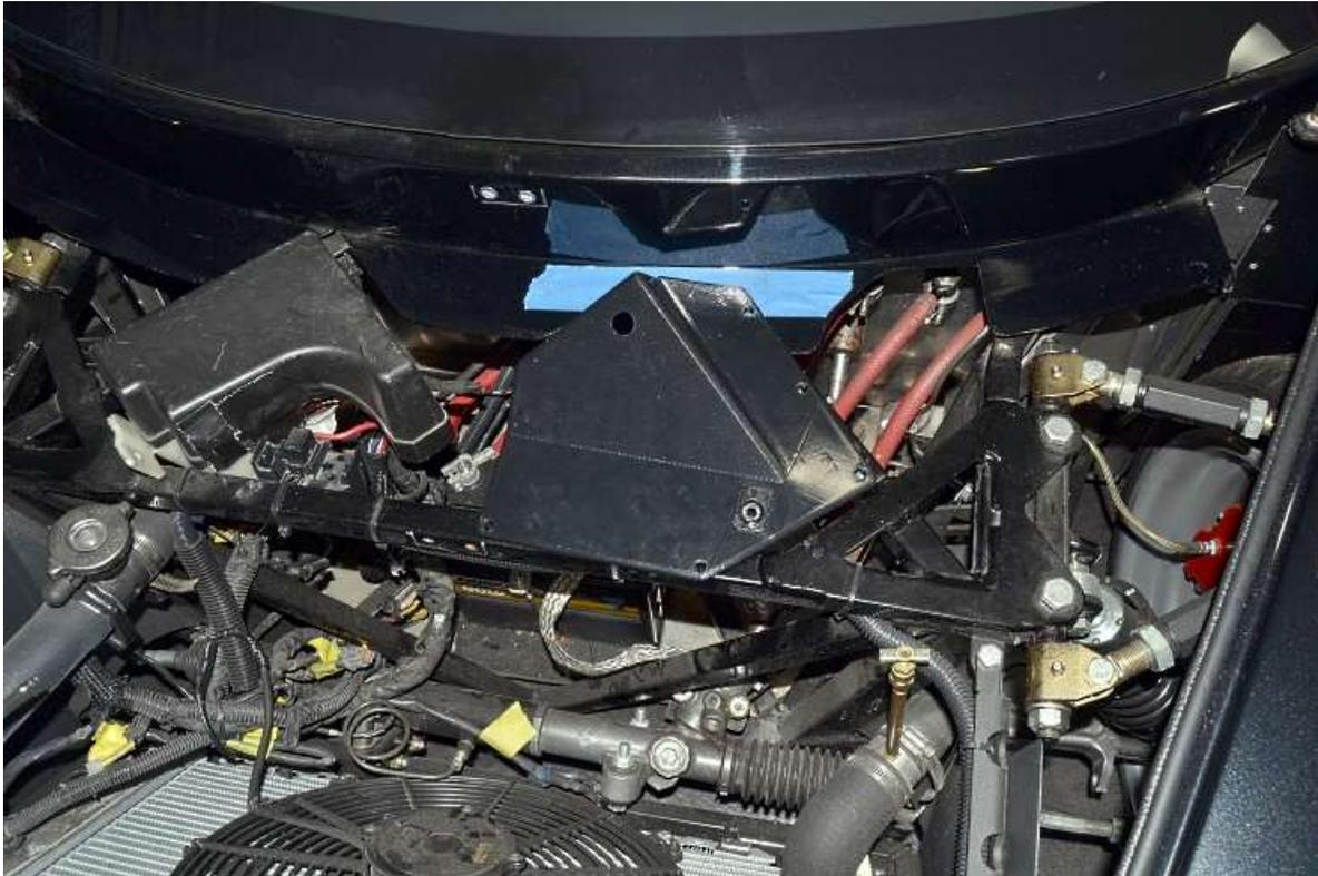
Place the wiper mount onto the chassis. It mounts at the base of the windshield on the driver's side with the front edge on the horizontal tube between the upper control arms. Depending on how your windshield surround is mounted, you may need to trim the edge of the surround and the wiper mount may need to slide under the windshield surround flange. Put some masking tape down then replace the mount.
