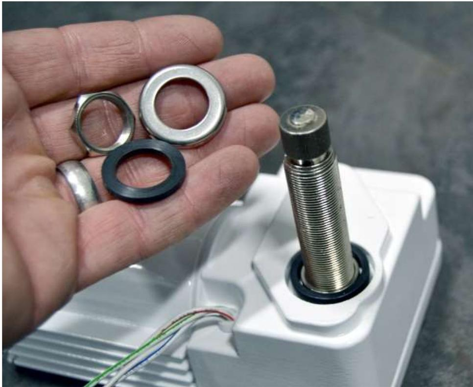
Remove the nut, trim pieces and wider rubber gasket from the motor shaft.
