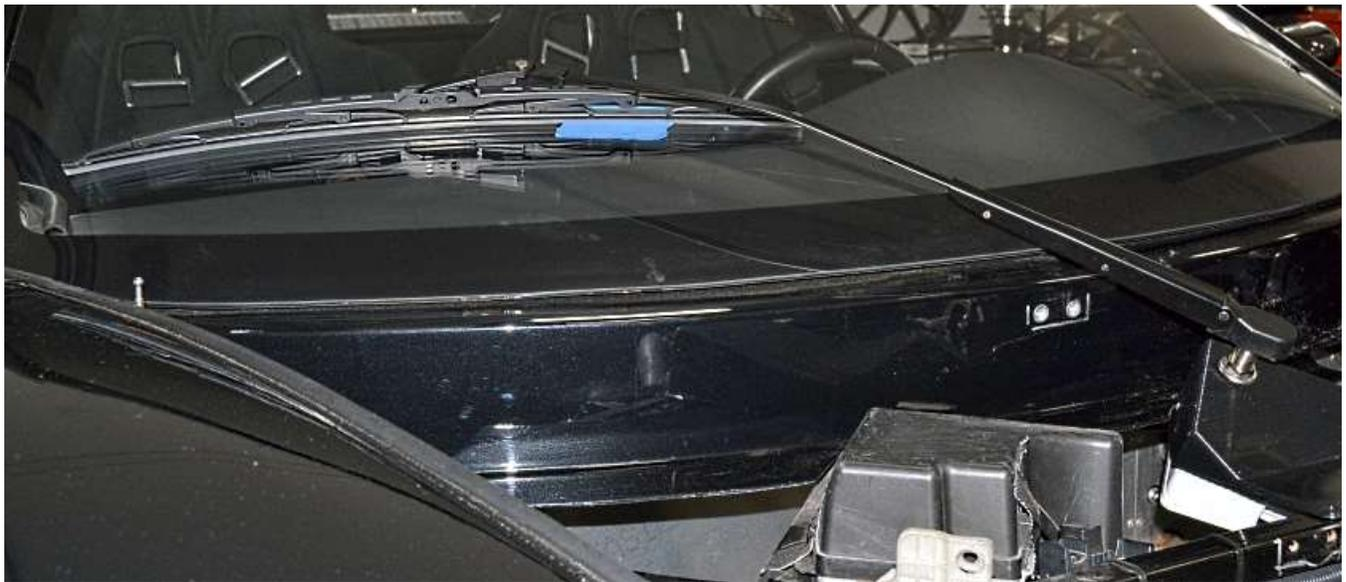
Because of the curve of the glass, you will need to bend the arm slightly so that the blade rests properly on the glass.
