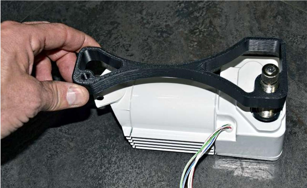
The kit comes with two spacers, one  $\frac{3}{8}$ " and one  $\frac{5}{8}$ ". You will need to use at least one of them to get the wiper arm down close to the glass. Start with the  $\frac{5}{8}$ " spacer and place it over the shaft aligning the small hole on the motor at the other end.
