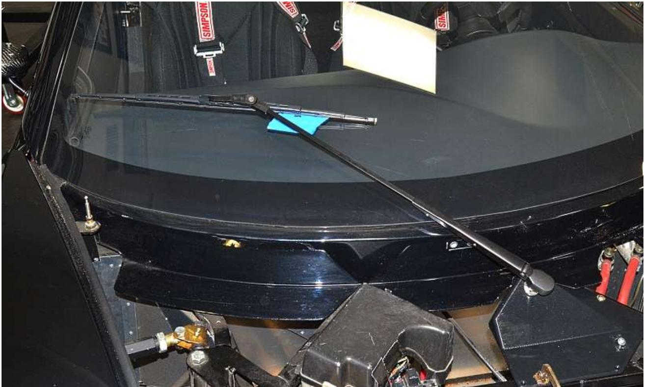
The blade parks at the base of the windshield on the right side. Adjust the angle of the blade at the end of the arm and attach the arm to the motor so that the blade will sit where the mark is on the tape.
