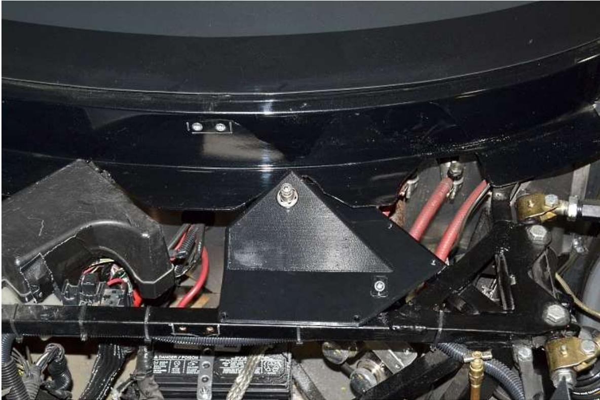
Reposition the motor on the frame then using the included self-drilling screws and  $\frac{5}{16}$ " socket, bolt the mount to the chassis.
