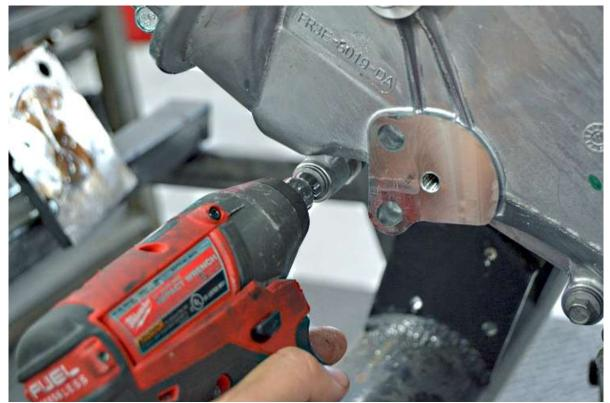
Remove the three bolts on the timing chain cover at the places indicated above using a 10mm socket.
