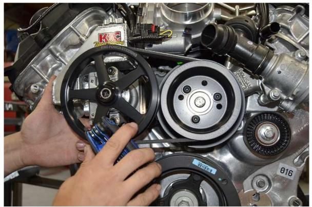
Pull the pump out so the belt is tight then tighten power steering pump bolts using a <sup>1</sup>/<sub>4</sub>" Hex.
