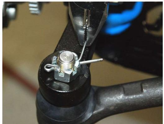
Attach the tie rod to the spindle, torque the castle nut to 25 ft-lbs and install the cotter pin from the kit.
