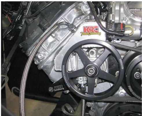
Route the return line next to the pressure line and attach it to the fitting on the tank.
