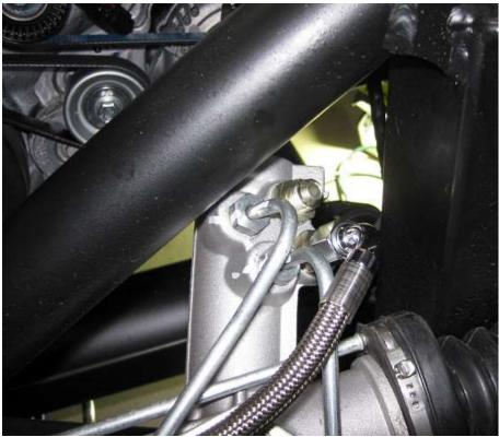
Attach a braided line to the lower steering rack pressure (send) fitting using the 90° end.
