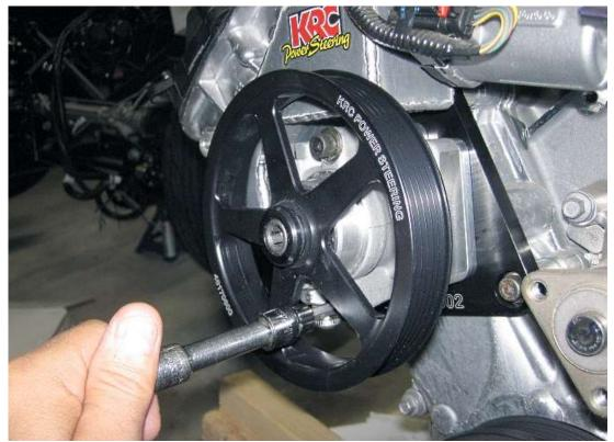
Use a <sup>1</sup>/<sub>4</sub>" Hex and ratchet to snug the bolts so that the pump can still rotate for now.
