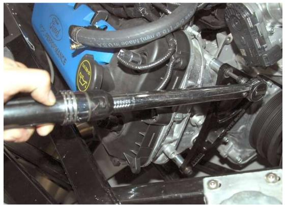
Torque the mounting bolts using a 6mm hex socket to **18lbft**.
