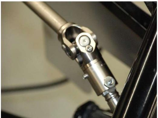
Line up the steering shaft and adapter and push the rack onto the steering shaft.
