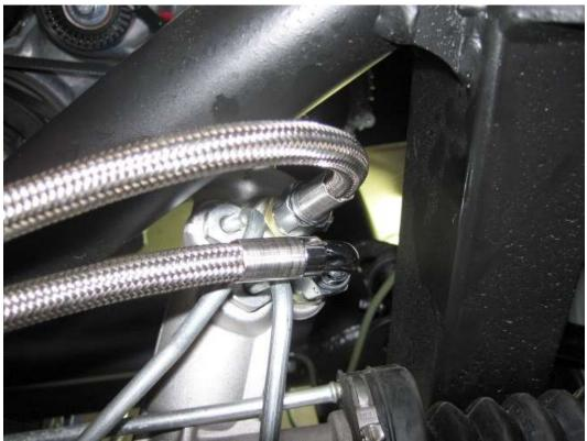
Attach the 90 degree AN fitting and straight hose end to the return connection on the rac. Leave the fitting slightly loose for now until the other end of the hose is put on.
