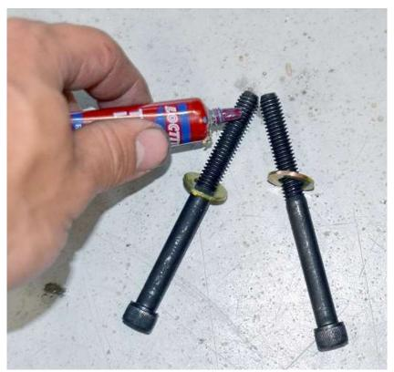
Place a washer on each of the scress then put a drop of blue Loctite on the screws.
