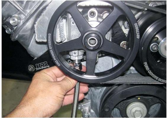
Attach the 90° AN fitting to the pump then the end of the braided line to the fitting using an 11/16" wrench.
