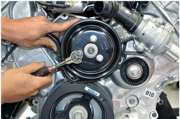
Use an impact wrench if available or the included serpentine belt like a strap wrench to hold the water pump pulley while removing the bolts with a 10mm socket.
