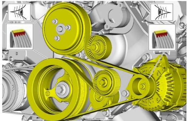
Install the alternator belt on the engine using the back serpentine belt location on the water pump. Use a 15mm socket and ratchet to pull the tensioner
