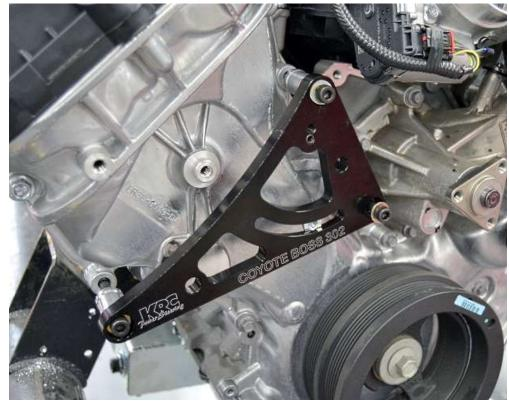
Repeat the bolt assembly and Loctite procedure at the other two bracket locations.
