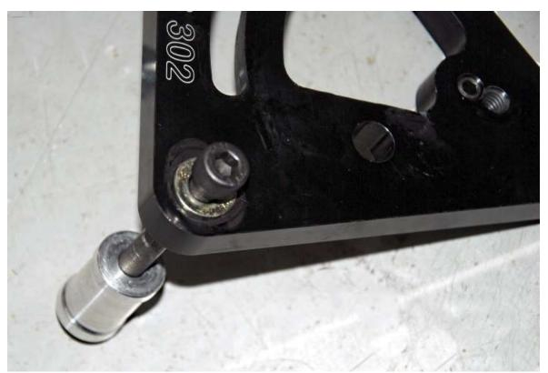
Starting at the bottom right bracket hole, put a washer on the bolt then pass the bolt through the bracket and spacer.
