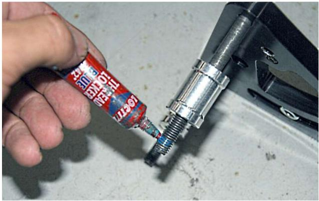
Use a small amount of blue Loctite on the bolt threads.
