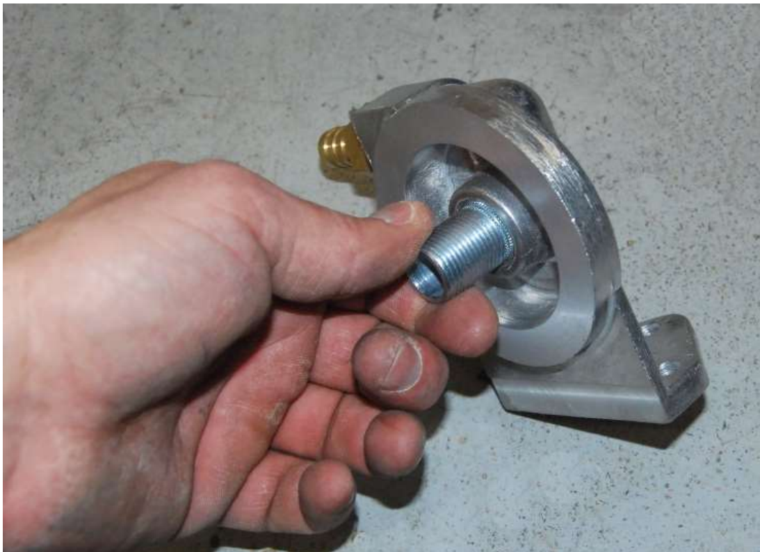
Screw the threaded nipple into the relocater.
