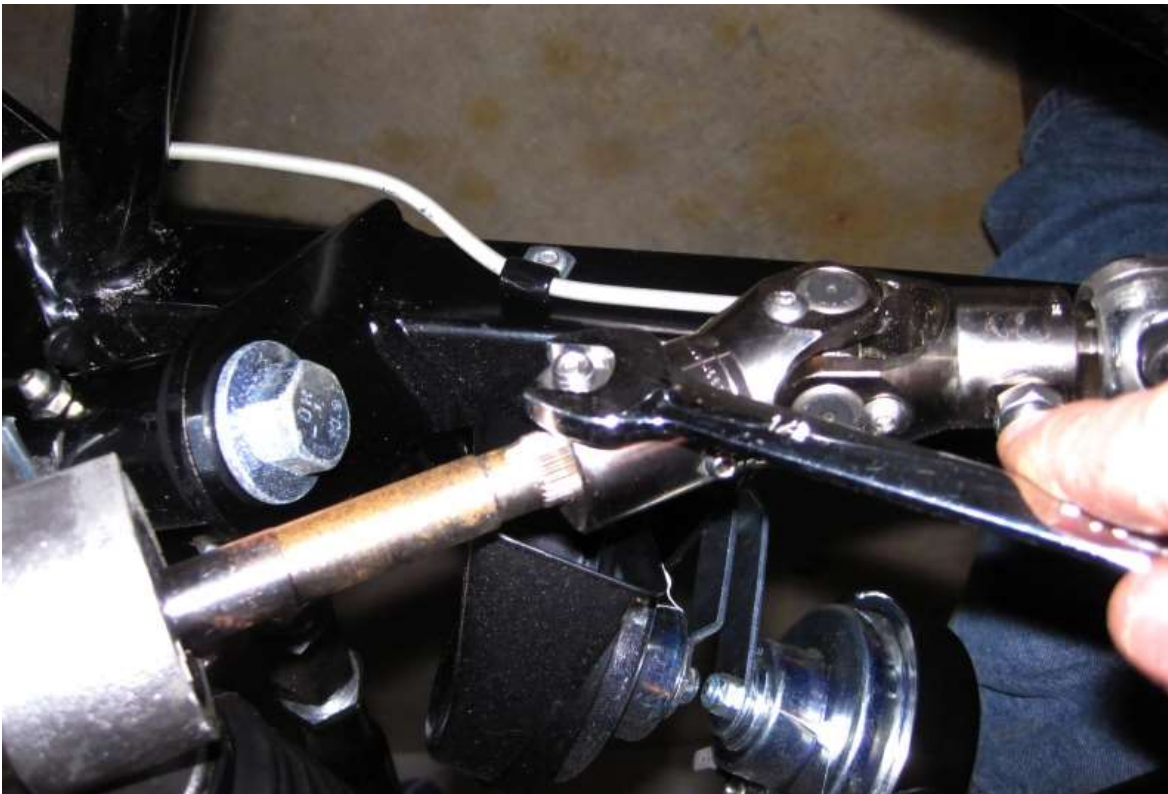
Tighten all of the set screws, jam nuts and flange bearing fasteners. Don't forget to Loctite the small set screw on the firewall joint.
