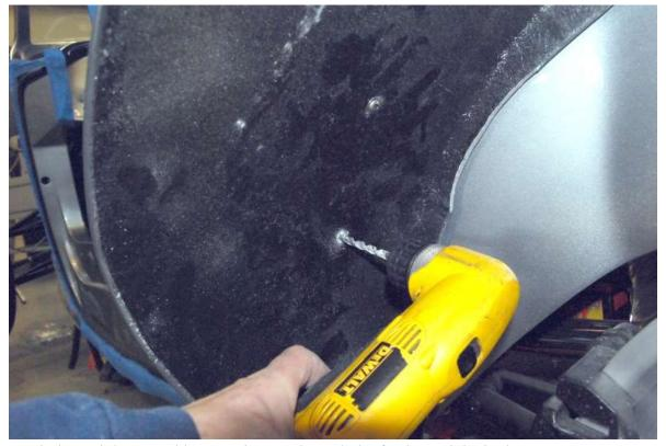
Drill a  $\frac{3}{16}$ " hole straight up making sure it goes through the fender and the body.
