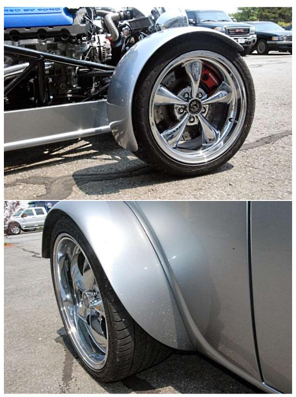
It is recommended to keep the fender low in the back so that any stones or sand that is thrown up is kept to a minimum.
