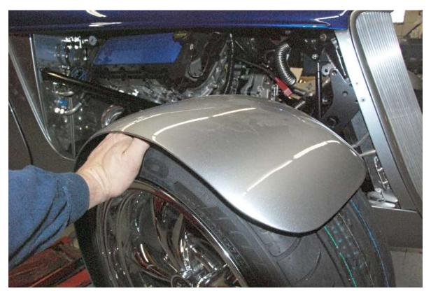
Recheck clearance between the fender and tire.
