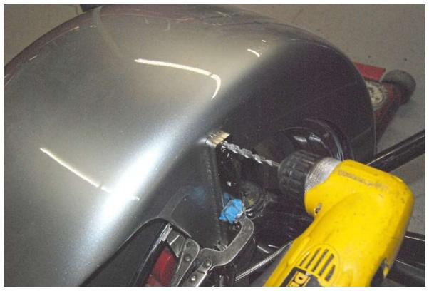
Use the fender mount holes as a guide to mark the 1/4" bolt holes in the fenders using a 1/4" drill bit.
