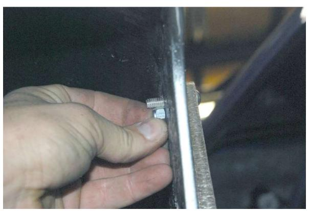
Check to make sure that the screw will go completely through the locknut. If necessary remove material from the fender.
