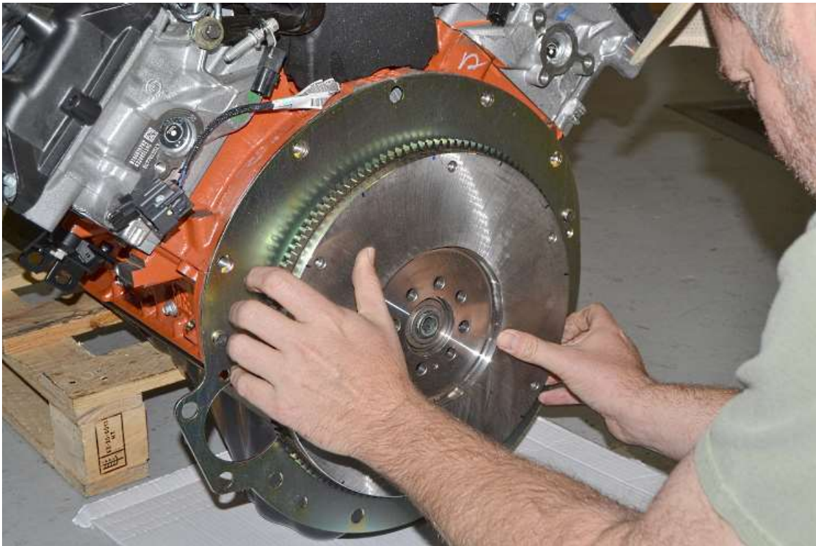
Install the flywheel using red Loctite on the bolts.
