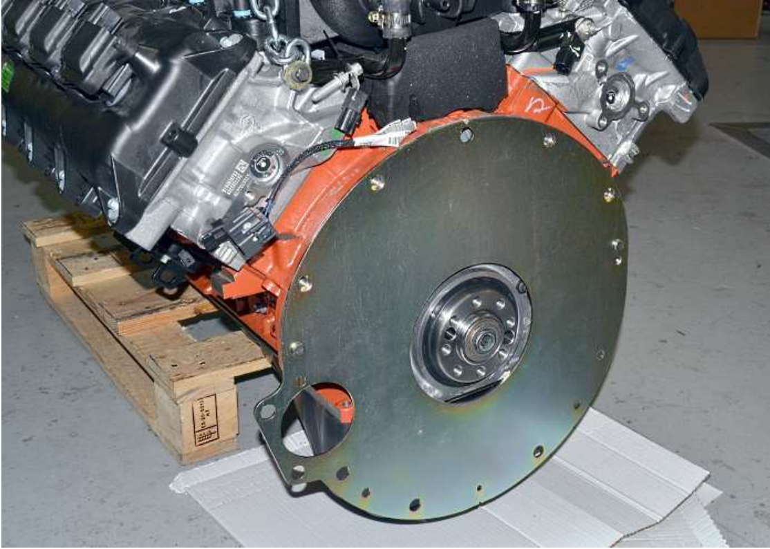
Position the backing plate for the scatter shield on the engine before the flywheel is installed.
