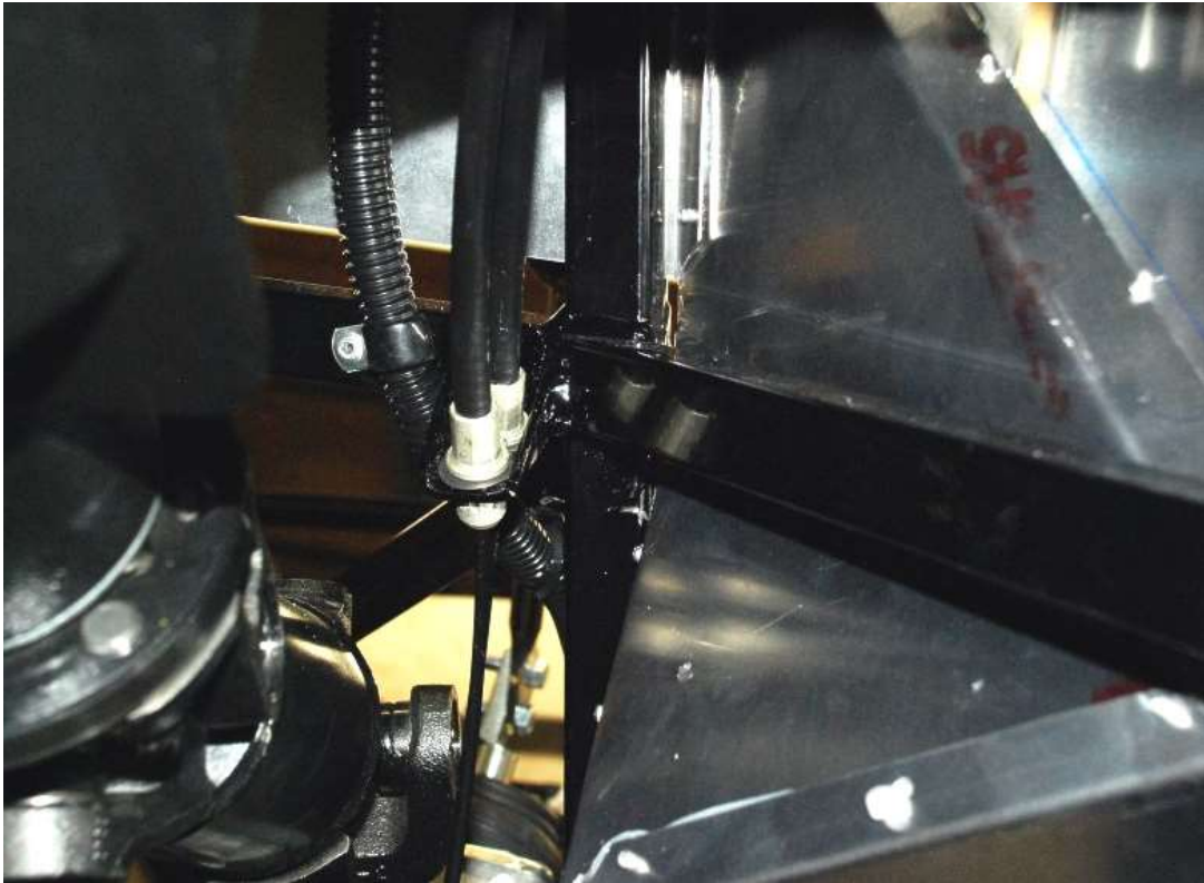
Insert the cables until the sheath end clicks in place. Roadster shown.
