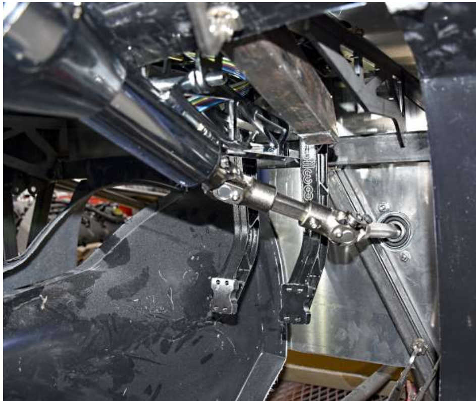
Attach the inside shafts and joints. Picture does not show the rod end installed. The Rod end must be installed.
