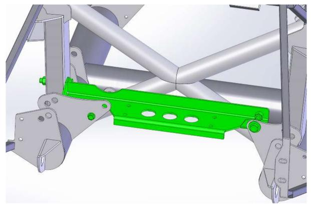
Insert the bracket between the X and the control arm mount as shown.
