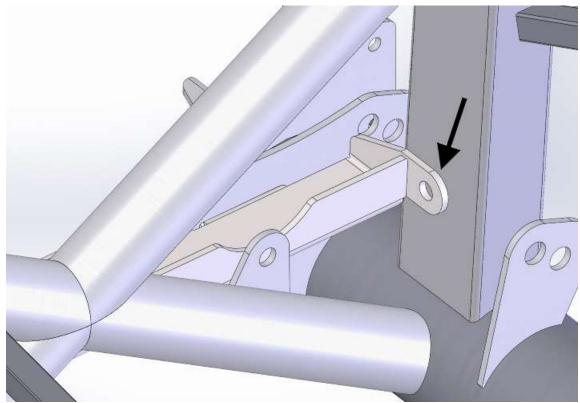
Mark the mounting hole on the 2"x 3" tube.
