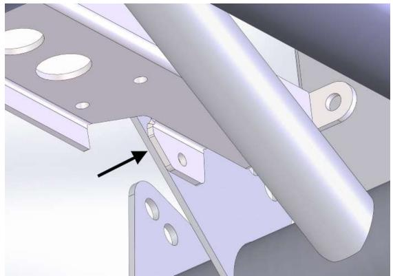
Adjust the bracket so that it is level using either a level or check the right front mount should be flush with the edge of the bracket.
