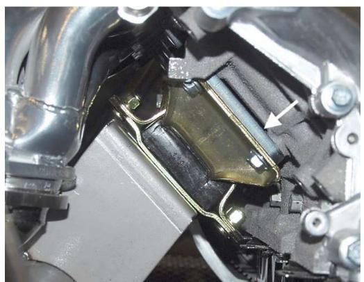
Attach the included engine mount space to the right side of the engine.
