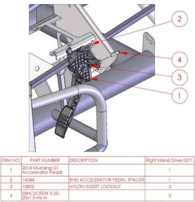
Attach the accelerator pedal to the frame using the spacer behind the pedal in the top left hole.
