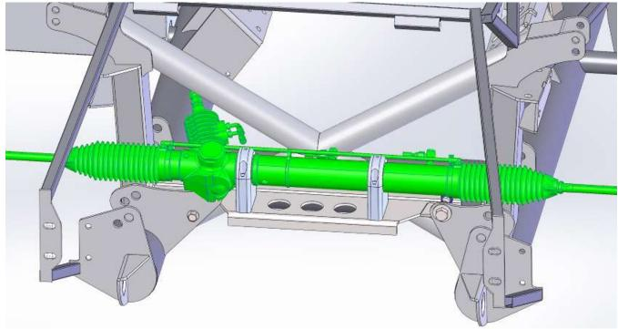
Insert the rack into the mounts.
