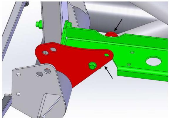
The two right side steering rack mounts will have to be trimmed so that the rack does not hit them.
