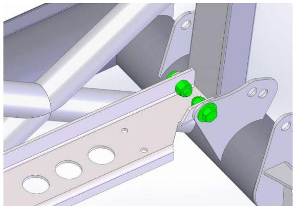
Insert the two  $\frac{1}{2}$ " x 1.25" bolts on the left side of the steering rack mount into the two slots on the frame. Do not tighten the bolts yet.
