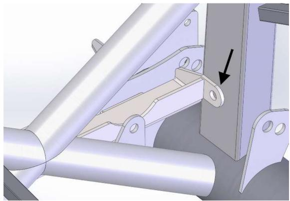
On the right side move the mount over so that the bracket will touch the 2"x 3" tube.
