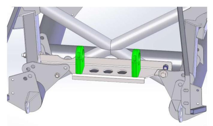
Attach the rack mounts to the frame using the 3/8" x 1" socket head screws. Do not tighten until the rack is installed.
