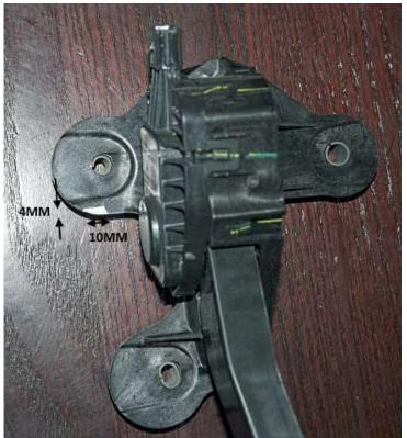
Mark the accelerator pedal as shown.
