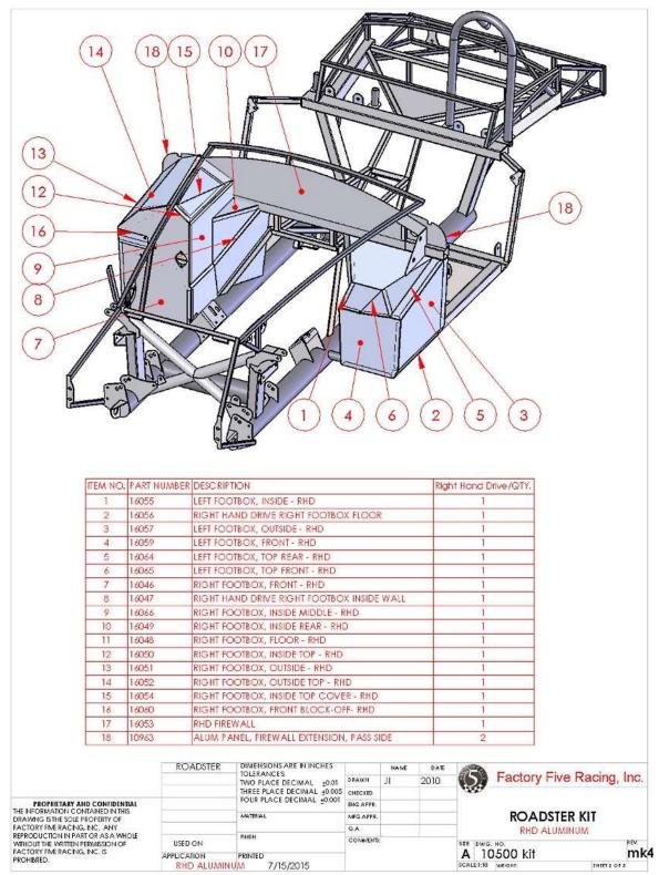
Attach the aluminum to the frame in a similar order as described in the assembly manual leaving the right footbox tops off for easy access for now.
