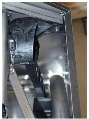
The pedal should go into the cut area of the pedal support.
