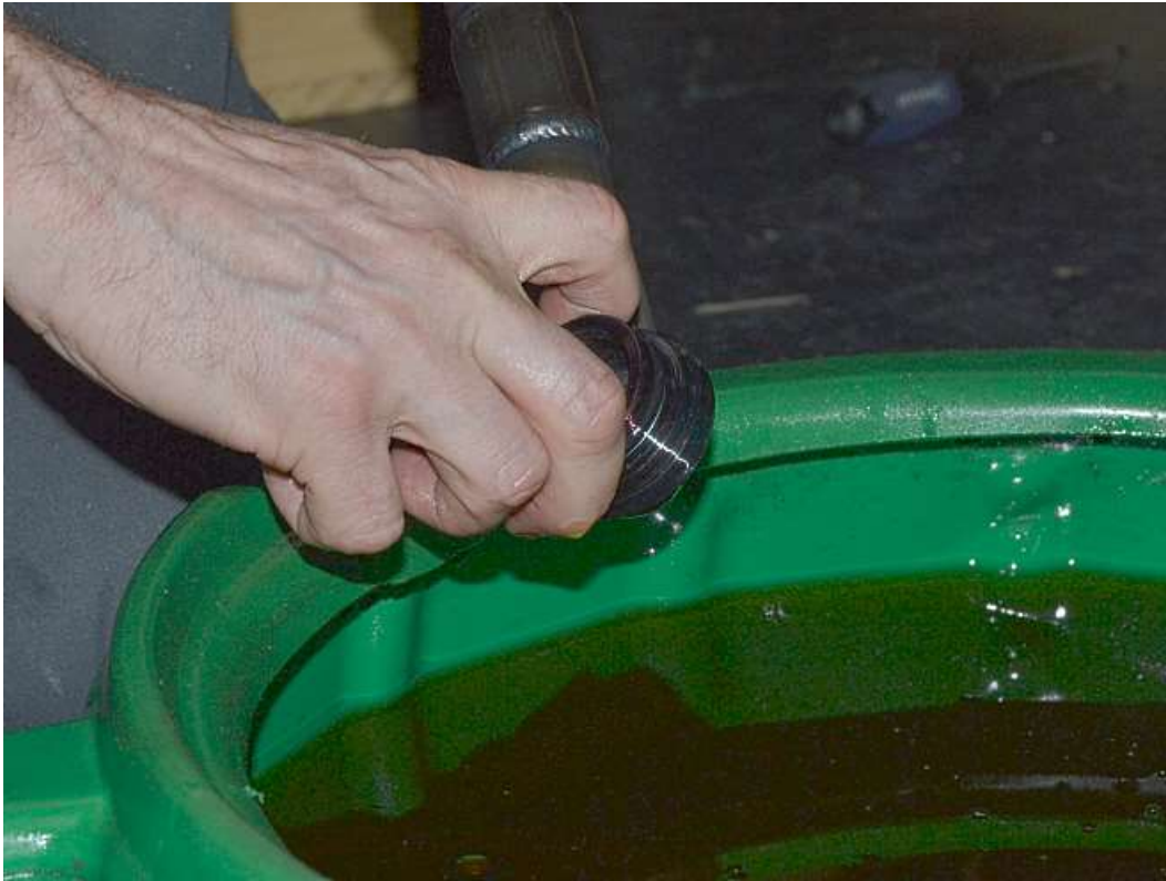
Apply some engine oil to the new pick-up O-ring.
