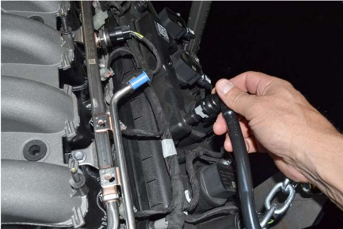
Attach the fitting to the left side valve cover.
