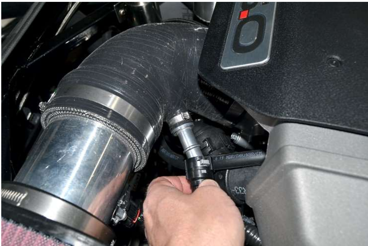
Attach the other end of hose to the intake hose CMVV Vacuum hose
