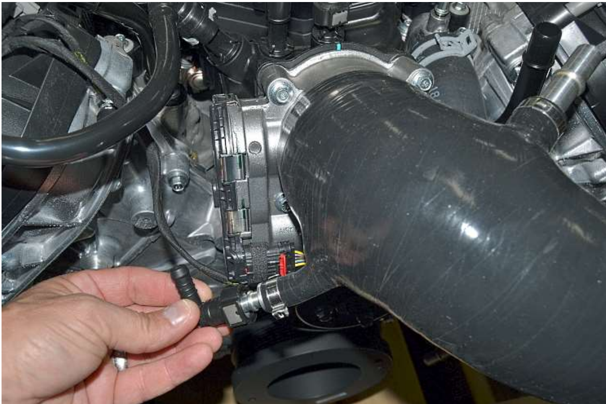
Attach a 90° 3/8" fitting to the hose connection on the bottom Silicone hose connection.
