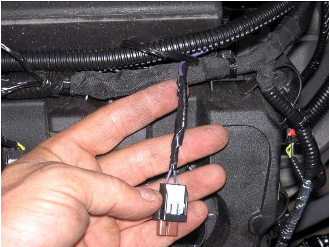
Re-wrap the coil plug wires.
