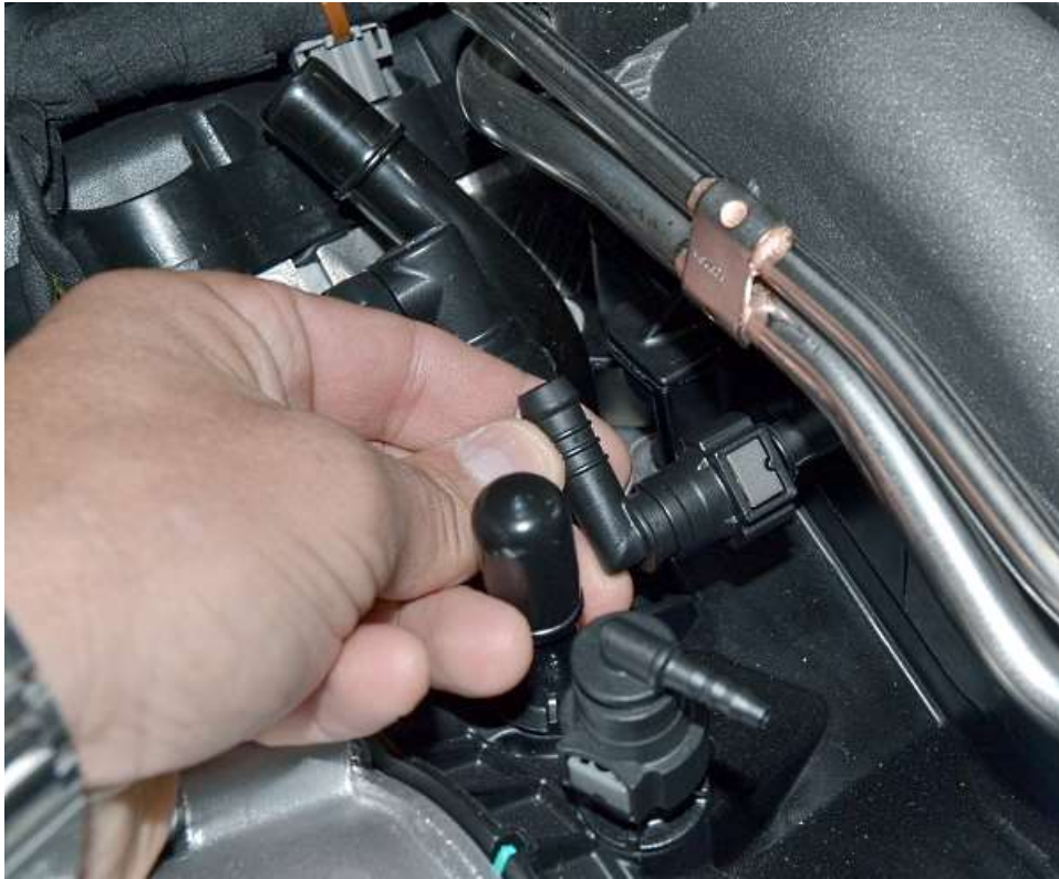
Attach a 90° 3/8" fitting to the hose connection under the intake behind the throttle body.
