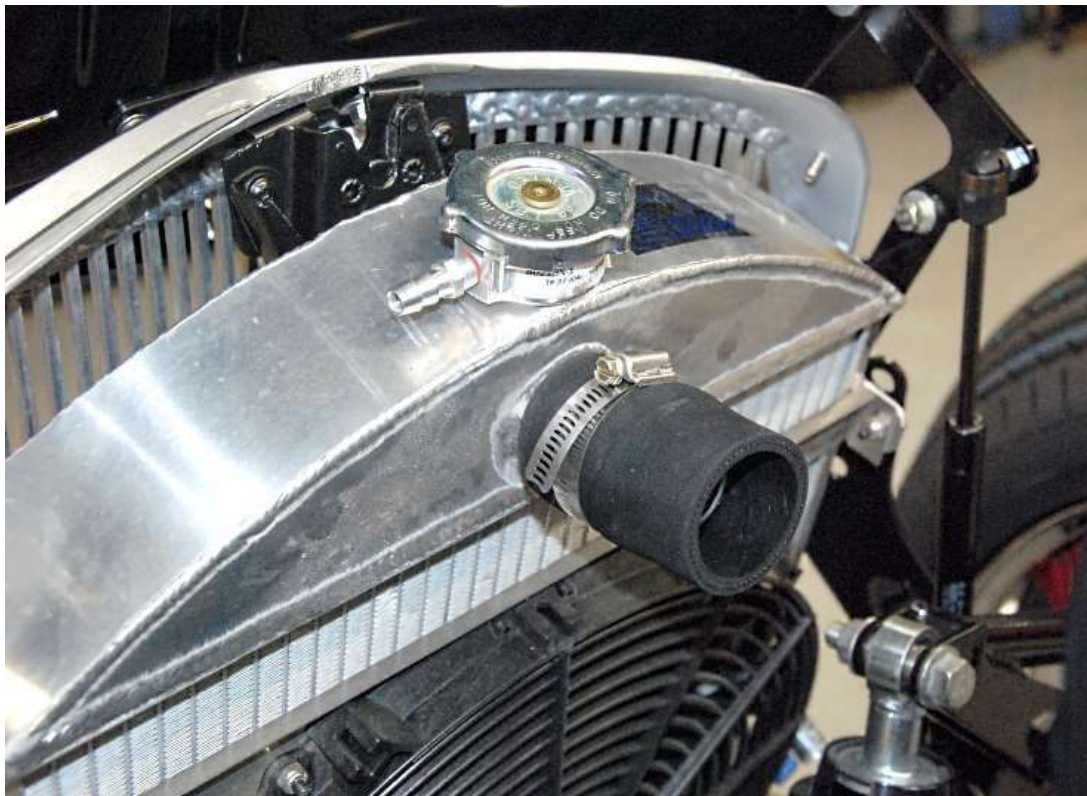
Attach another hose adapter to the radiator.
