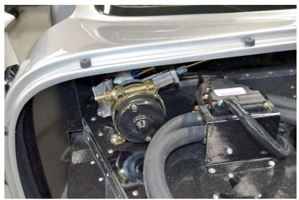
Using the wiper cable as a guide, locate the motor mounting location on the right side of the footbox so that the curve is easy or so that it is on the outside of the heater controls if being installed.
