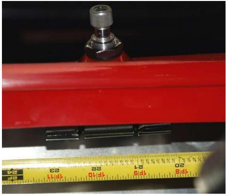
Curve the tape measure if necessary so that the tape measure is at the same angle the tubing will be compared to the wheelbox and measure to the inside of the right wheelbox. The picture shows in this cas this would be 21".
