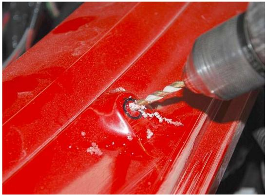
Use a <sup>3</sup>/<sub>16</sub>" drill bit to drill the center of the hole wheelbox location.
