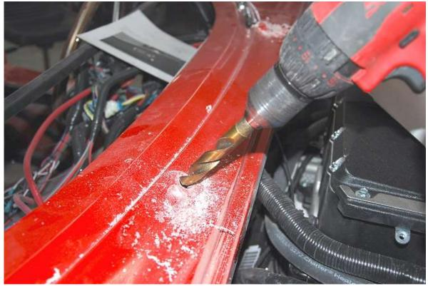
Open up the holes using a 5/8" drill bit.
