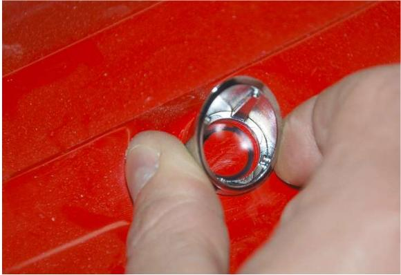
Use the chrome wiper base upside down at the molded in wiper locations and run a marker around the inside of the hole.
