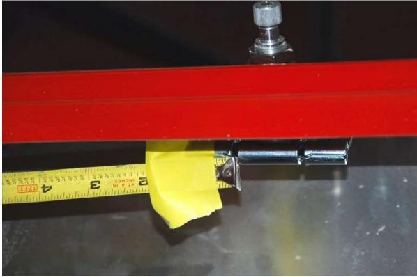
Tape one end of a tape measure to the left wheelbox inside cut area as shown.
