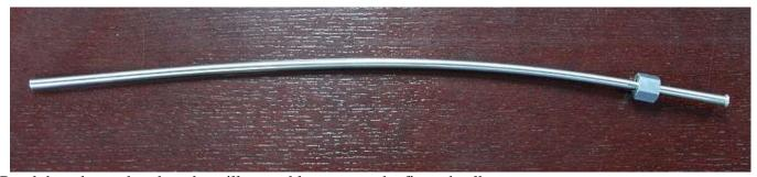
Bend the tube so that the tube will smoothly go up to the first wheelbox.
