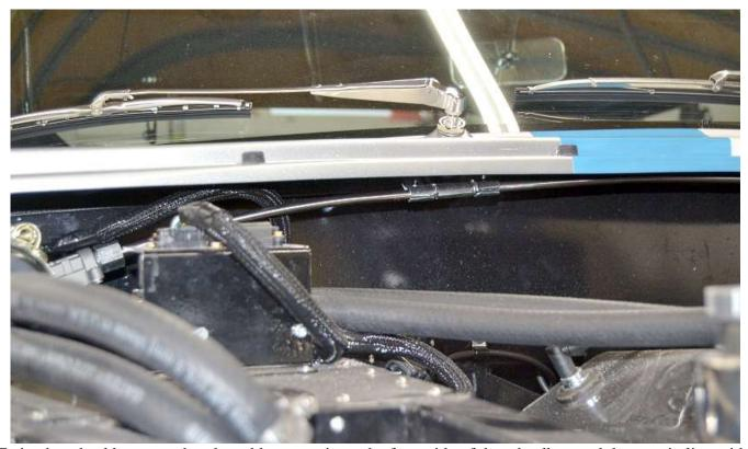
Twist the wheel boxes so that the cable mount is on the front side of the wheelbox and they are in line with each other and are pointing towards the wiper motor.
