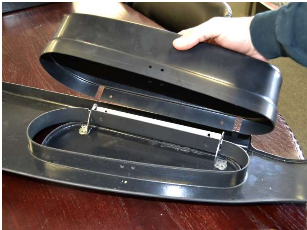
Put the glove box tub on over the flange so the hinge arms go through the slots.
