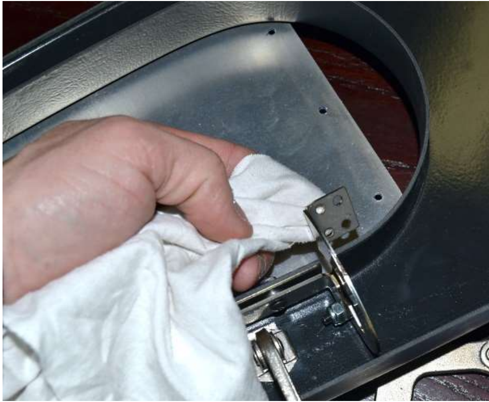
Wipe the hinge arm tabs with cleaner.
