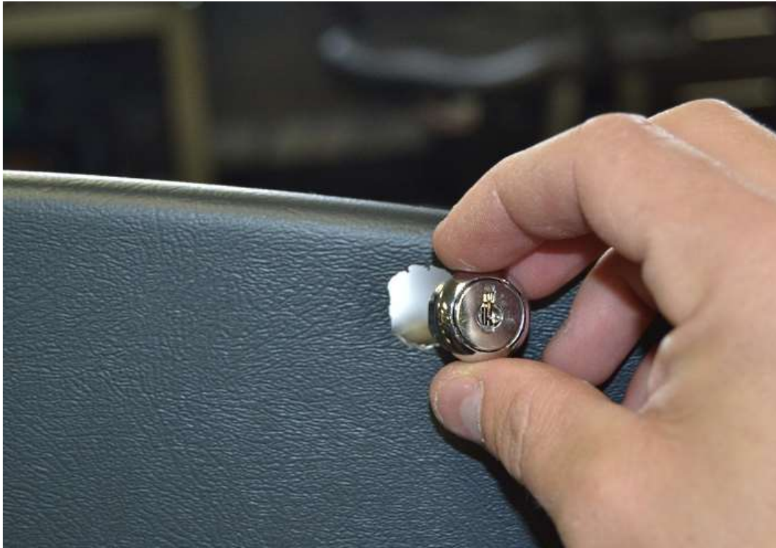
Insert the lock into the glove box door.
