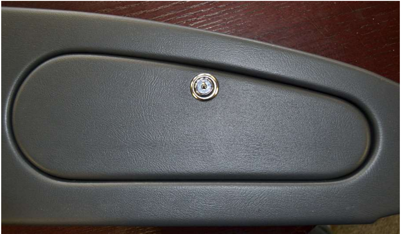
The glove box lock can be used with or without the trim ring as desired.
