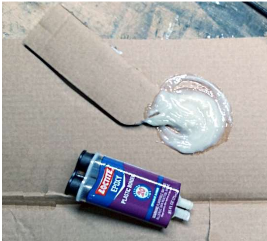
Mix up a small amount of 5 minute epoxy as directed.
