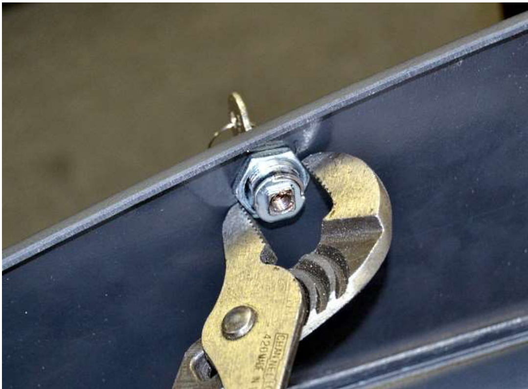
Tighten the nut on the backside using a pair of channel lock pliers.
