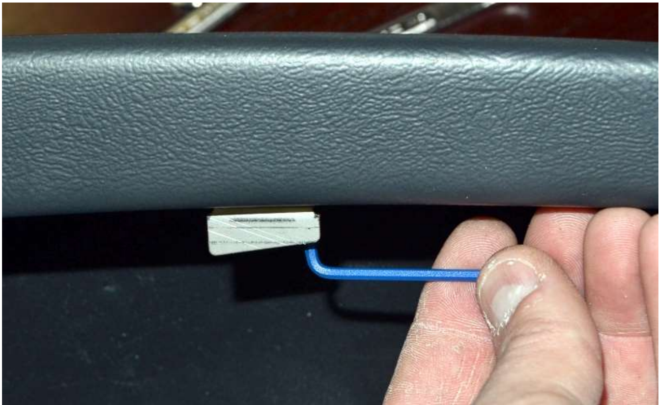
If the door does not sit flush with the dash at the top, loosen and adjust the lock tab.
