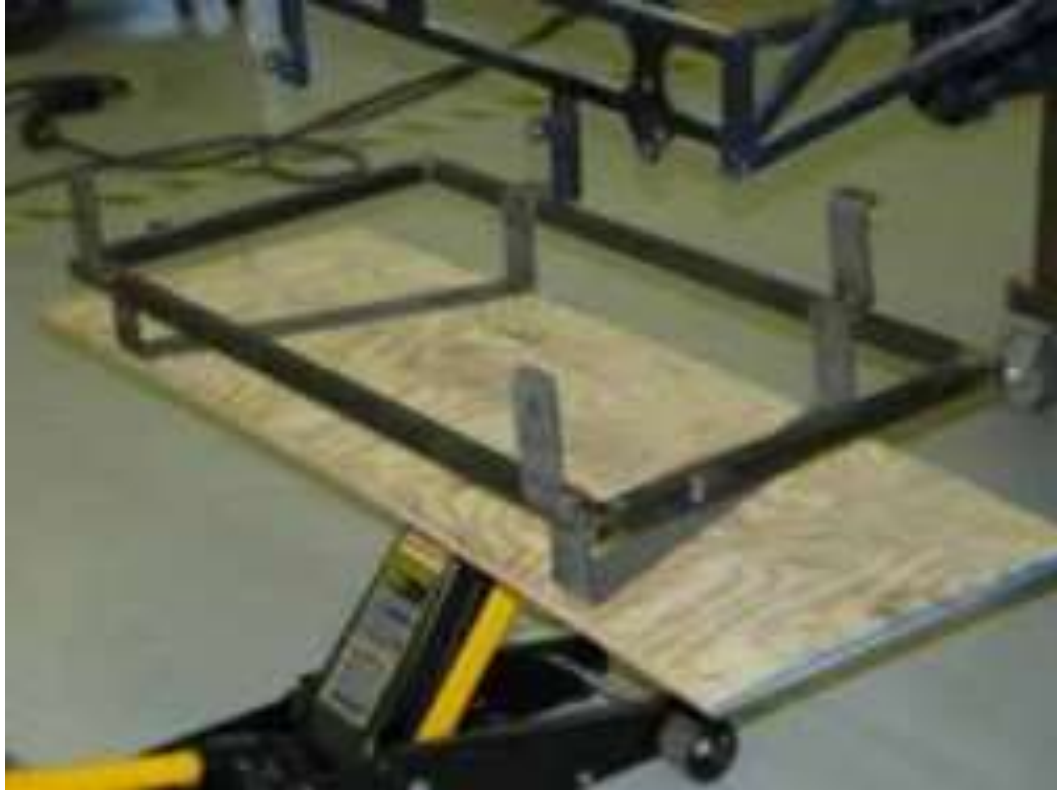
Trial fitting of the cage without cell in place.
