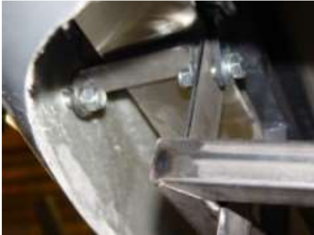
Lower Body/Cage Mount Bracket Installation showing Body Bolt and Upper Cage/Frame Bolt. Lower Cage Bolt not Visible.
