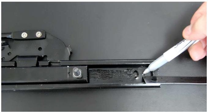
Use a <sup>3</sup>/<sub>16</sub>" drill bit at the point marked on the tracks then open this up with a <sup>5</sup>/<sub>16</sub>" drill bit.
