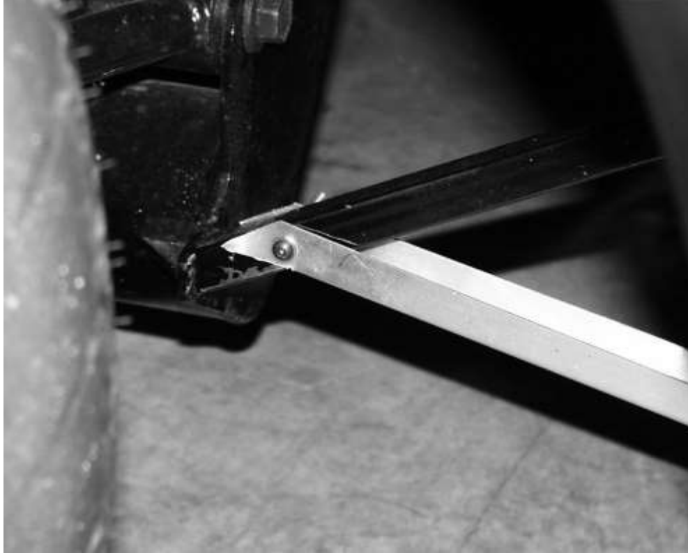
Support brace attached to lower front body mount support
