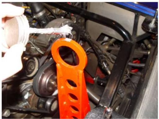
Once you have a height you want, clamp or tape the hook in position and put a dab of grease or anti-seize on the top.
