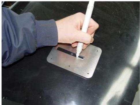
Drill a small hole through the hood at the center of the marked spot and then use the trim plate as a template to mark where you will cut. It is always best to start tight with the hole in case any adjustments are needed.
