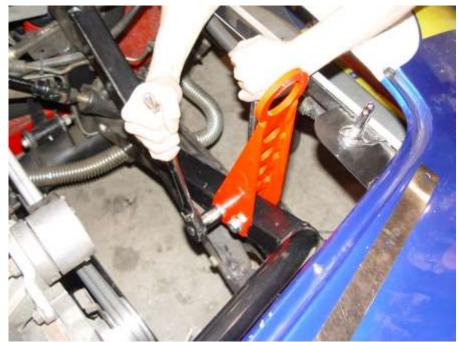
Bolt the hook in place using the two <sup>1</sup>/<sub>2</sub> inch bolts and lock nuts.
