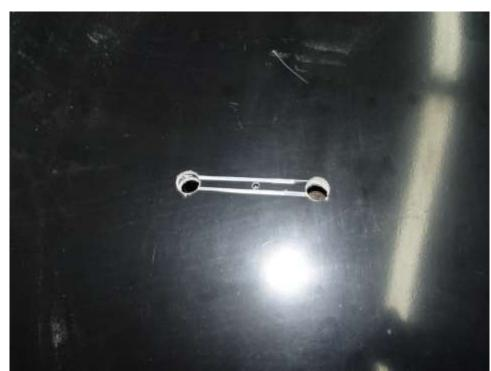
Drill out both ends of the slot with a  $\frac{1}{2}$ " drill and connect the two holes with your saw.
