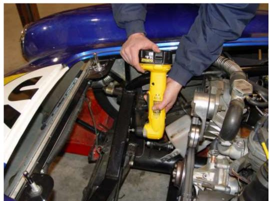
Remove the hook and drill the two holes. It is easier to do this if you start with small bits and work your way up. Be very careful to keep the drill straight so the bolts will fit through both sides.
