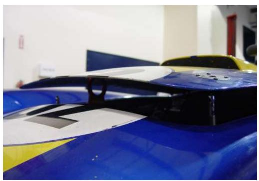
Gently set the hood down in place allowing the grease to mark the spot where you will need to cut the slot and then remove.
