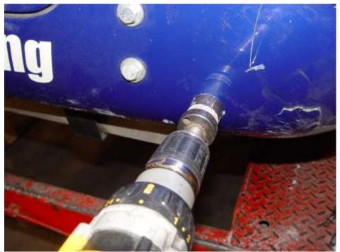
Drill a small pilot hole for the tow eye through the body and frame member. If you are centered on the tube where you would like to be use the hole saw to cut out the body centering on the pilot hole.
