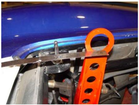
Using a flexible ruler or small sheet of poster board or other flexible material you can simulate the arc in the hood and determine the mounting height for the hook.
