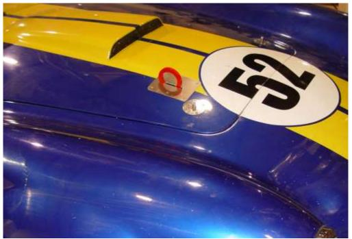
Set the hood back into position and fit the trim plate. It is set up for 1/8" rivets but can be screwed down to match the hood pin plates as well.
