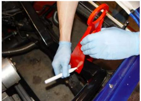
Once the hook is lined up with the slot and is at a height where it is easy to attach a hook to with the hood in place, remove the hood and mark the frame for mounting.
