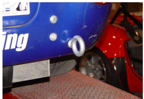
Slip the trim plate (if desired) on the tow eye and install it using the spacers to bring it out past the body where a hook or strap can get to it, once in position tighten it using a pry bar through the eye and a little thread locker on the nut.
