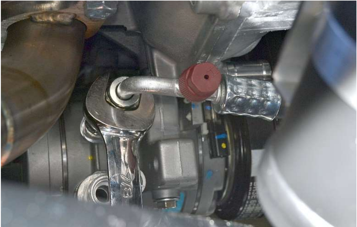
Oil the o-ring and reinstall the compressor fitting tightening the fitting using a \frac{7}{8} " wrench.
