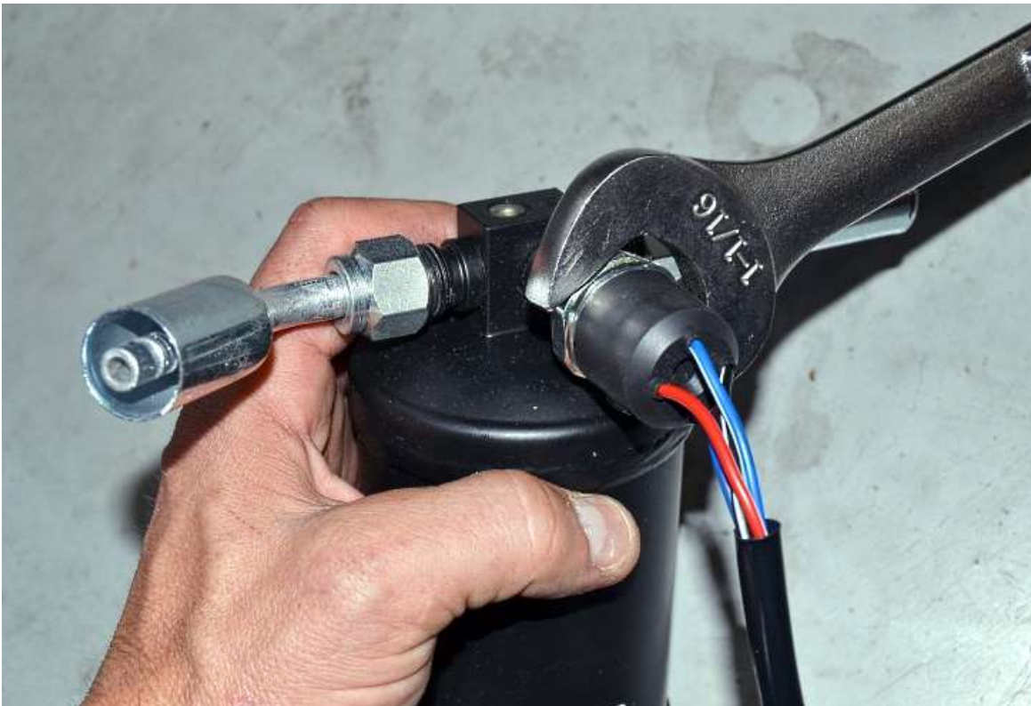
Use a 1 1 / 16 " wrench to tighten the trinary switch onto the Drier.
