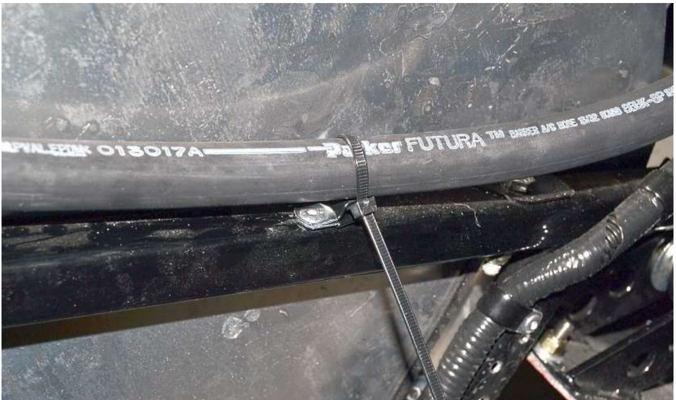
Fasten the hose to the nose support tubes using a small insulated clip, \frac{3}{16} " rivet and a zip tie from the kit.
