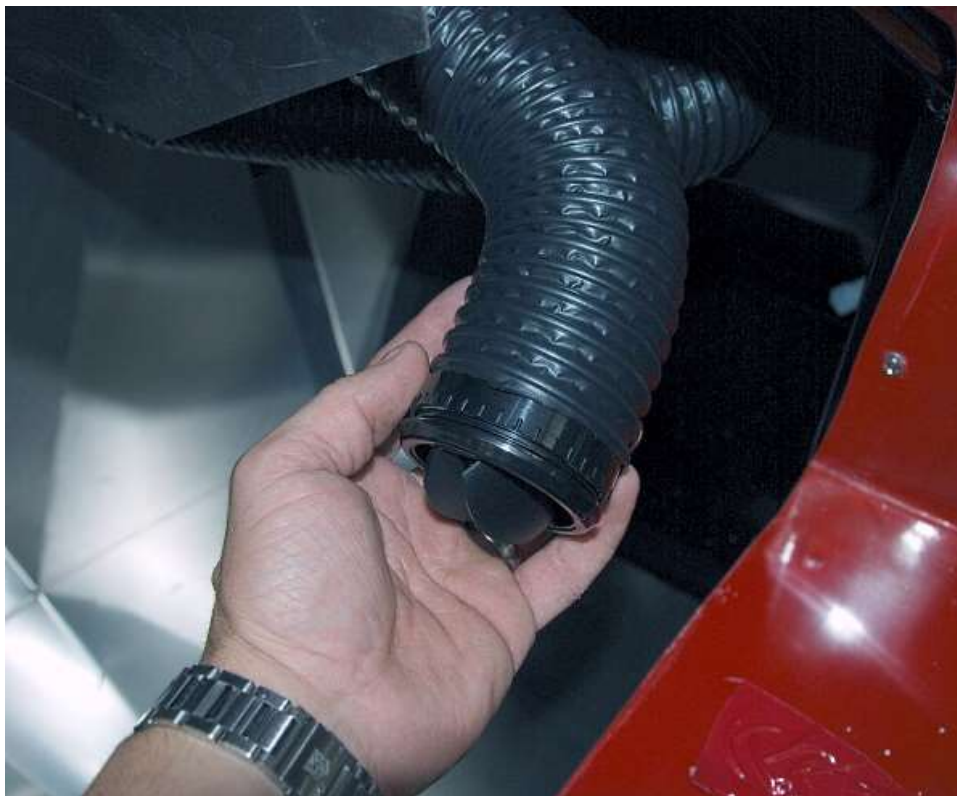
Cut the hose and put a dash vent in the end.
