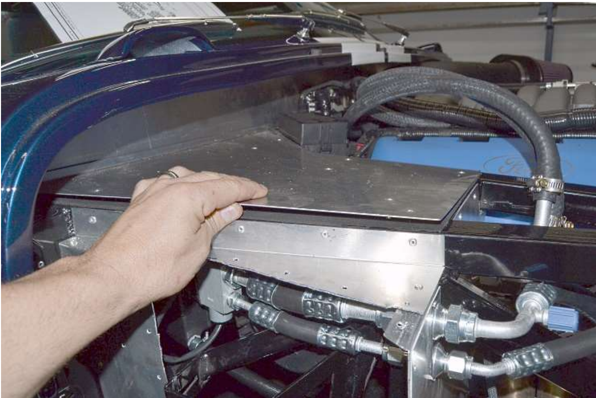
Position the footbox top back on the frame using a couple screws or rivets to hold it in place.
