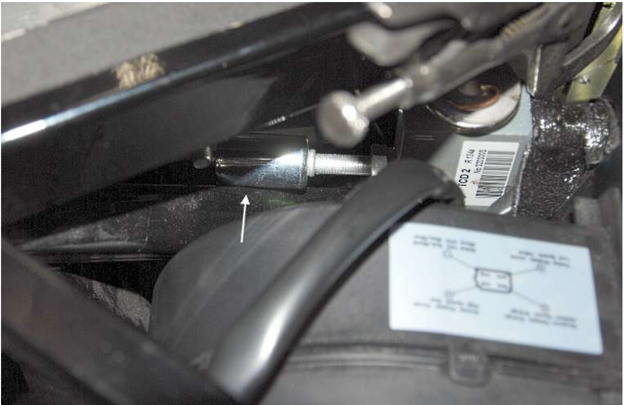
the A/C lower #6 hose fitting clears the frame tubes;
