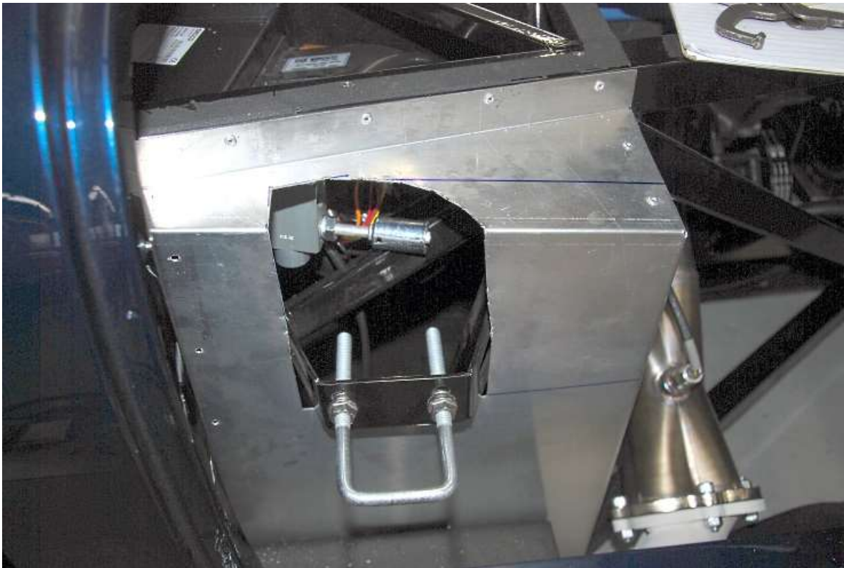
Cut the piece off to give easier access for the tin snips.
