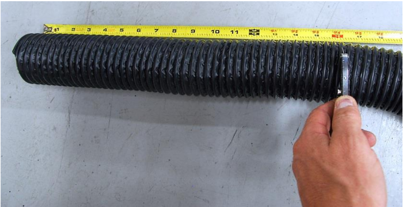
Cut a 16" piece of the 2.50" air hose with a razor knife.
