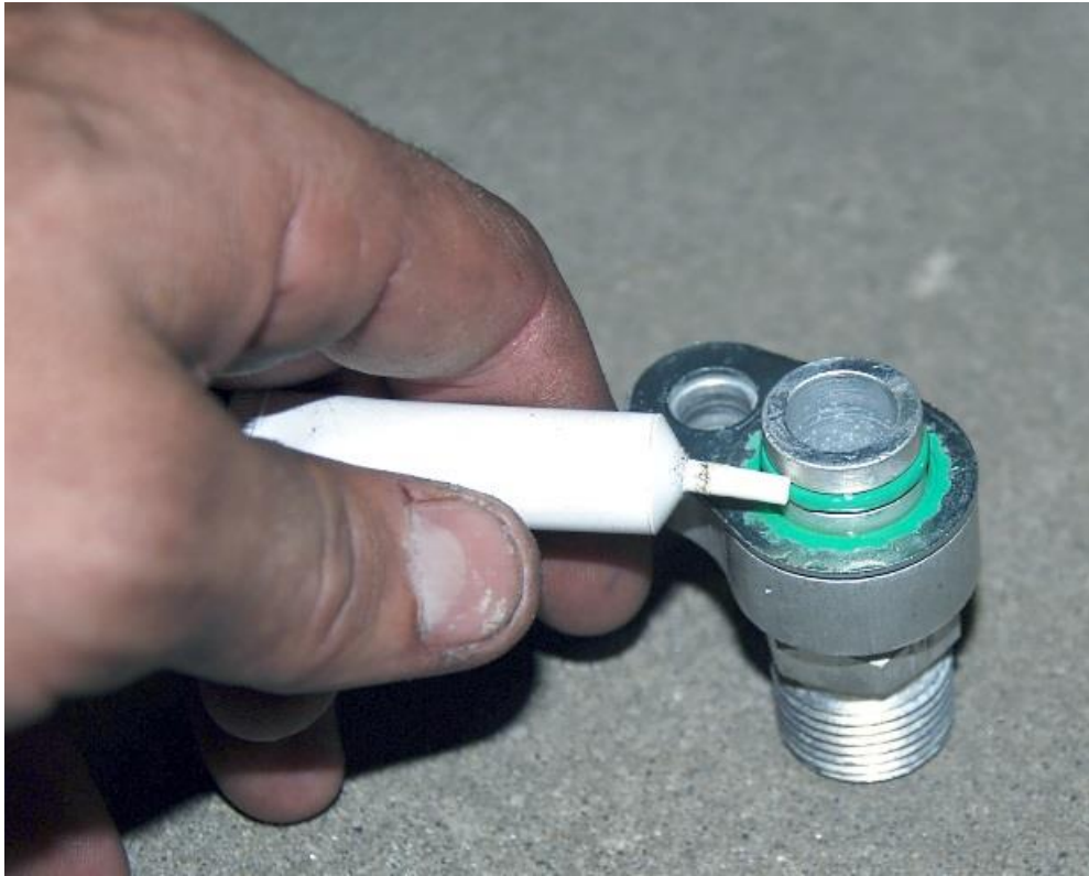
Lubricate the green O-ring and surface of the adapter blocks.
