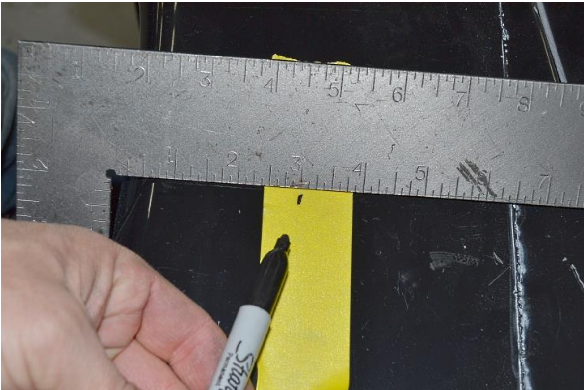
On a hot rod, in front of the driver and passenger measure from the edge of the dash towards the windshield location 3" and put a dot on the top of the dash. On the truck this measurement should be 5.50".
