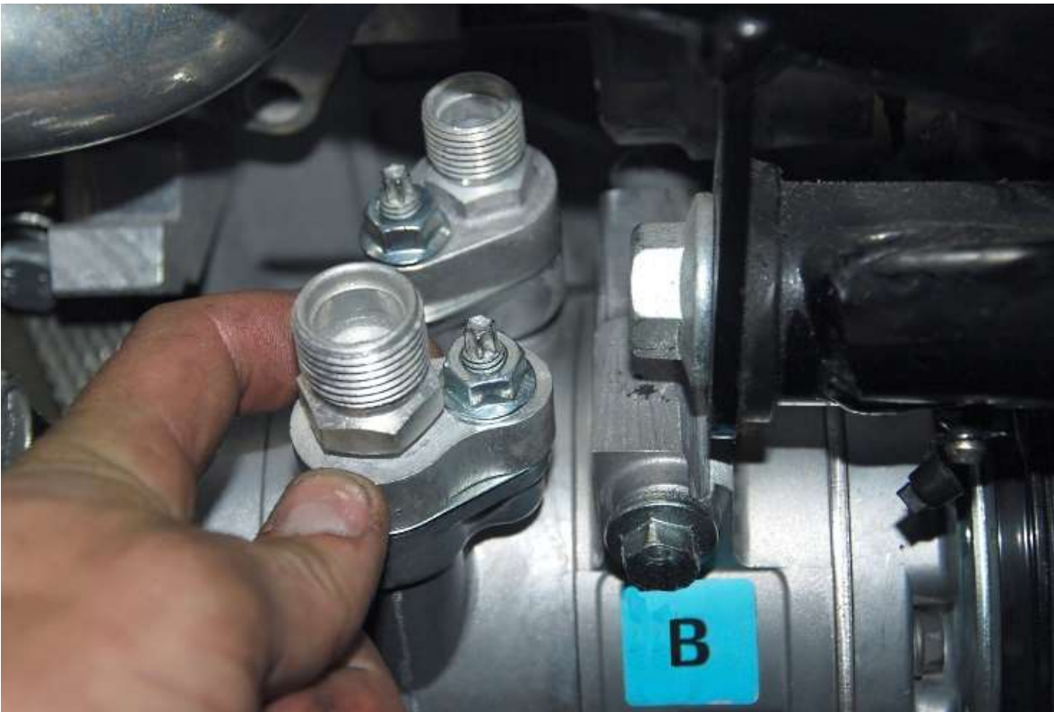
Use a 13mm socket and ratchet to tighten the blocks to the compressor.
