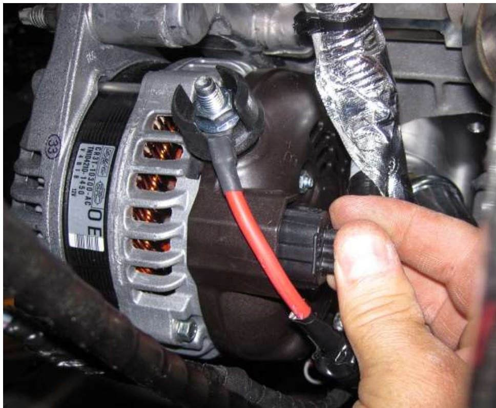
Attach the engine harness alternator plug to the alternator.
