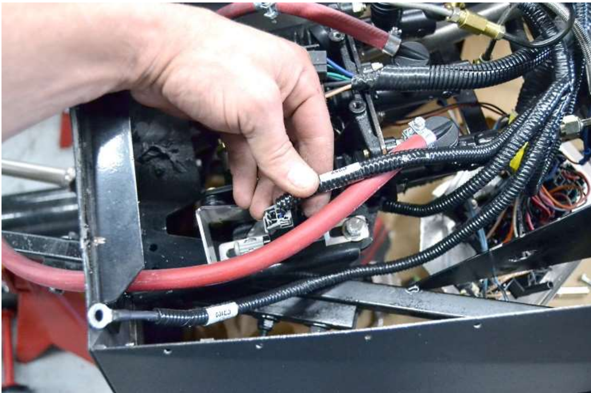
Connect the clutch pedal travel switch lead to the switch.
