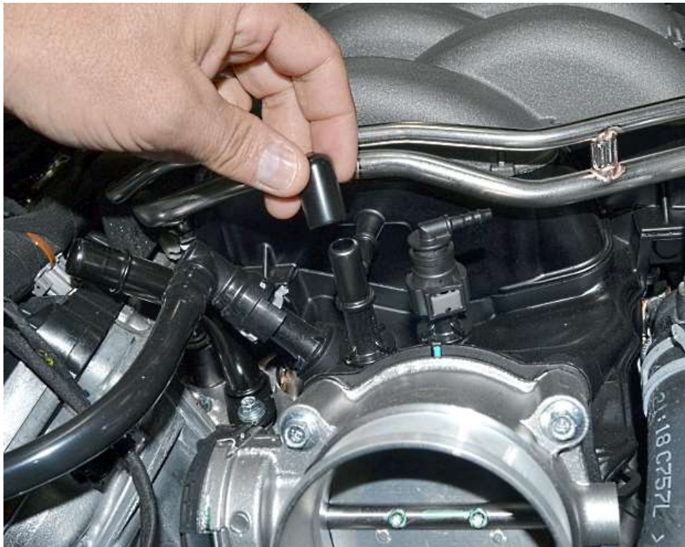
Block off the \frac{1}{2} " large vacuum port just behind the throttle body.
