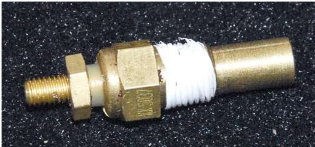
Screw the adapter into the larger adapter on the block.
