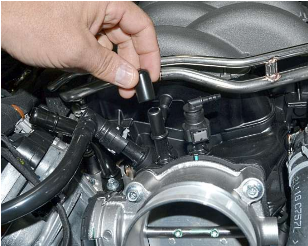
Block off the large vacuum port just behind the throttle body.
