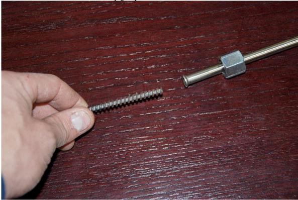
Insert the wiper drive cable into the tube with the ferrule on from the flared tube end and slide the tube down to the motor and attach the nut to the motor.
