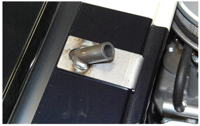
With the hood open, use the diagram above to locate the wiper drilling tool on the cowl from the hood lip and the inside of the windshield mount holes, the tool will go over the body hood lip.
