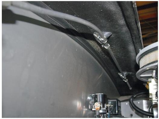
Twist the wheel boxes so that the cable mount is on the front side of the wheelbox and they are in line with each other and are pointing towards the wiper motor.
