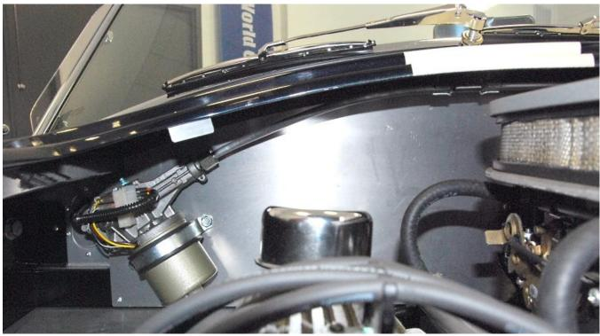
Using the wiper cable as a guide, locate the motor mounting location on the right side of the firewall so that the curve is easy or so that it is on the outside of the heater if being installed.
