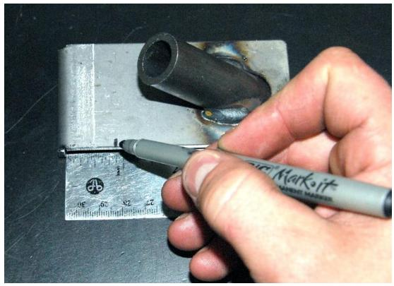
Mark the wiper tool 1/8" from the inside of the bend
