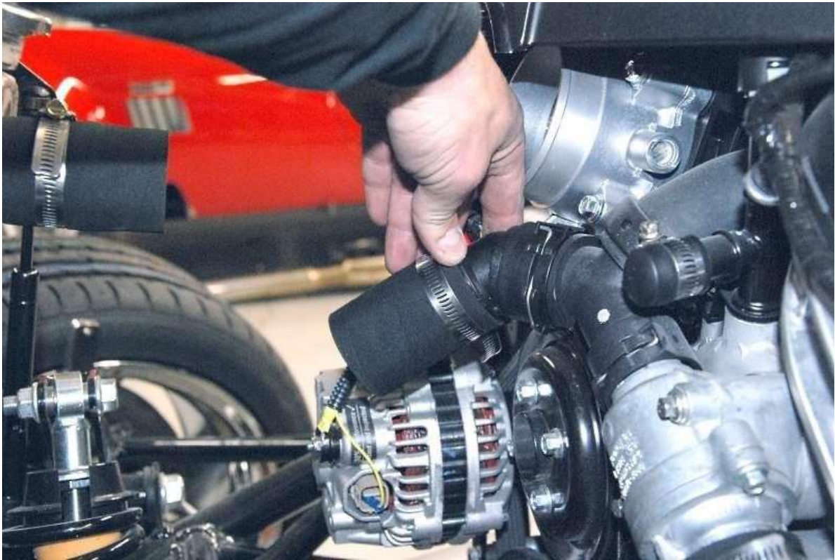
Push the adapter onto the engine.
