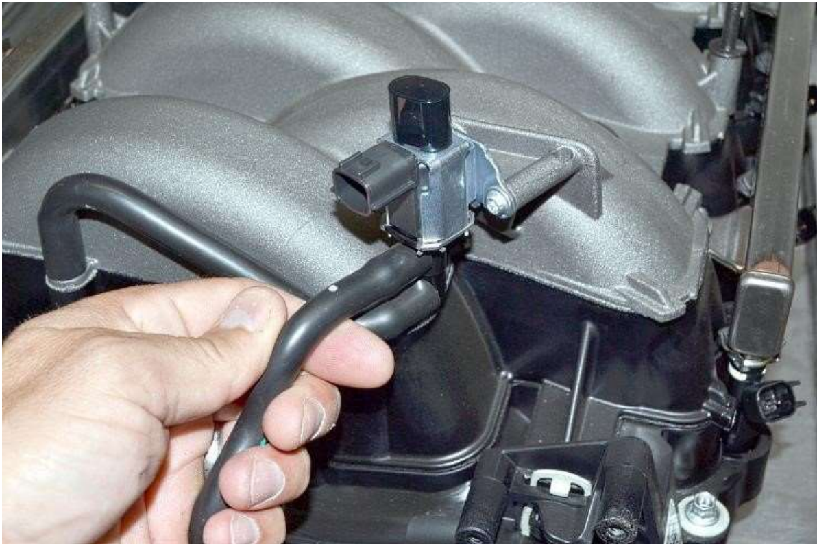
Remove the vacuum line going to the CMCV from the solenoid on the intake.
