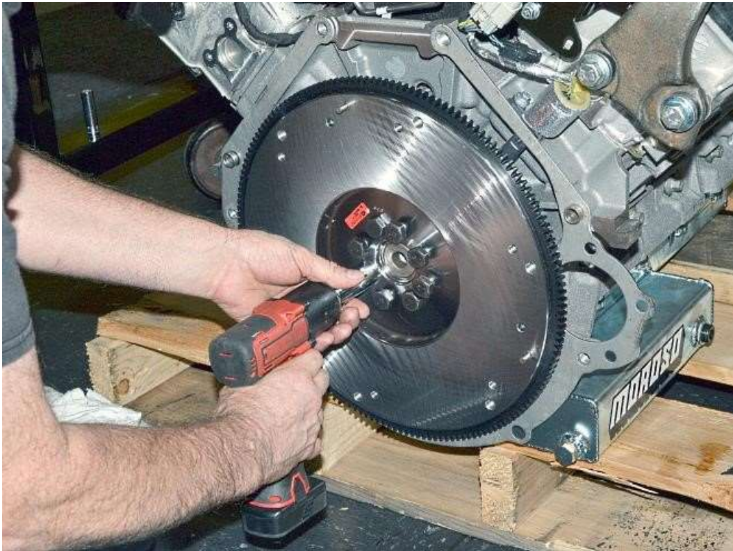
Attach the flywheel to the engine with a 19mm socket.
