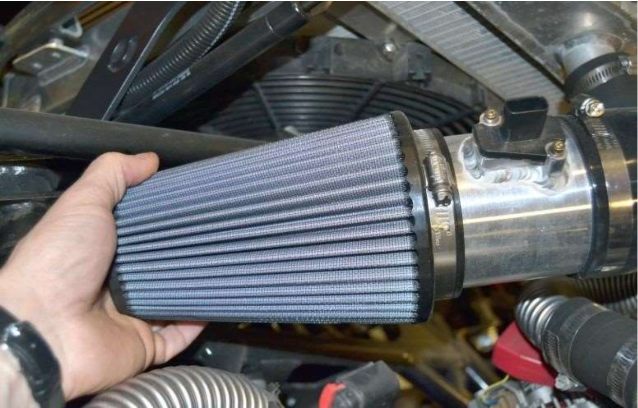
Push the FFR filter onto the Mass Air meter making sure that the meter is facing the correct direction. Slide hose clamps onto the 90° Silicone hose.
