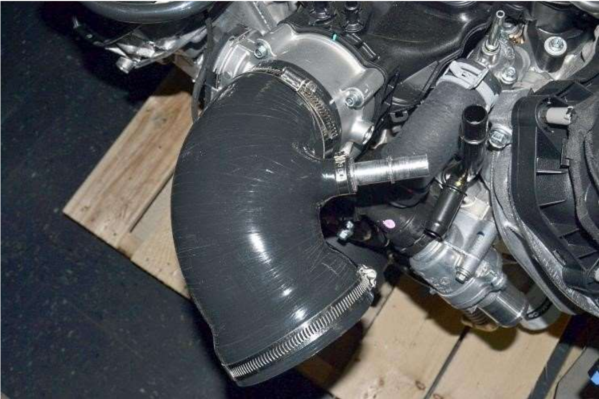
Push the small end of the silicone hose onto the throttle body.
