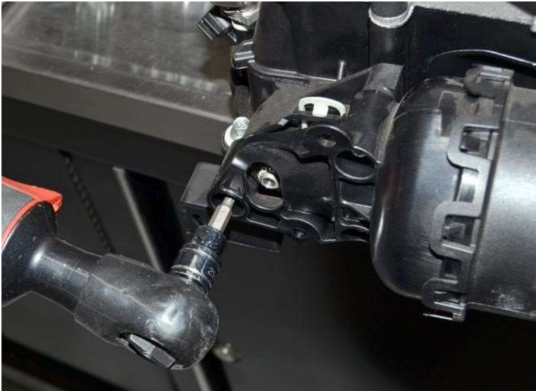
Remove the screws using a T-25 Torx bit.
