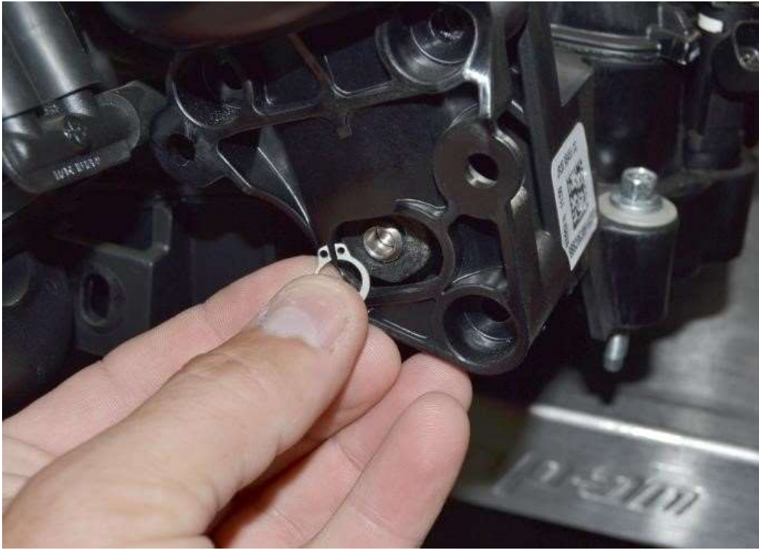
Remove the snap ring holding the CMCV to the intake shaft.
