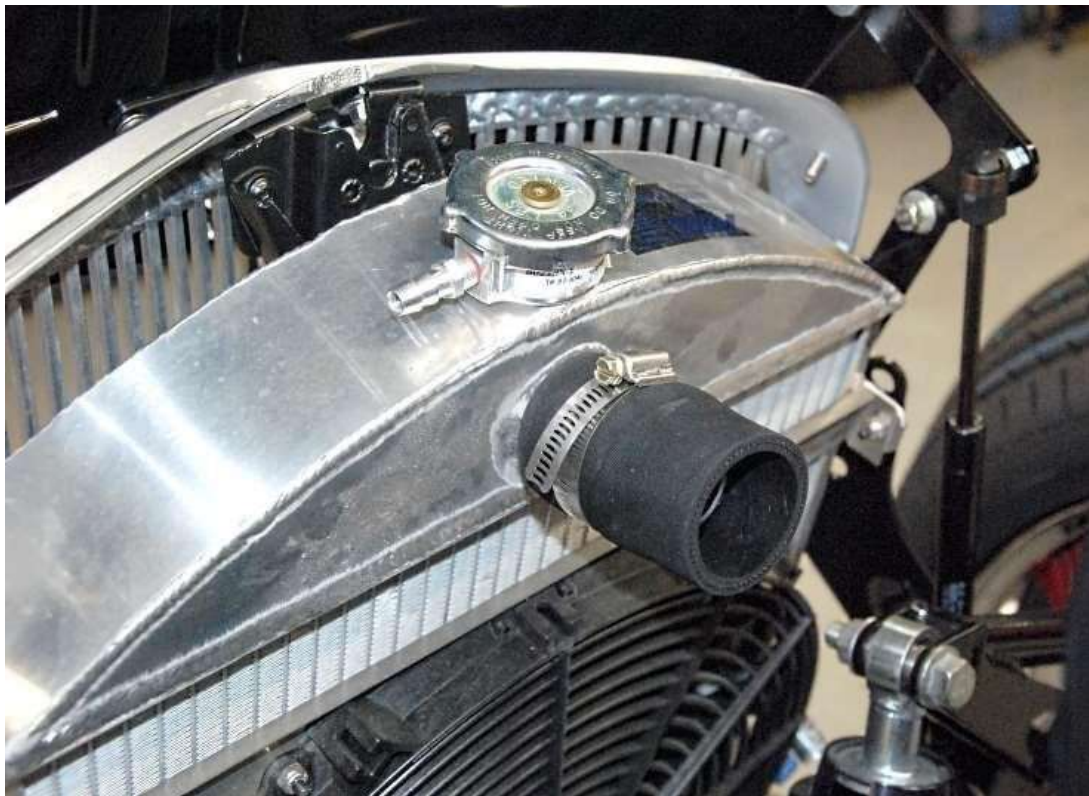
Attach another hose adapter to the radiator.
