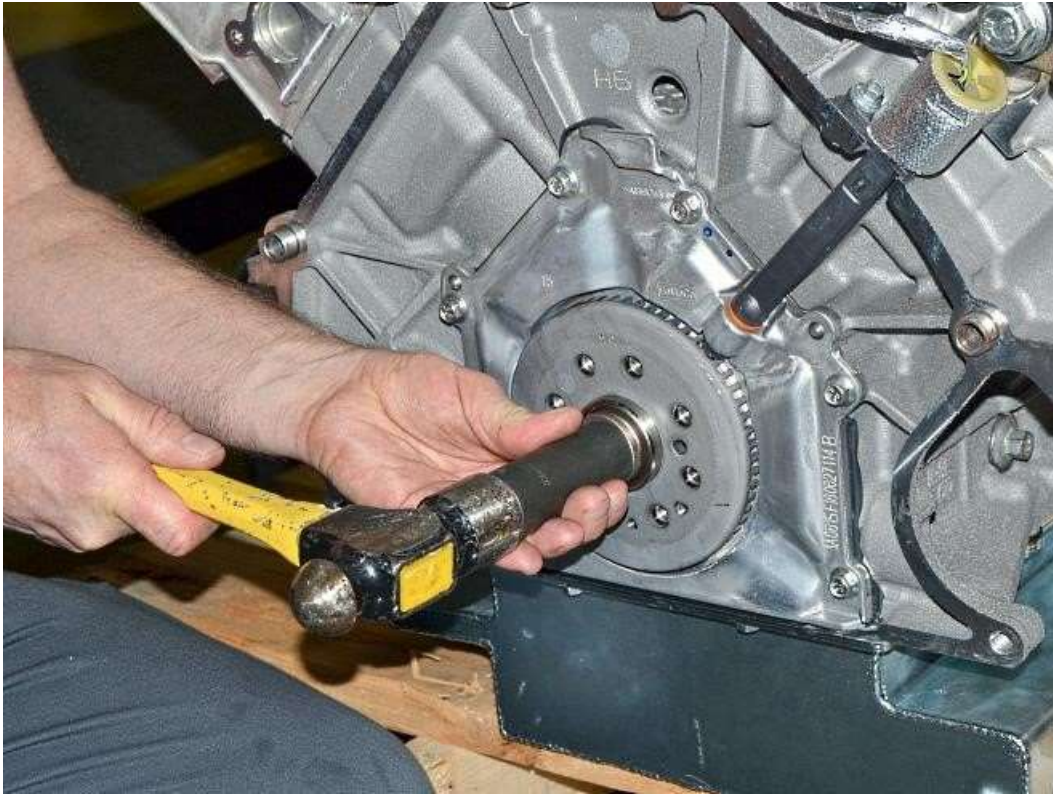
Use a hammer and 7/8" or 22mm socket to hit the thrust bearing into the back side of the crank.
