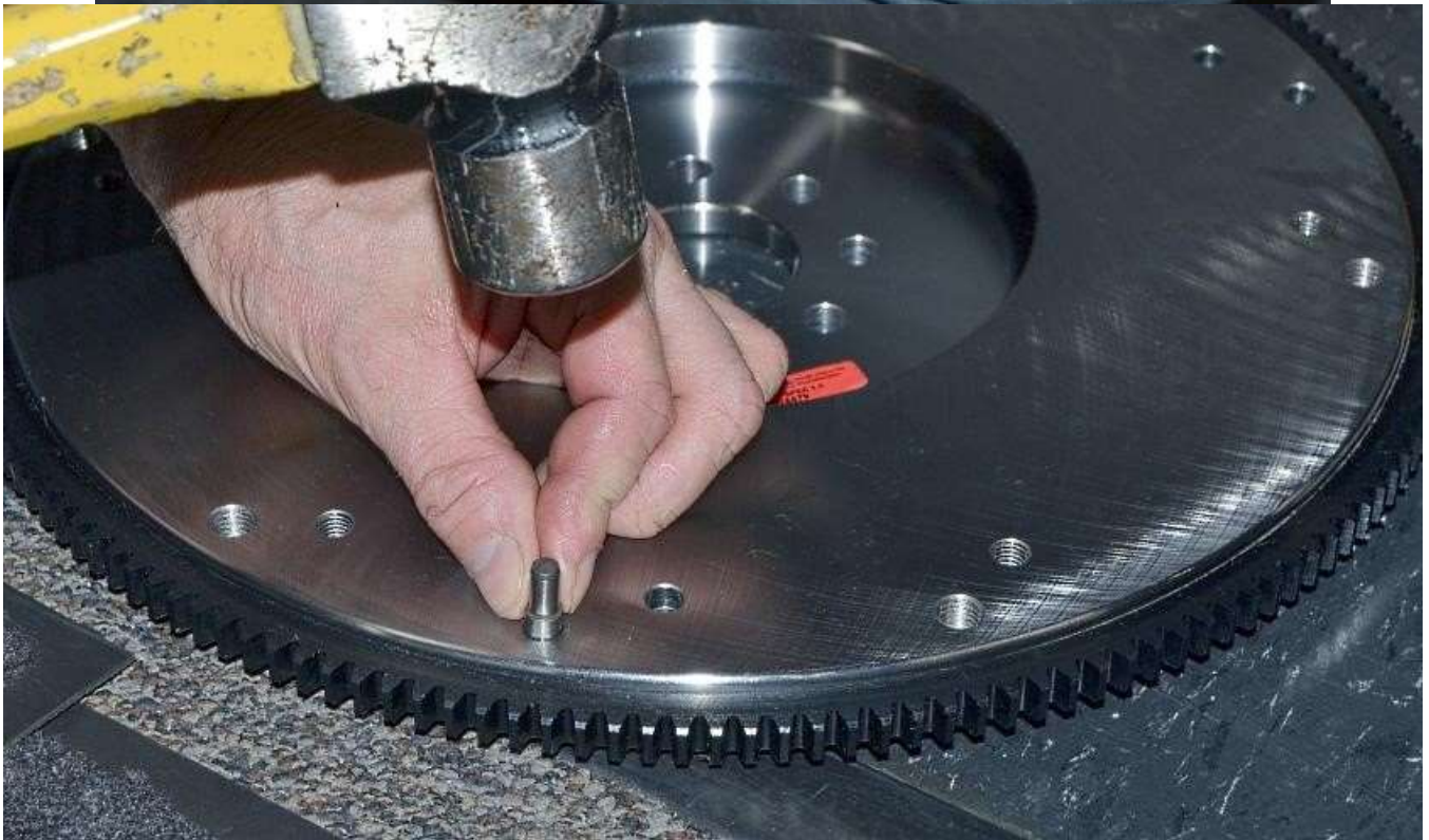
Use a hammer to hit the clutch pins into the new flywheel.
