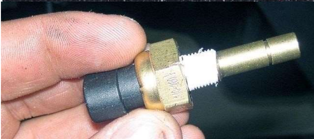
Put Teflon tape on the sending unit Autometer top, Vintage bottom
