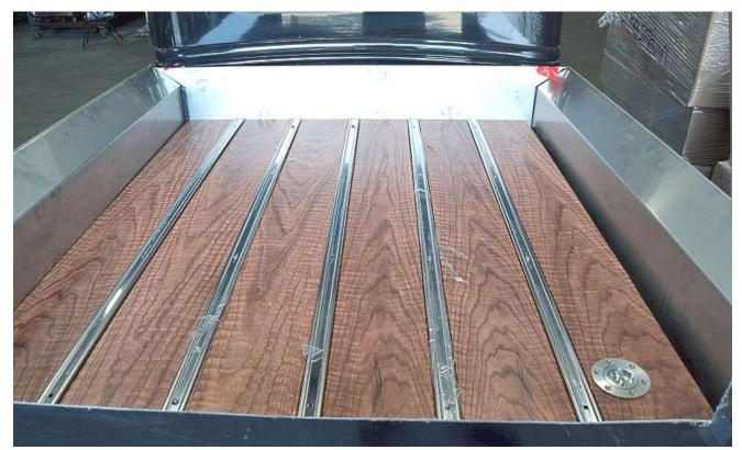
Install the remainder of the Floor Boards with the filler/rounded edge board on the right side. Do not attach the filler neck to the cap yet.
