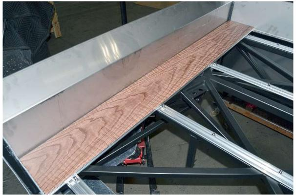
Starting on the left side, lay the rounded edge board on the Floor supports making sure there are no T-Nuts underneath and against the bed side.
