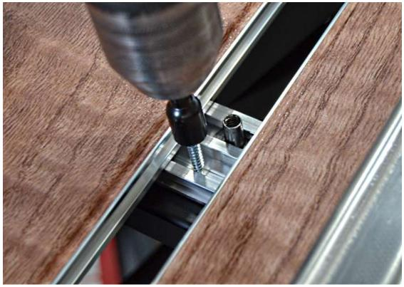
Remove the center Bed strip then use a drill with  $\frac{5}{16}$  nut driver to screw the #10 self drilling screws through the other slot in the Support bracket into the frame tube.
