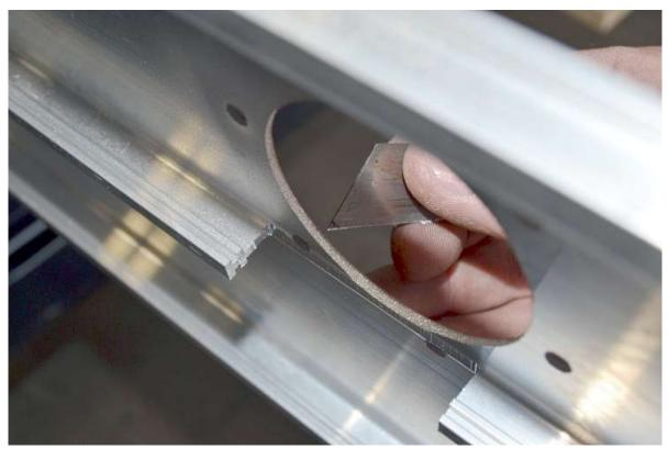
Looking through the hole in the floor board from the back side, use a razor to put a slice into each of the holes.
