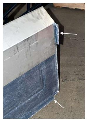
At the front of the side panel, it may be necessary to trim the upper flange and lower cut corner more so that the panel becomes tight with the bed front.
