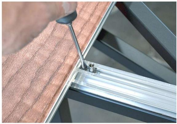
Slide the last T-nut about  $\frac{3}{4}$ " over from the edge of the board.
