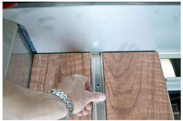
Lay another board down and use a Bed Strip to space it so the Bed Strip will fit into the edge grooves.
