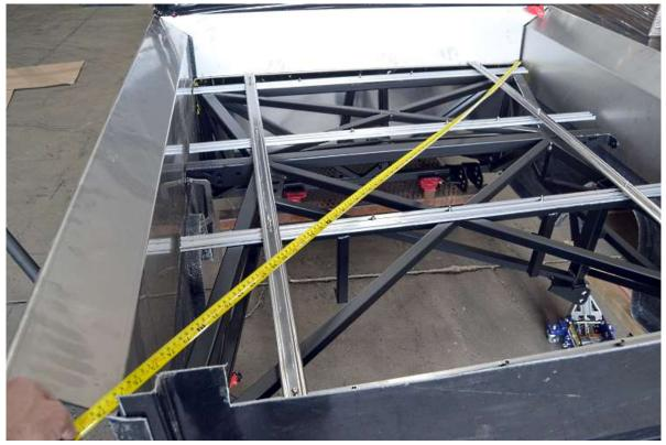
Use a tape measure diagonally between the corners to square up the bed.
