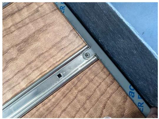
Place the rear board cover on top of the Bed Strip and behind the bed rear panel and attach loosely with short Button head screws.
