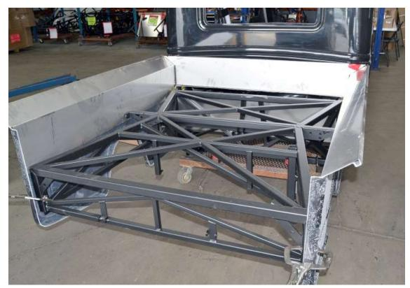
Place the bed front on the frame behind the cab and clamp the bed sides to the frame.
