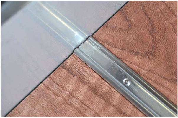
At the front of the bed make sure that the bed strips are even with the edge of the boards.
