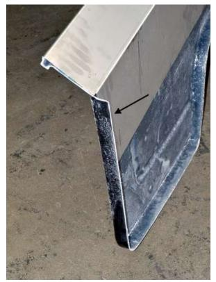
At the rear of the side panel, it may be necessary to trim the flange location shown as well as the corresponding flange on the rear panel to get the correct width.
