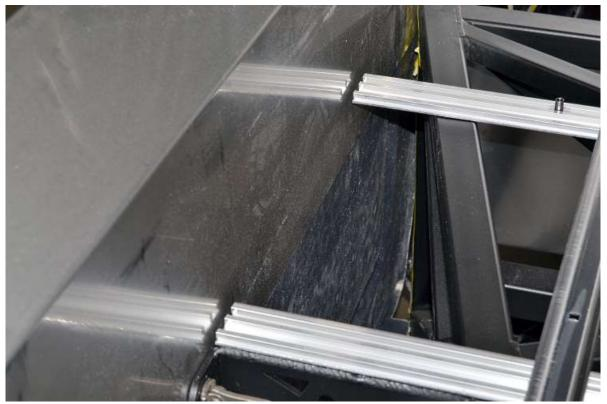
The Under Floor Supports should touch or be very close to the bed sides. If not these can be adjusted later after the bed dry fit. For now, butt the Supports against the left side.
