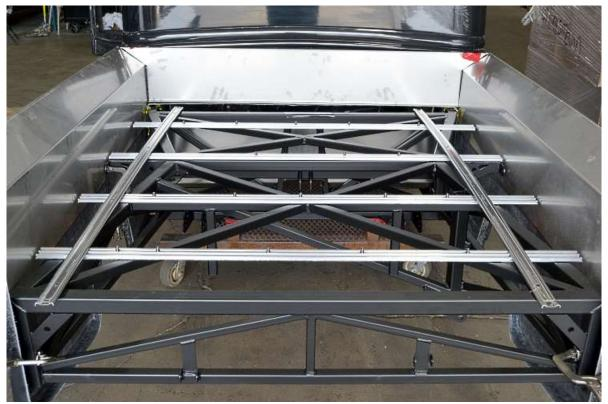
Lay the five Under Floor Supports across the frame and lay two of the Bed Strips front to back on the frame to get the location of the supports.
