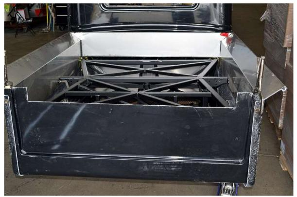
Clamp the rear panel on the inside of the side panels so that the back panel touches the back of the frame. This will also set the front to back location of the bed.
