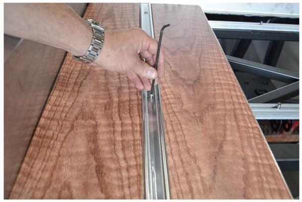
Thread the long button head screws into T-nuts a few turns.
