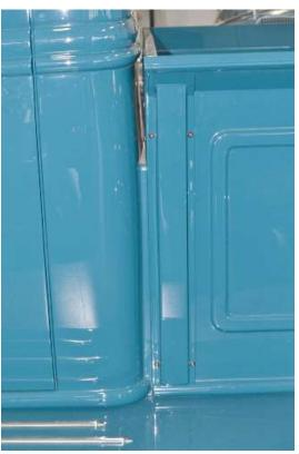
$^{\circ}$  The truck bed will end up roughly 0.50" behind the cab with an even gap.
